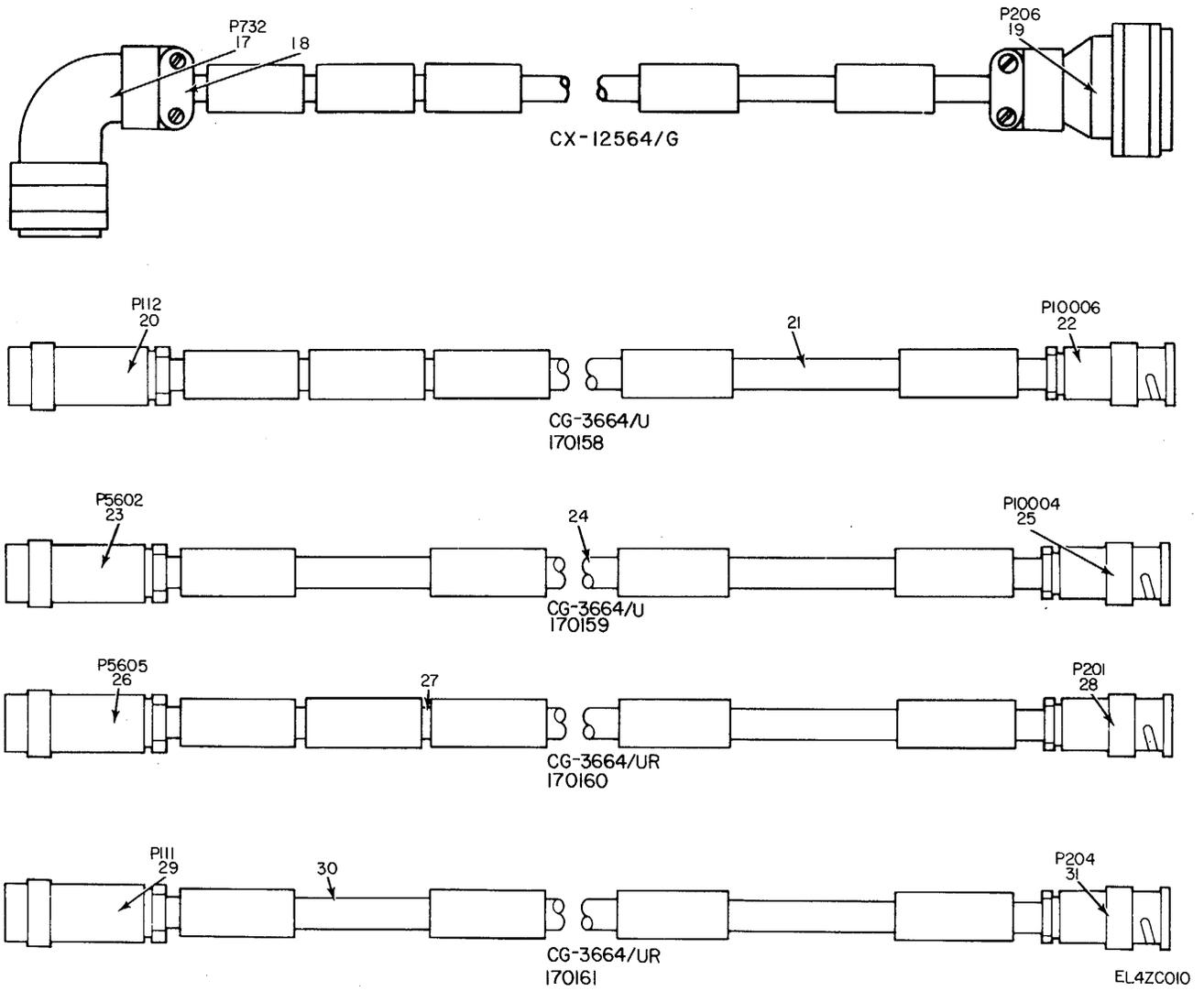
Figure 6. Cable Assemblies, RF and Power (Sheet 2 of 2).
