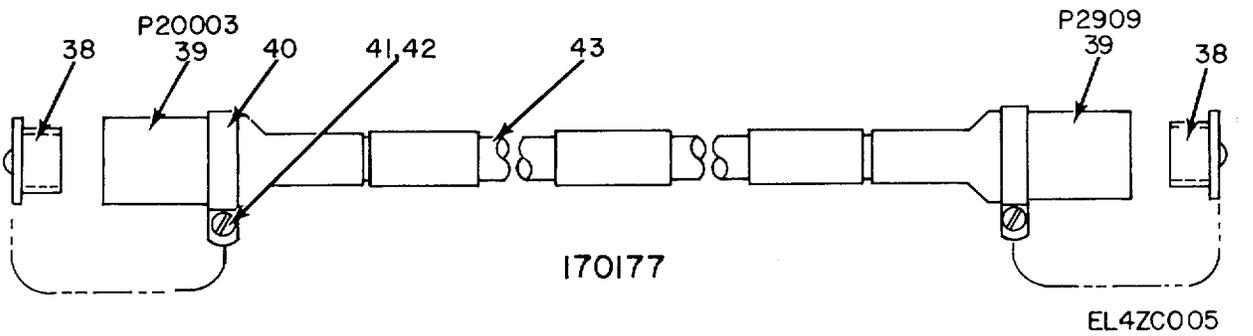
Figure 3. Cable Assemblies, RF and Power (Sheet 2 of 3).
