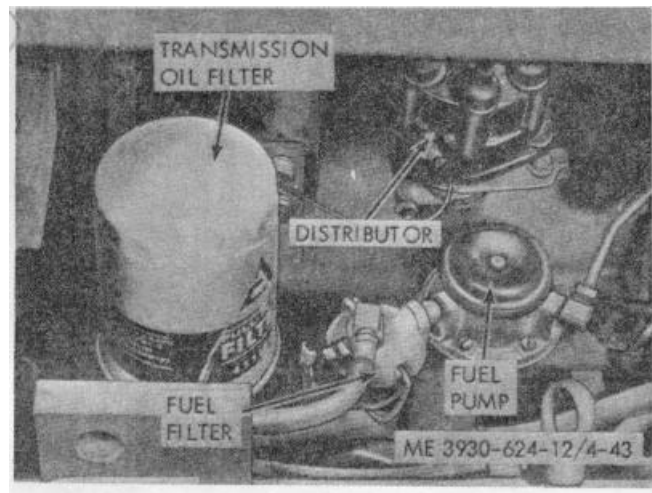
Figure 4-43. Transmission oil filter element.
