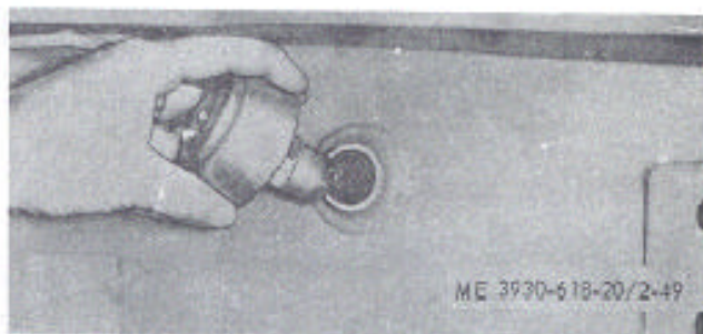
Figure 2-49. Removing hydraulic oil tank breather.
