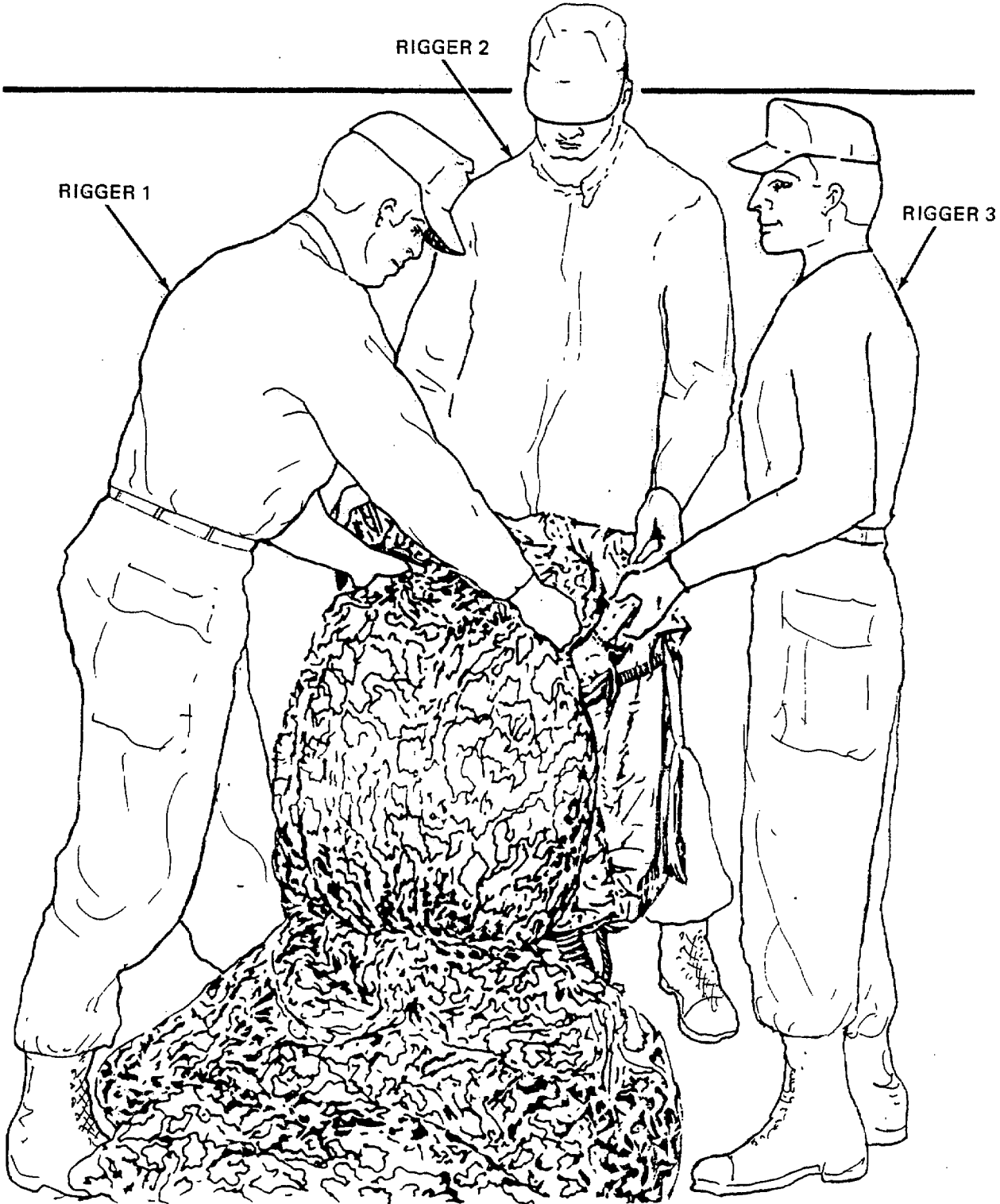
Figure 2-79. Stowing the Canopy Into the Deployment Bag .
