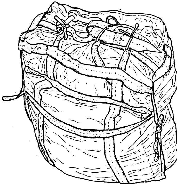
Figure 2-43. Packing Completed, G-12D Parachute.
