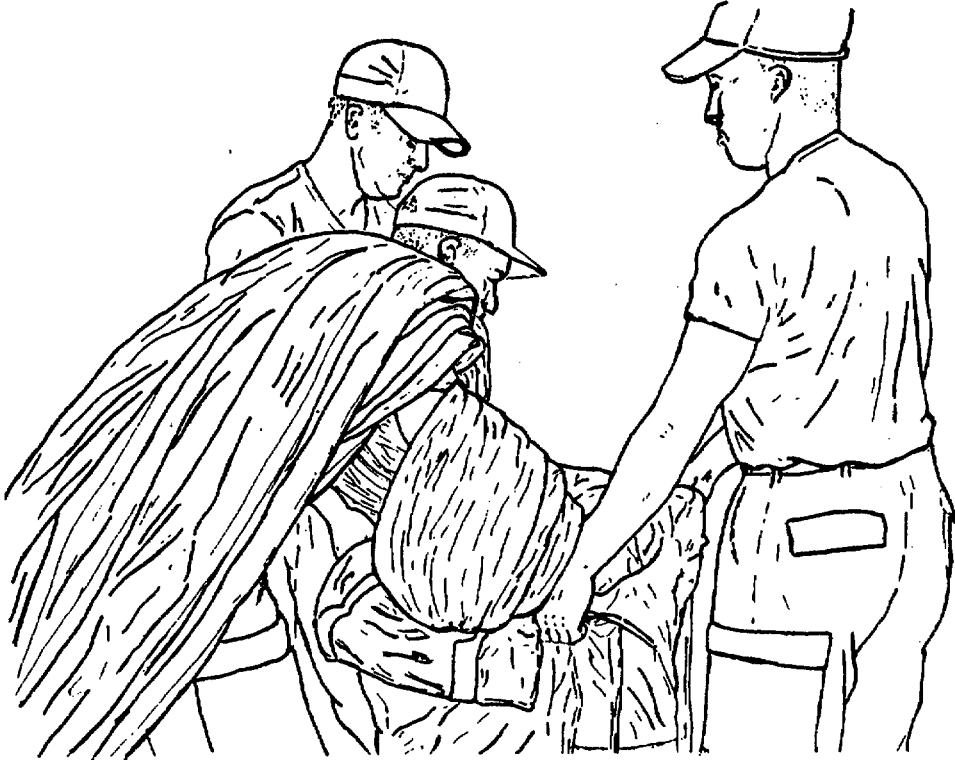
Figure 2-30. Stowing the Canopy in Deployment Bag.
