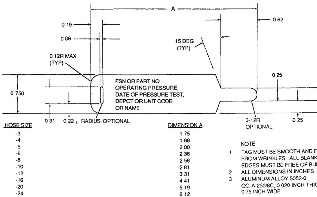
**Figure 4-42. Identification Tags for Field Fabricated Hose Assemblies**
