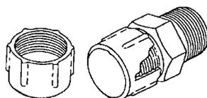
**Figure 4-55. Plastic Protective Dust Cap**
