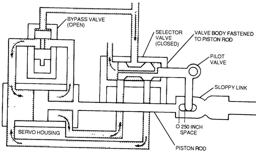
Figure 4-138. Hydraulic Servo
