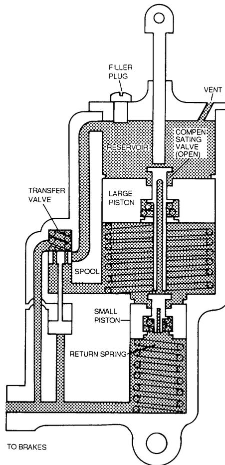
**Figure 4-149. Compound Master Cylinder**
