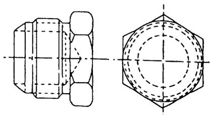
Figure 4-54. Aluminum Protective Dust Plug and Moisture Seal
