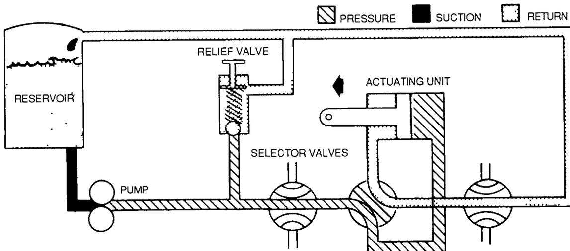
Figure 4-144. Open Center Hydraulic System (Valve Open)
