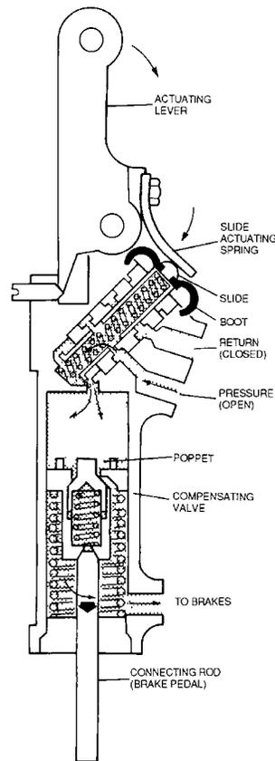
**Figure 4-150. Power-Boost Master Cylinder (Brake Applied)**
