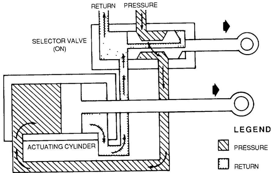
Figure 4-134. Double-Action Actuating Cylinder (Extension)
