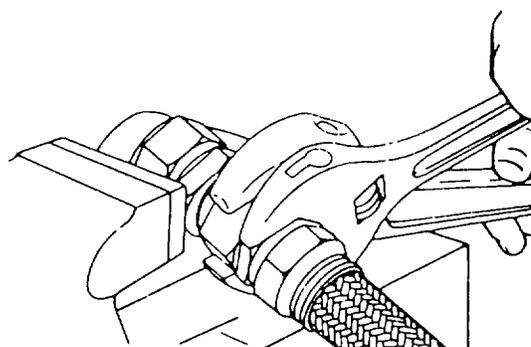
DO — PLACE WRENCH ON NIPPLE HEX TO HOLD LINE WHILE LOOSENING SWIVEL NUT
