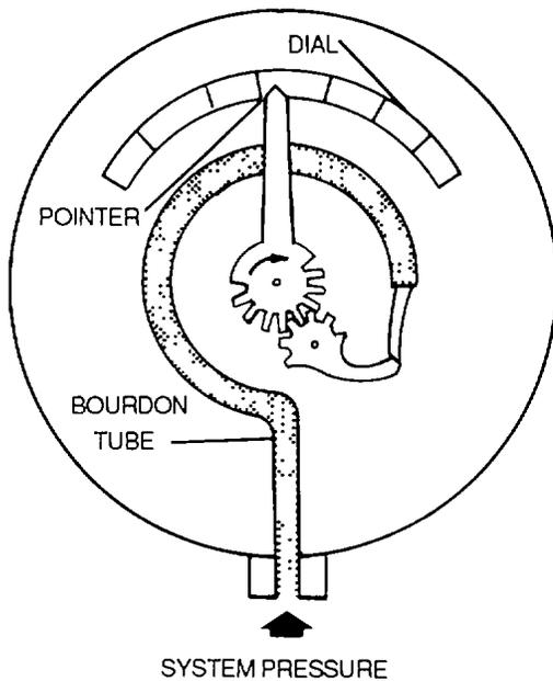
Figure 4-114. Pressure Gauge
