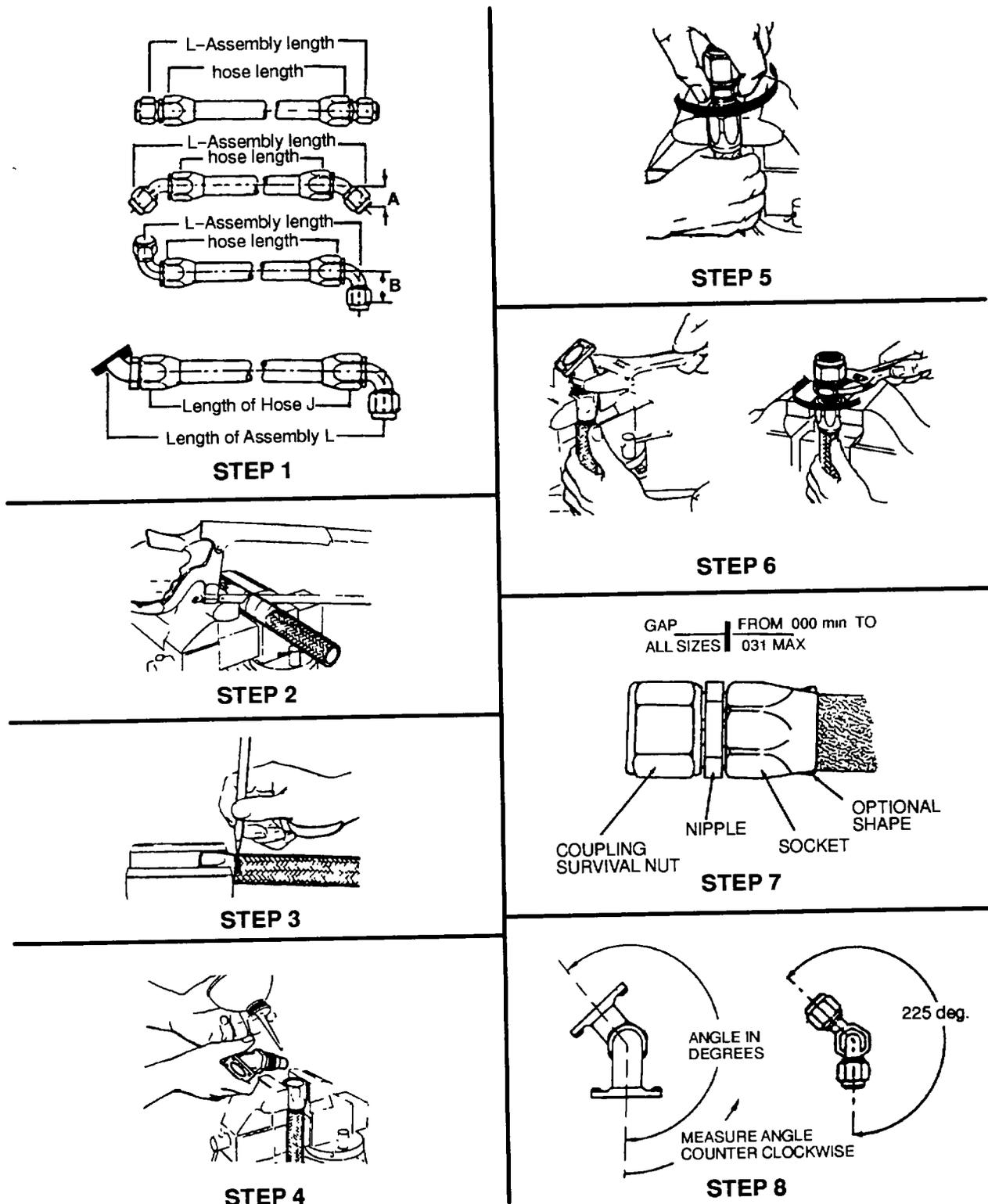
Figure 4-50A. Field Assembly of Lightweight Rubber Hose
