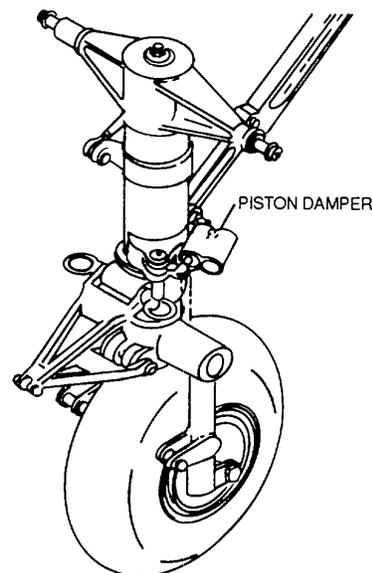
Figure 4-164. Nose Landing Gear with Piston Damper
