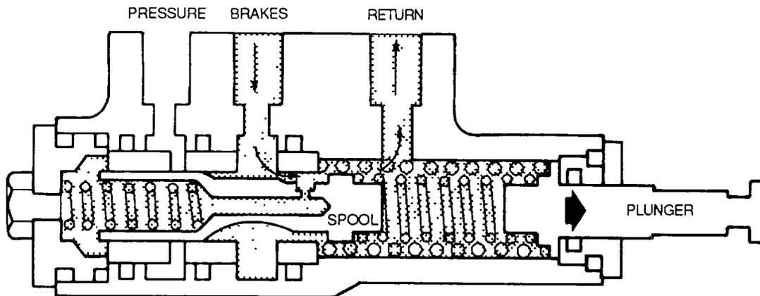
Figure 4-153. Power Brake Control Valve (Brakes Released)
