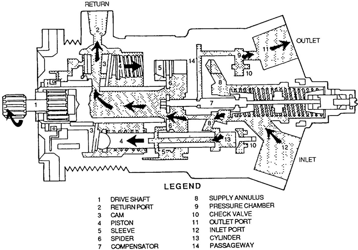
Figure 4-105. Stratopower Effective Stroke Pump (Full Flow)
