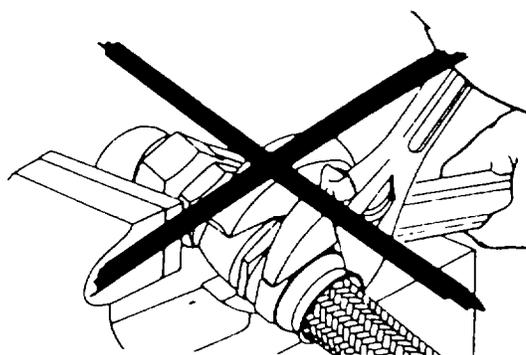
DONT — PLACE WRENCH ON SOCKET FLAT TO HOLD LINE WHILE LOOSENING SWIVEL NUT
