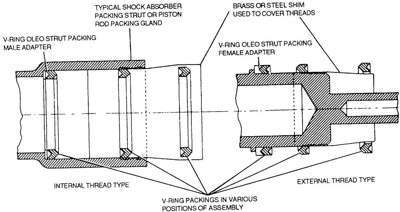
**Figure 4-71. V-Ring Packings in Various Positions of Assembly**
