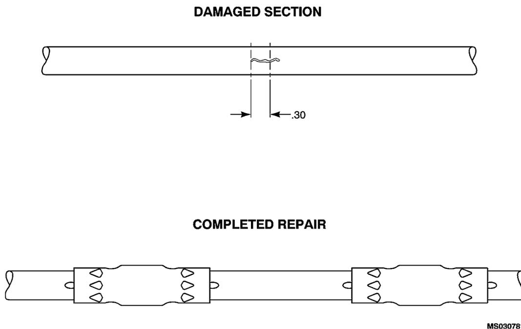
**Figure 4-87. Type 2 Repair, Crack is longer than 0.30"**
