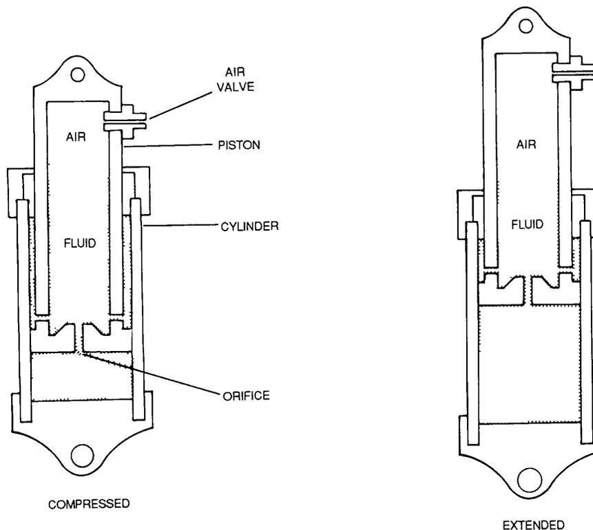
**Figure 4-170. Simple Shock Strut**
