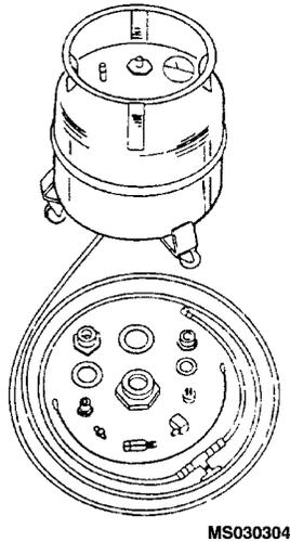
**Figure 3-1. Typical Hydraulic System Filler and Bleeder**
