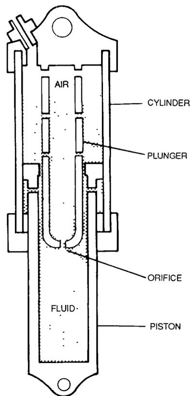
Figure 4-172. Complex Shock Strut (Plunger)
