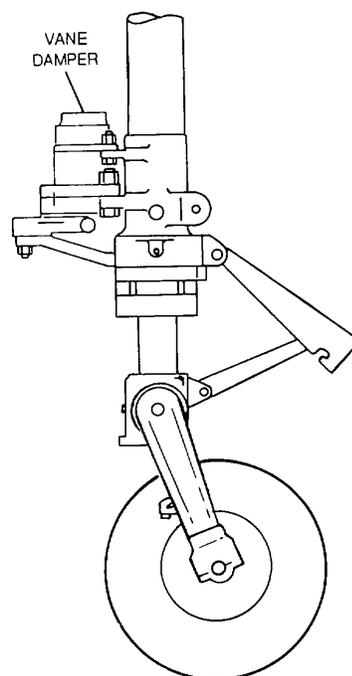
**Figure 4-168. Nose Landing Gear with Vane Damper**
