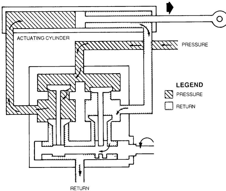
Figure 4-123. In-Line Cam-Operated Selector Valve (Actuator Extending)
