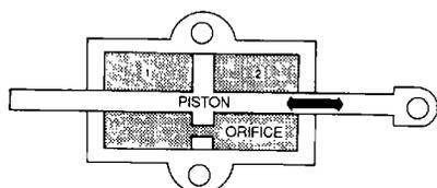
Figure 4-163. Piston Damper Cross Section
