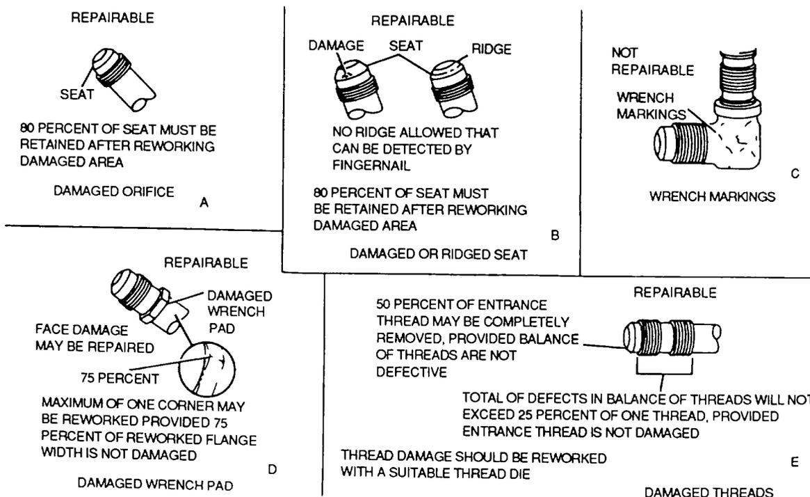
Figure 4-29. Damaged Fittings
