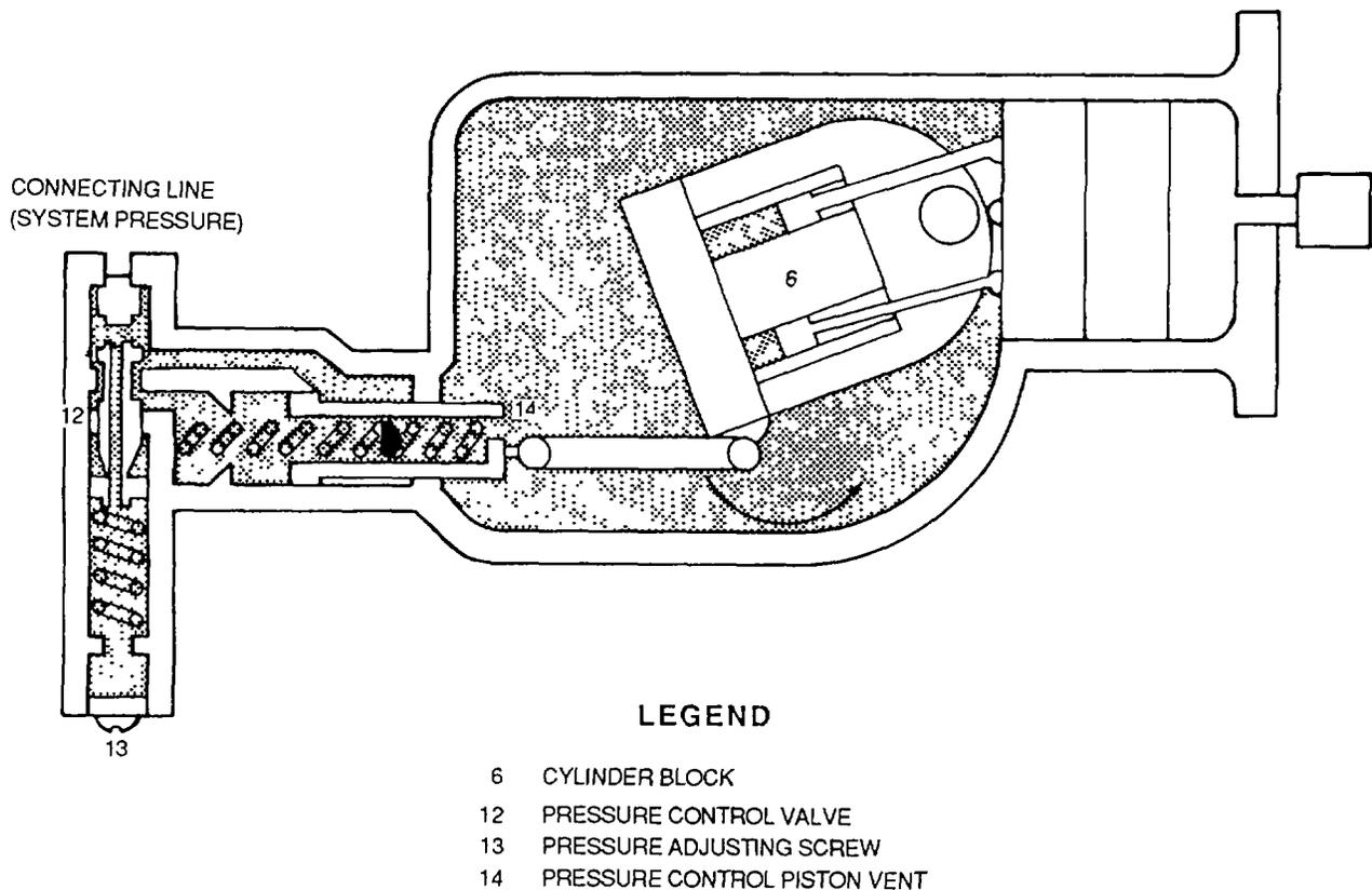
Figure 4-108. Vickers Stroke Reduction Pump (Full Flow)
