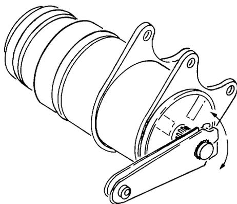
**Figure 4-166. Vane Damper**
