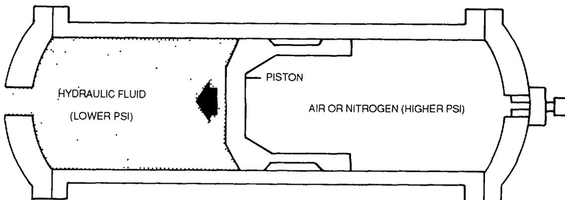
Figure 4-118. Cylindrical Accumulator
