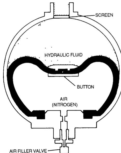
**Figure 4-119. Spherical Accumulator**
