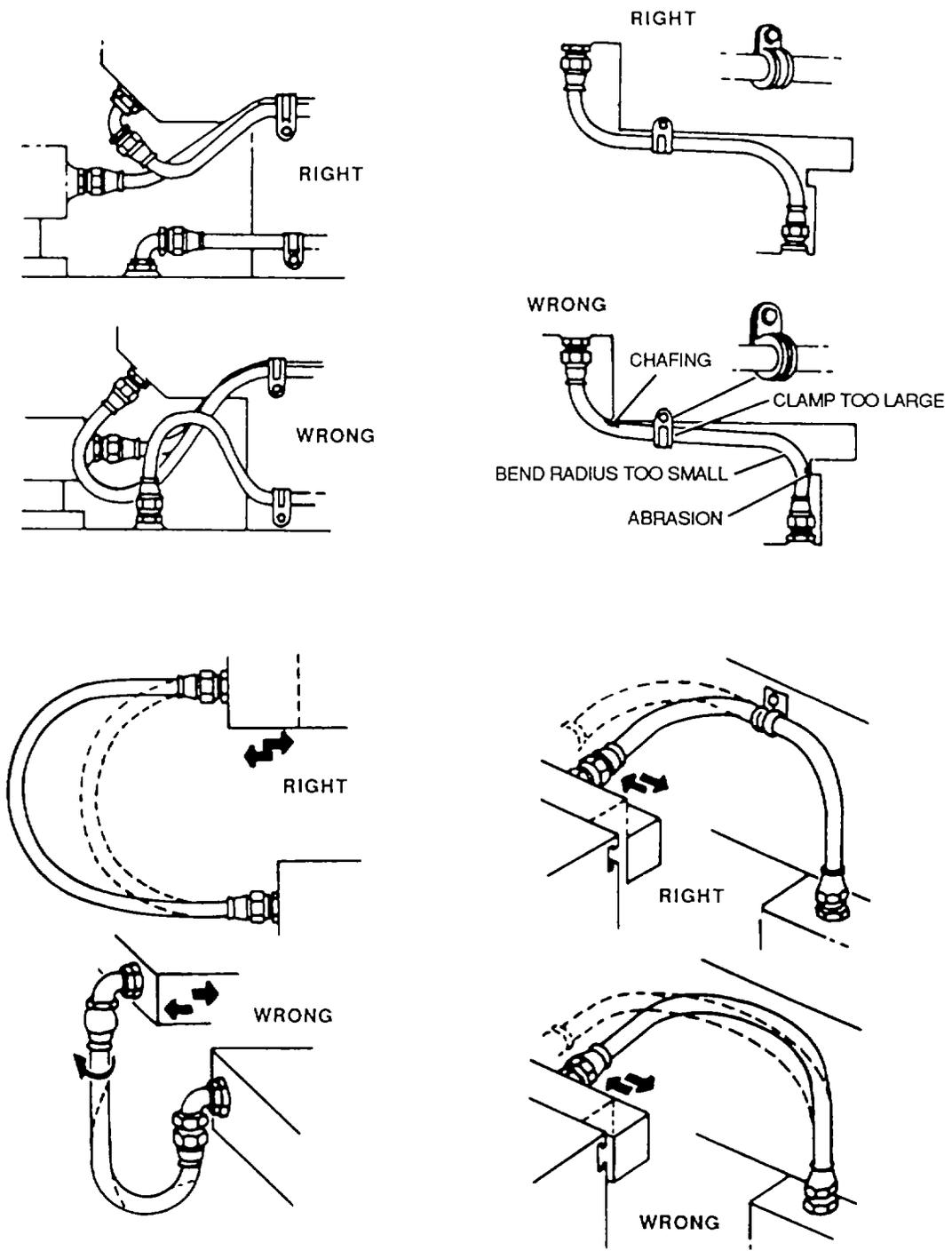
Figure 4-49. Teflon Hose Installation Procedures, Right and Wrong
