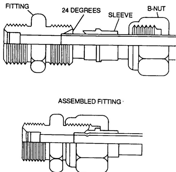
Figure 4-17. MS Fitting and Components
