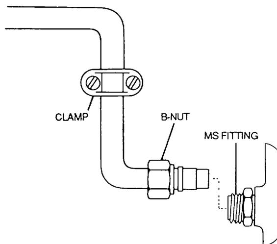
Figure 4-20. Tubing Alignment
