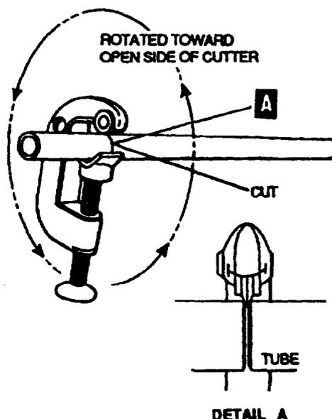
Figure 4-3. Cutting Tube with Tube Cutter.
