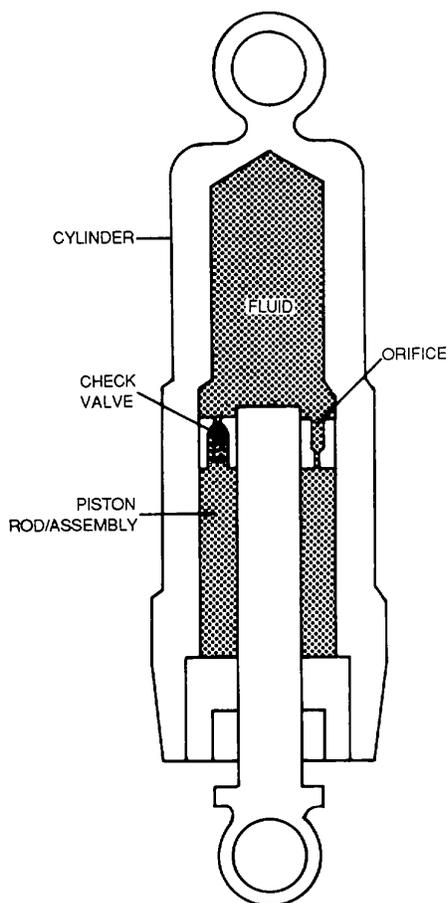
**Figure 4-175. Liquid Spring**
