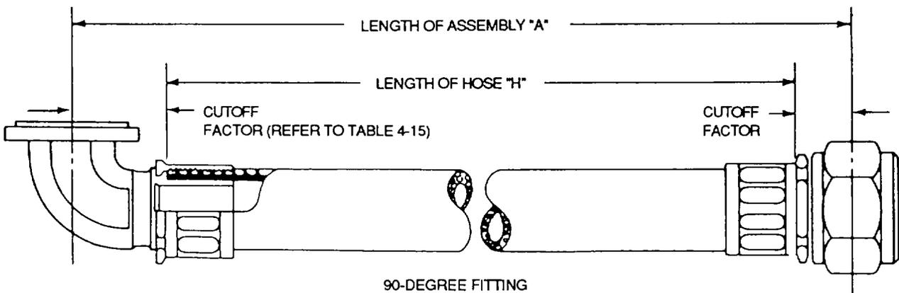
Figure 4-40. Determining Hose Assembly Length
