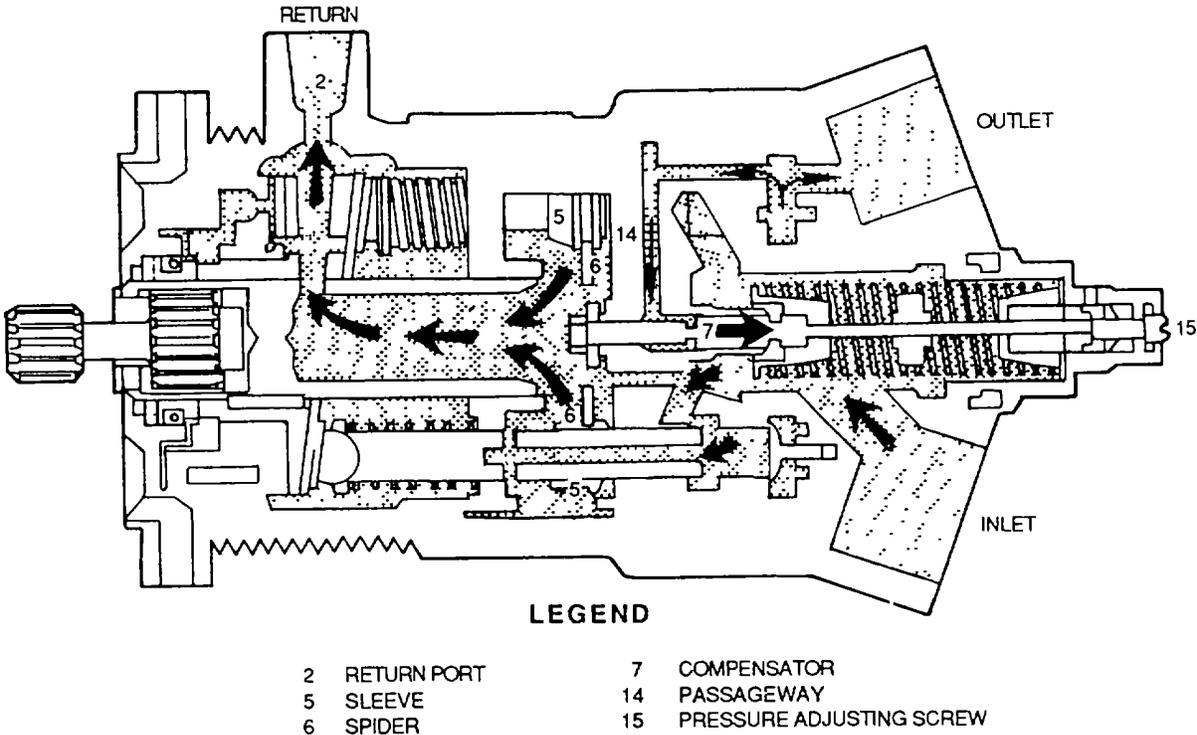
Figure 4-106. Stratopower Effective Stroke Pump (Zero Flow )
