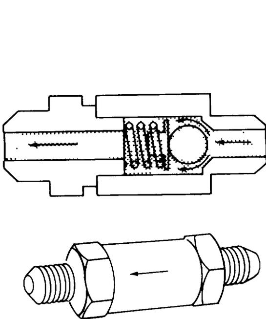
Figure 4-127. Simple Check Valve
