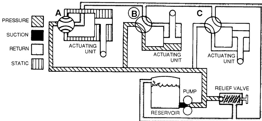
Figure 4-146. Selector Valve B Open
