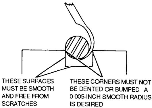
Figure 4-60. Removing O-Ring
