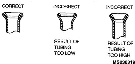
**Figure 4-11. Tubing with Double Lap Flare**
