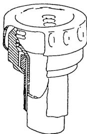
Figure 4-52. Steel Protective Dust Plug and Moisture Seal
