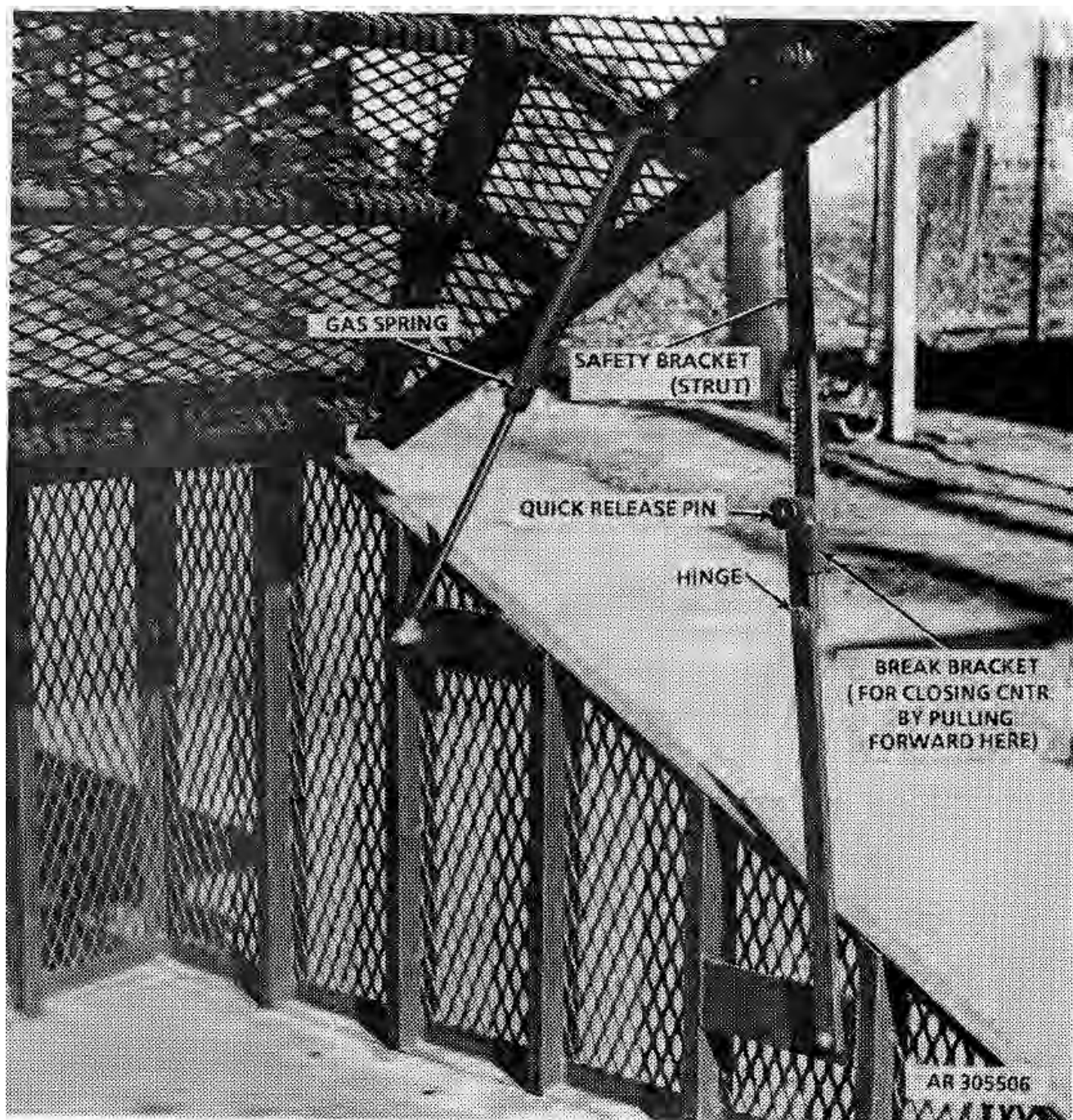
Figure 1-5. Details of Support Bracket and Gas Spring
