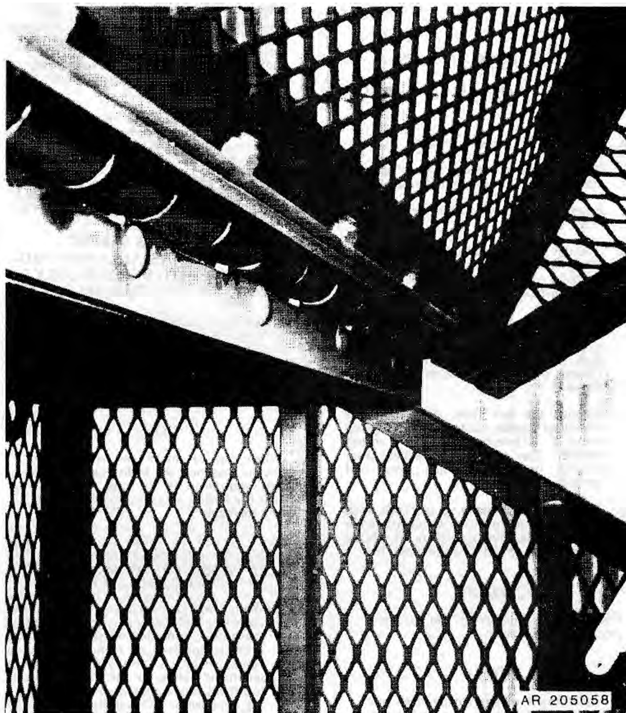
Figure 2-2. Hinge and Mounting from Underside of cage.
