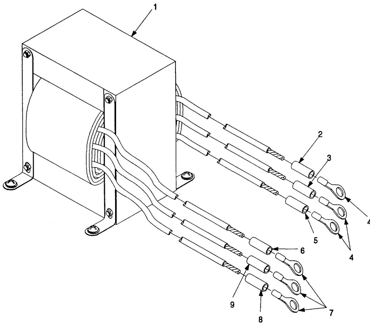
Figure 18. Transformer Assembly 9354036.
