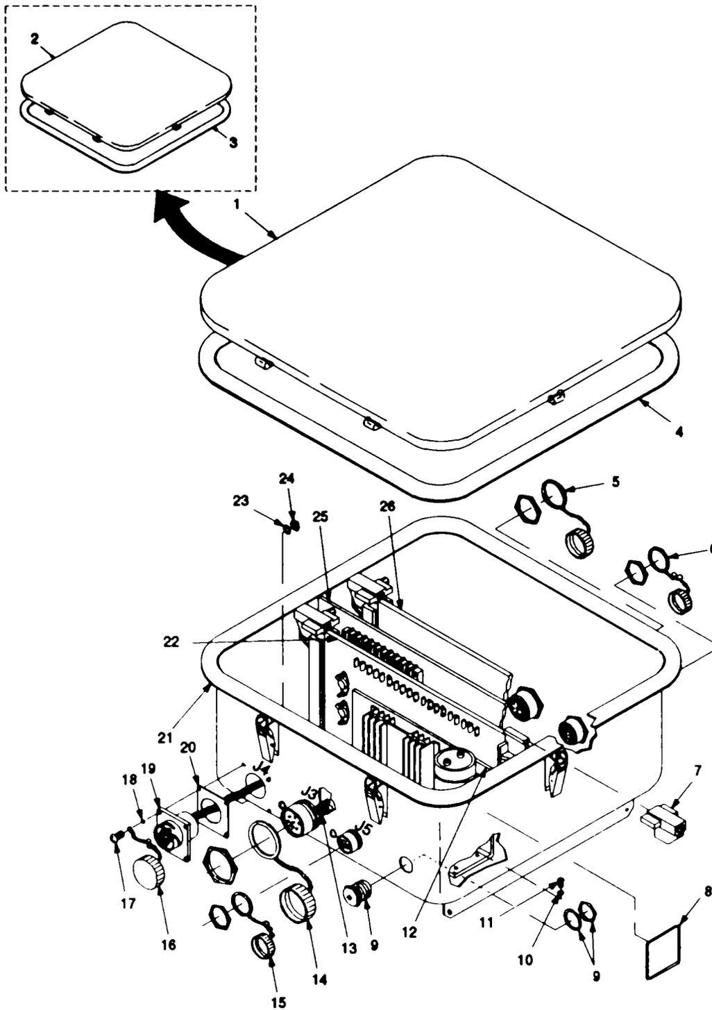
Figure 1. Interconnecting Box, Target Interface 9353787 (Sheet 1 of 3).
