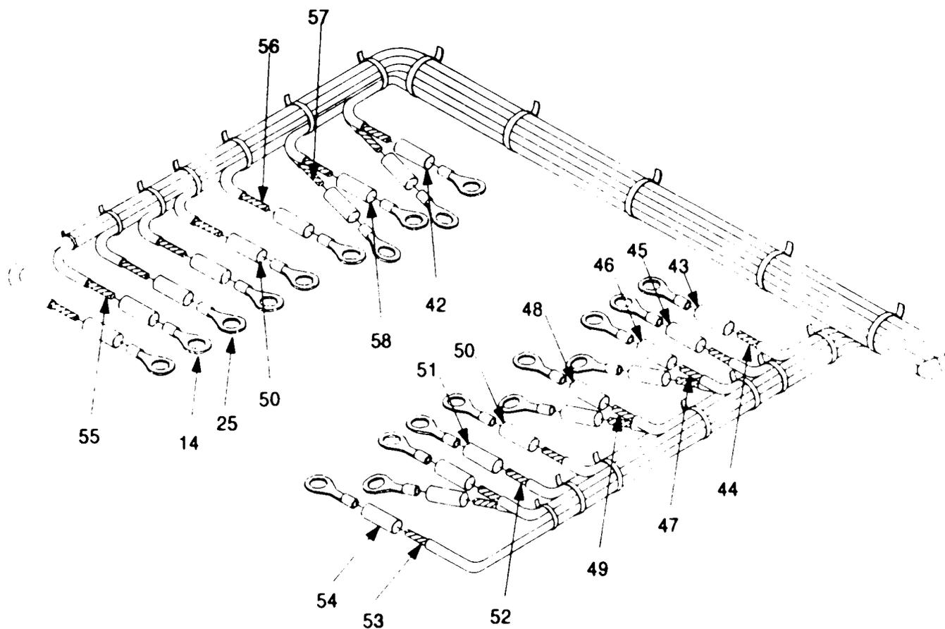
Figure 5. Wiring Harness 9353793 (Sheet 3 of 3).
