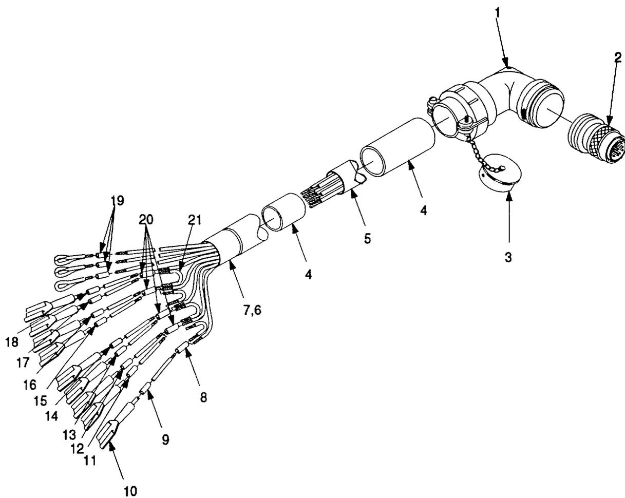
Figure 22. Cable, Special Purpose 9354096-1.
