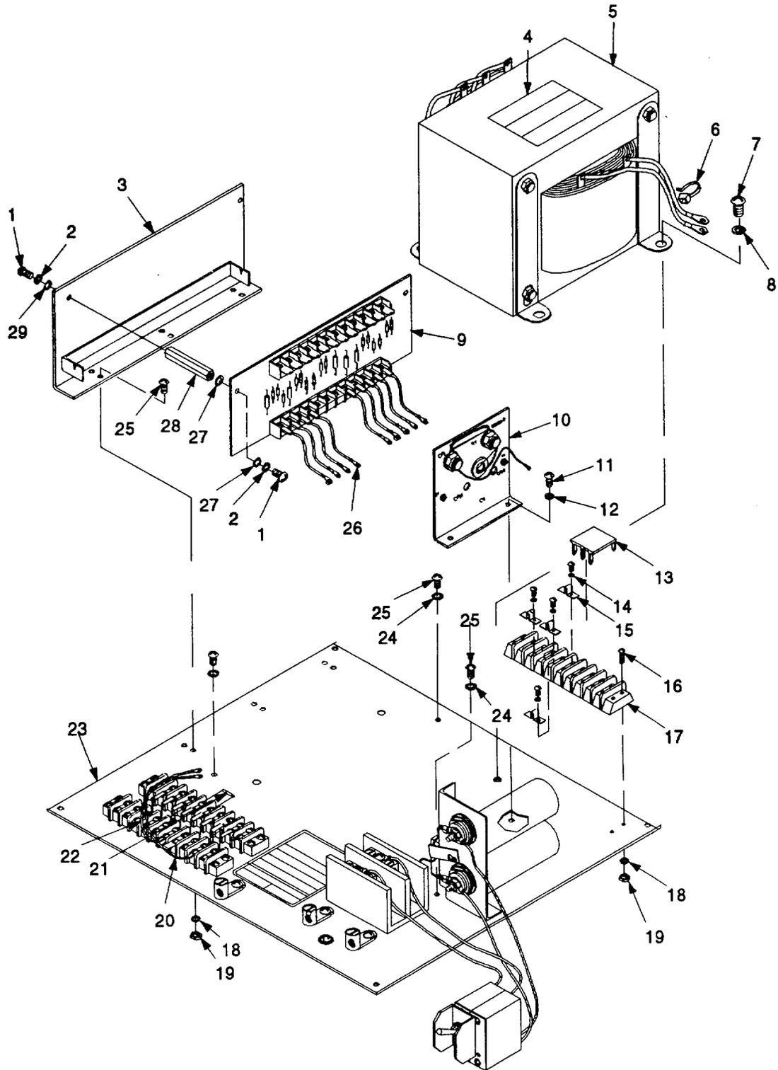
Figure 8. Interconnecting Box, High Power 9353786 (Sheet 1 of 3).
