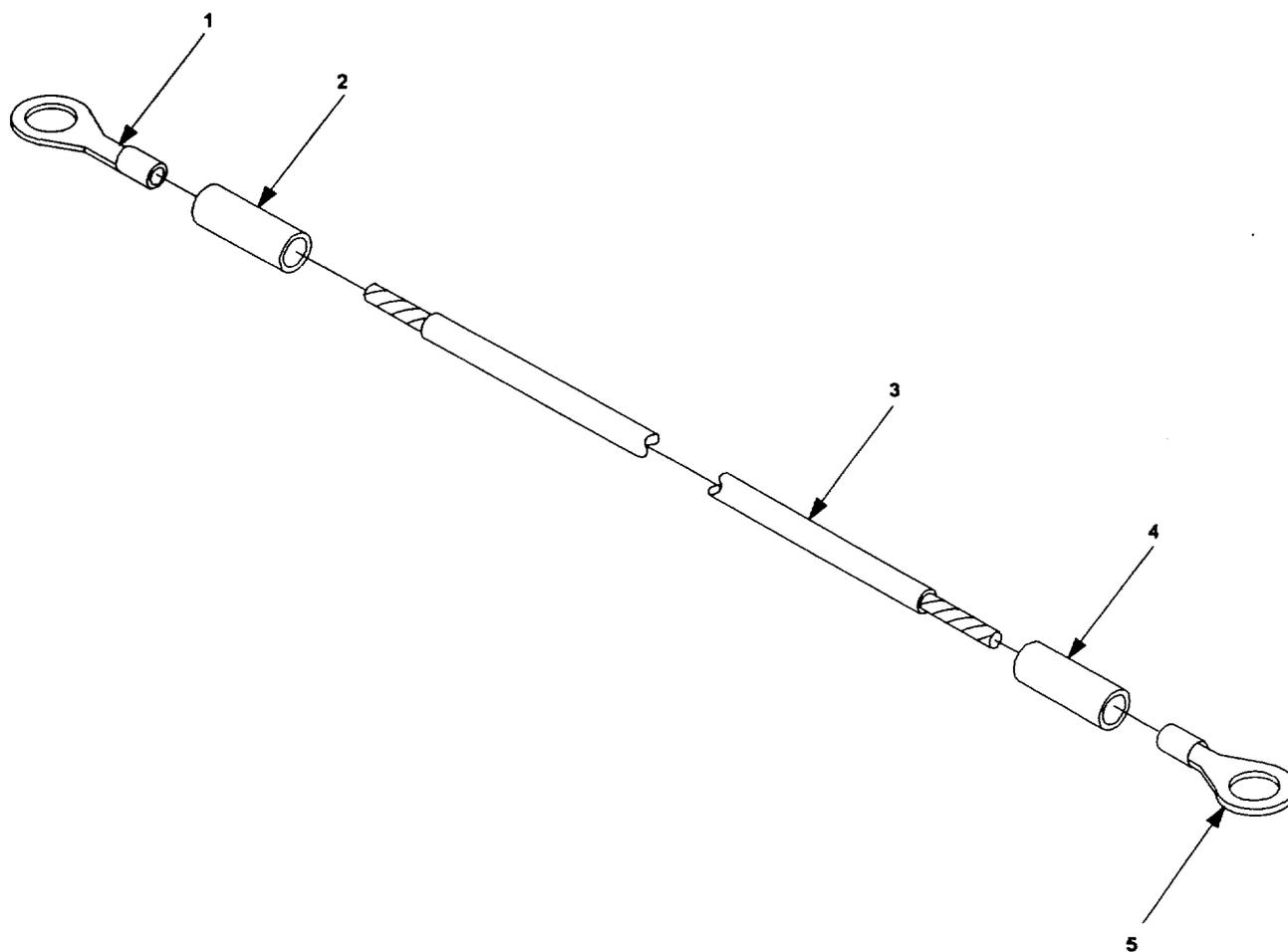
Figure 12. Jumper Assembly 9387197-1.
