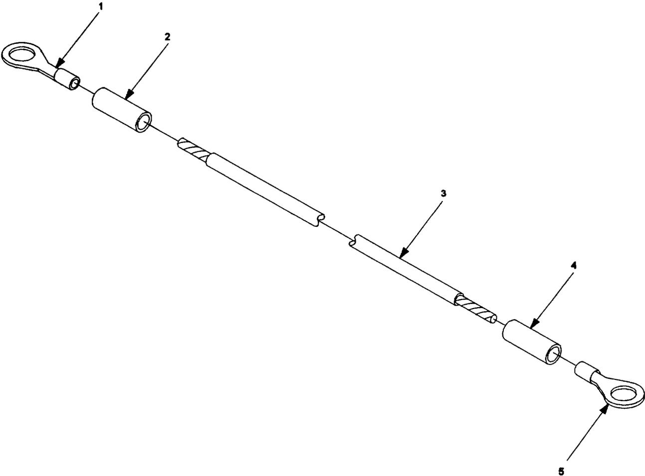
Figure 21. Jumper Assembly 9387197-2.
