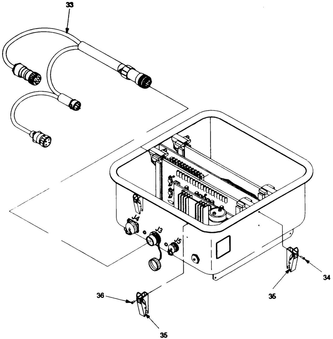
Figure 1. Interconnecting Box, Target Interface 9353787 (Sheet 3 of 3).
