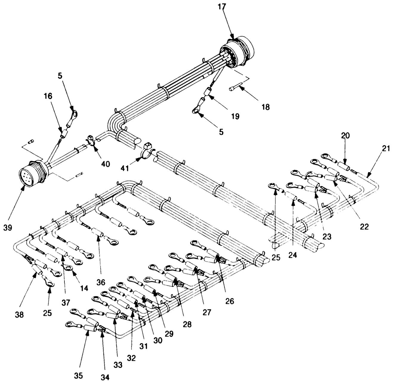
Figure 5. Wiring Harness 9353793 (Sheet 2 of 3).
