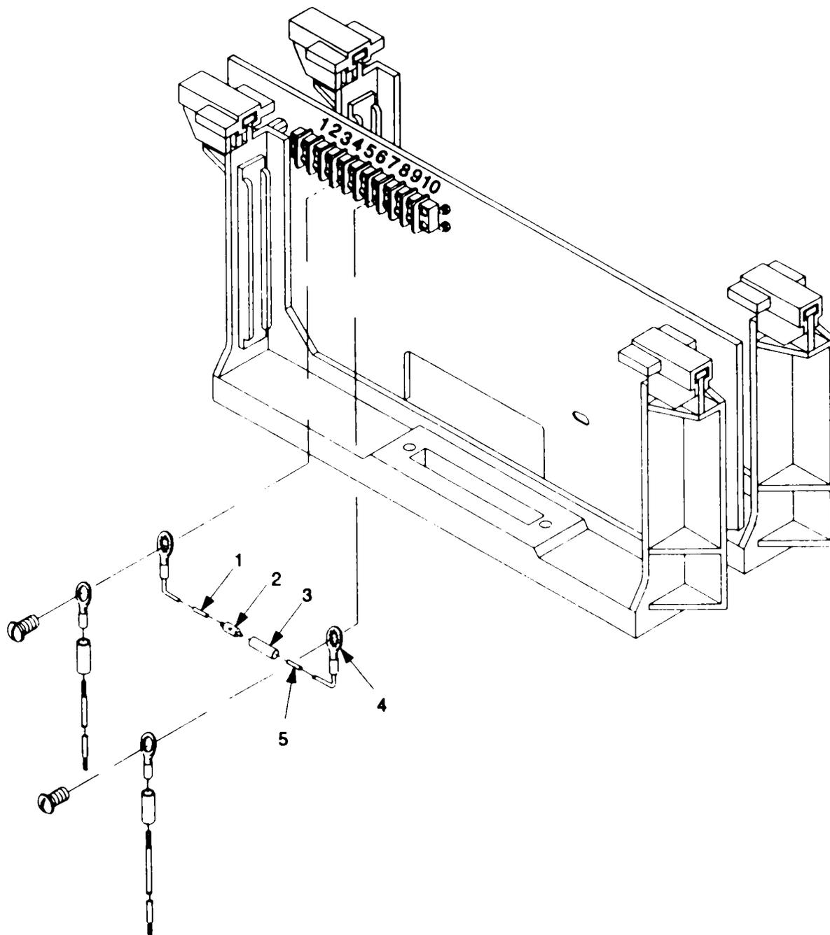
Figure 4. Transient Suppressor 9354186-3.
