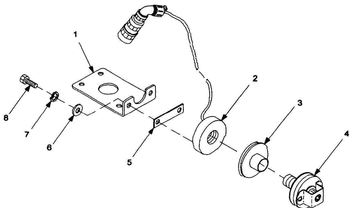
Figure 35. Hit Sensor Assembly 9363053.
