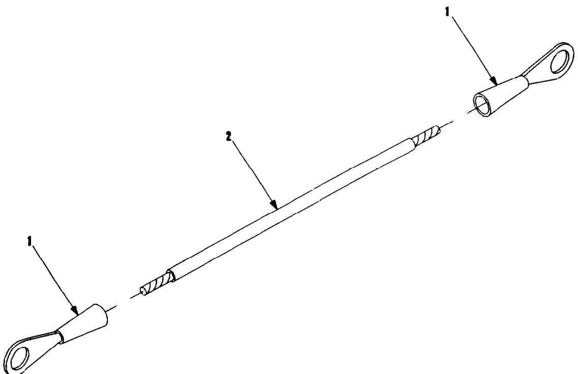
Figure 17. Wire, Bonding 9353984.
