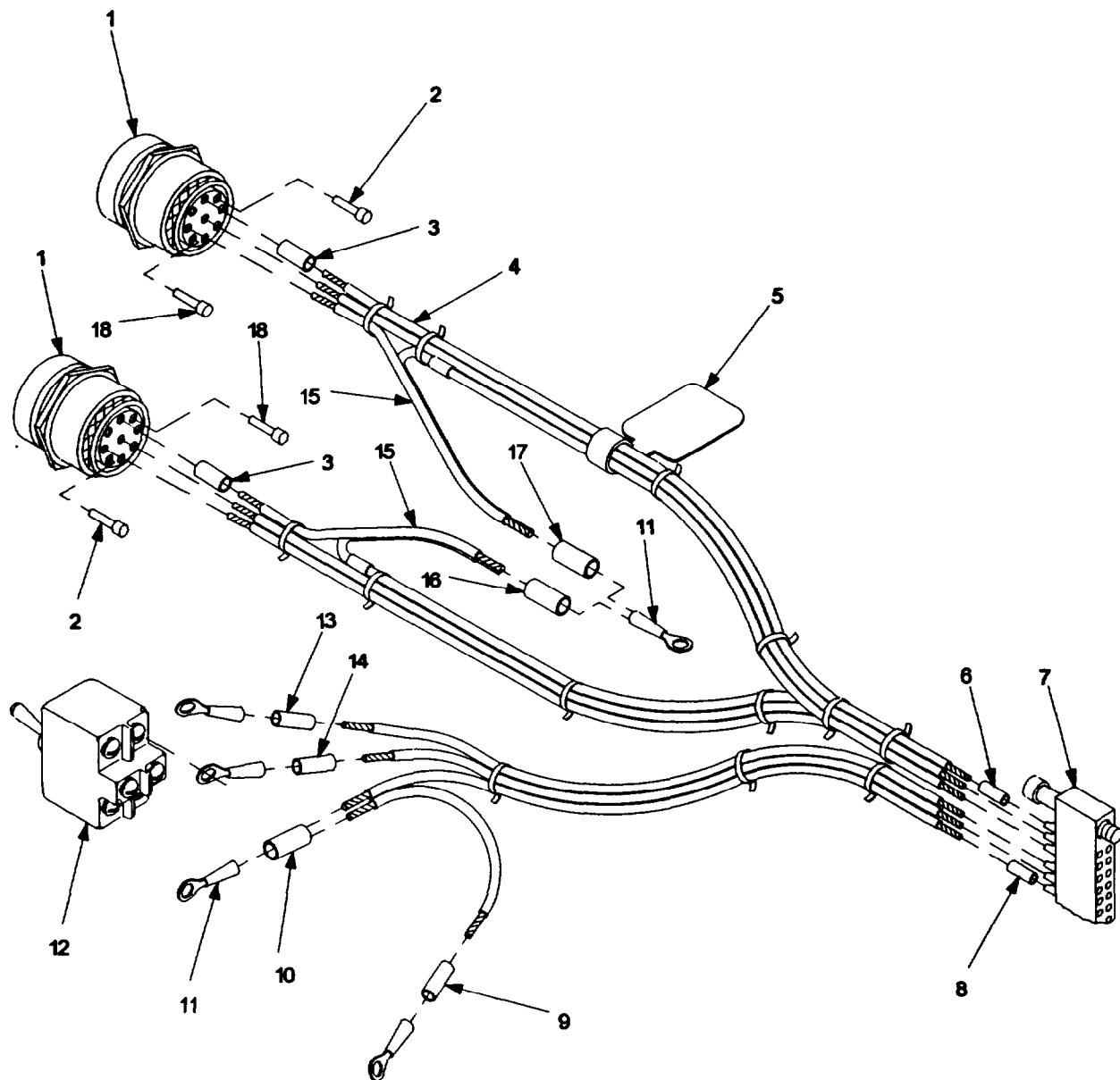
Figure 26. Cable Assembly 11829463 (Sheet 1 of 2).
