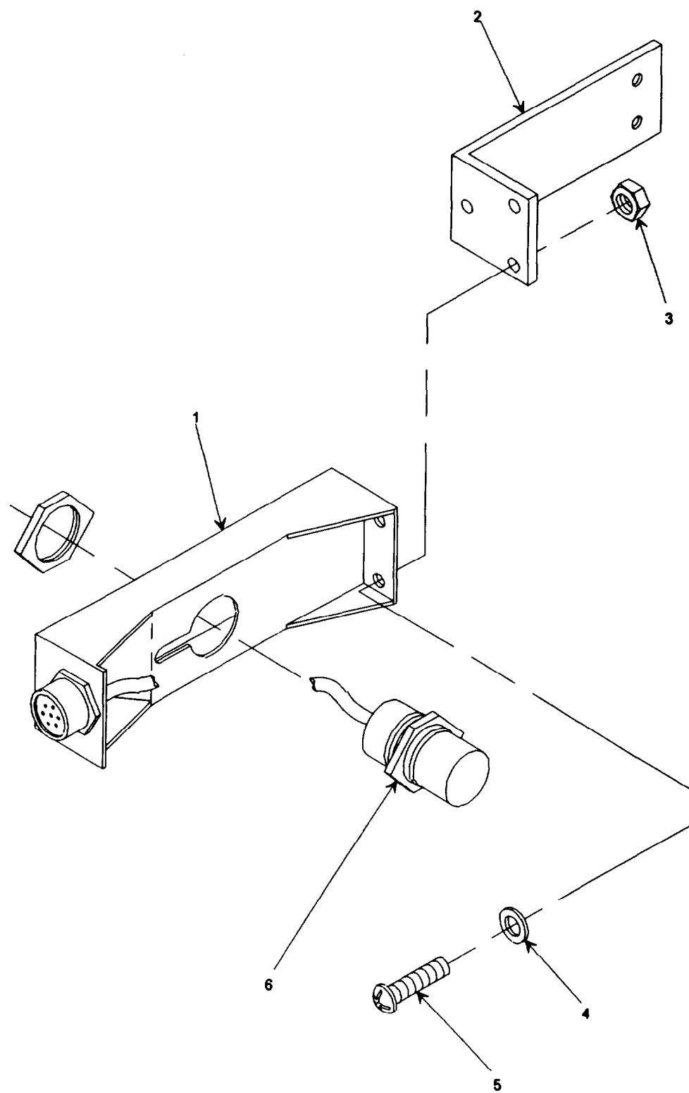
**Figure 19. Bracket Assembly 9353990.**
