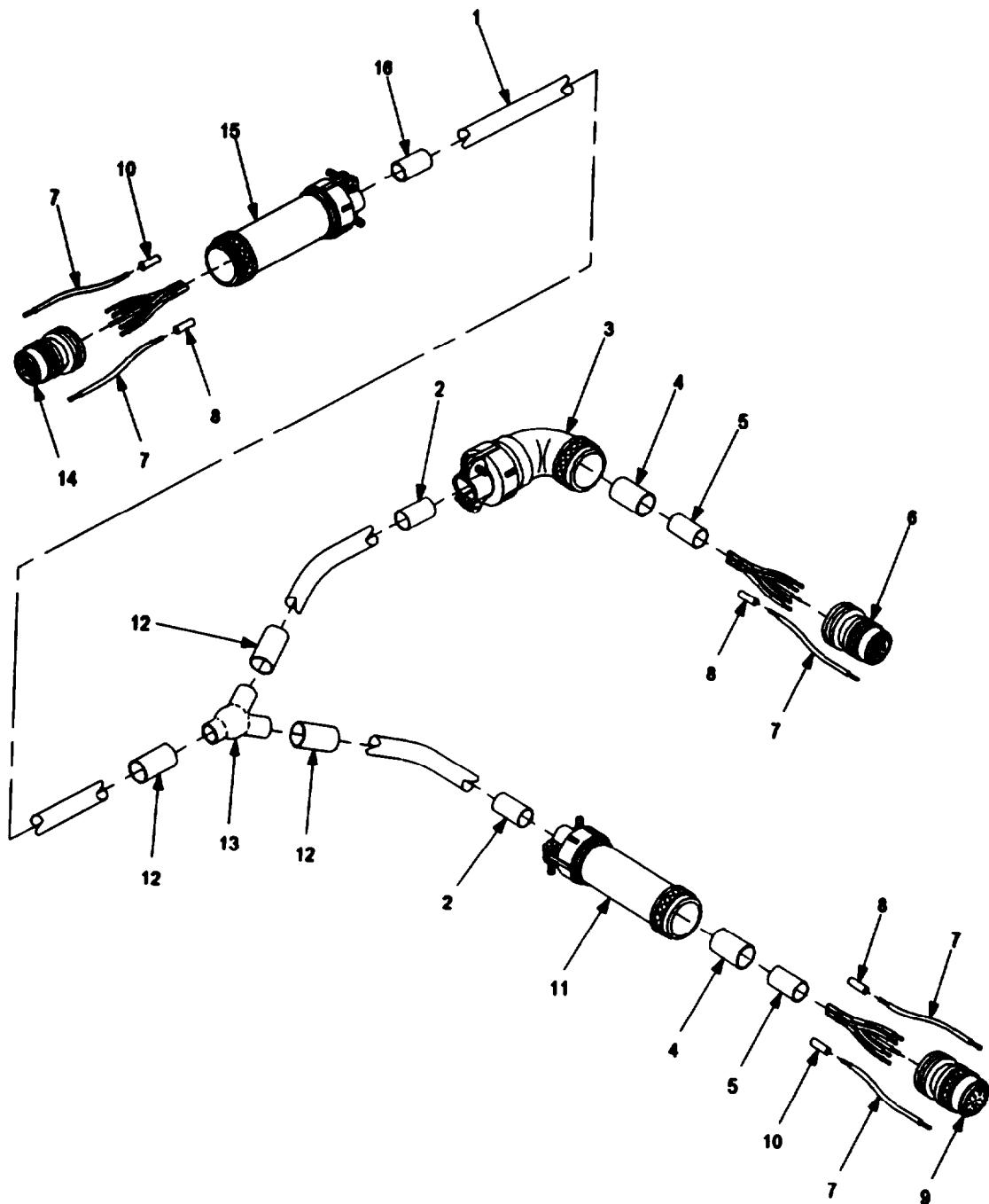
Figure 31. Cable Assembly, Special 9354099.
