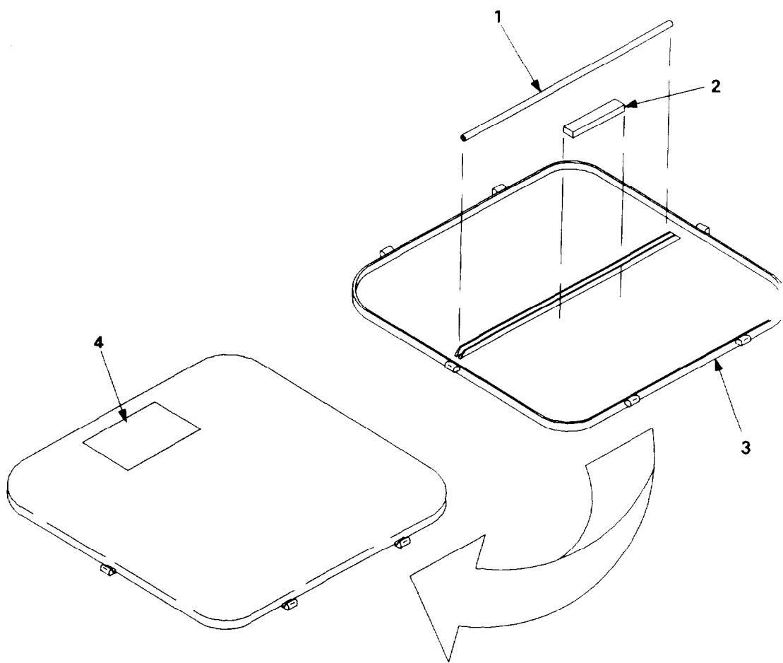
Figure 33. Cover, Electronic Communication 11829343-1.
