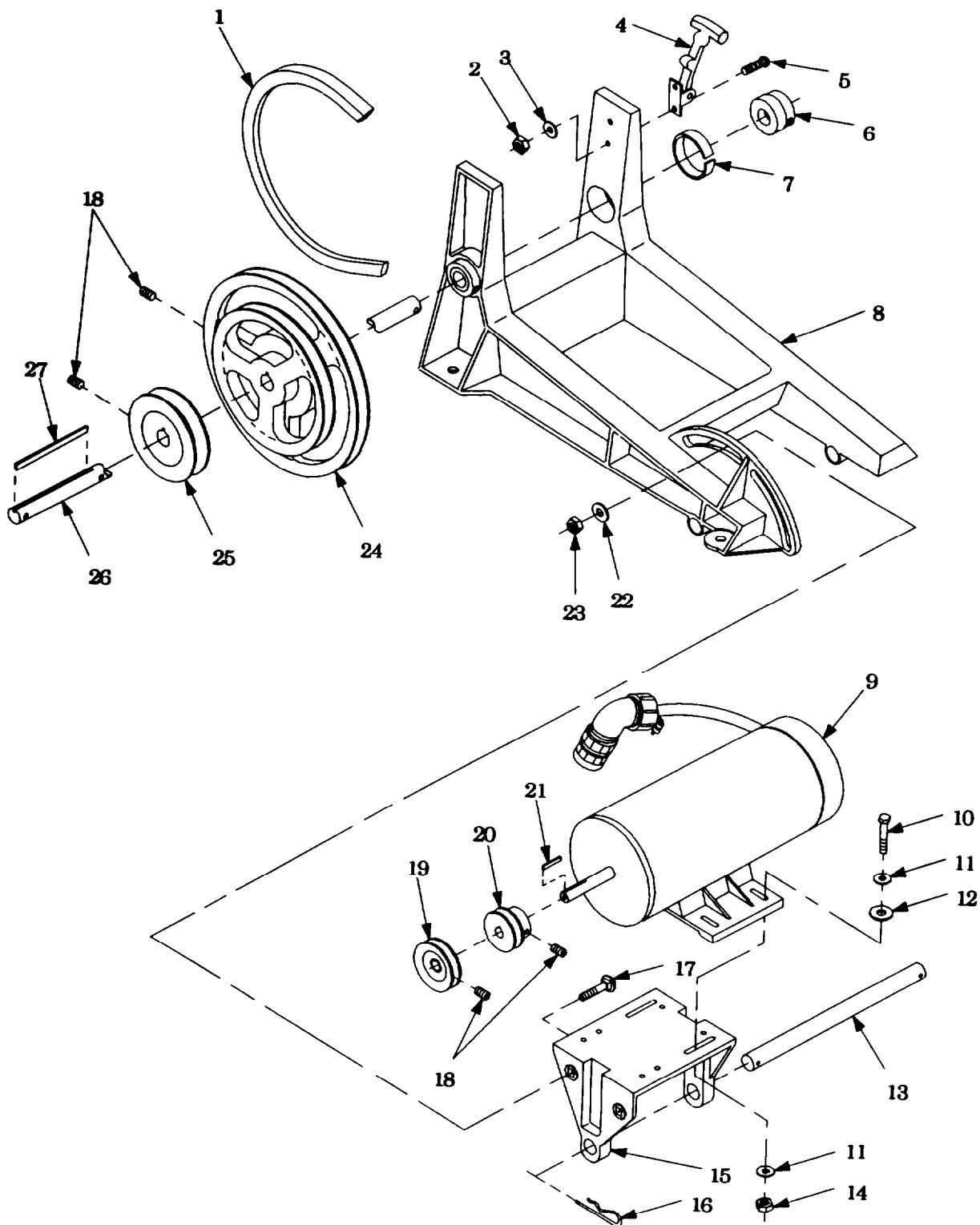
Figure 13. Actuator, Electro-Mechanical 9340977.
