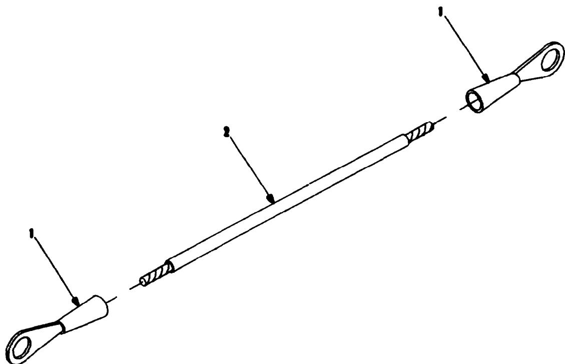
Figure 11. Wire, Bonding 9353984
