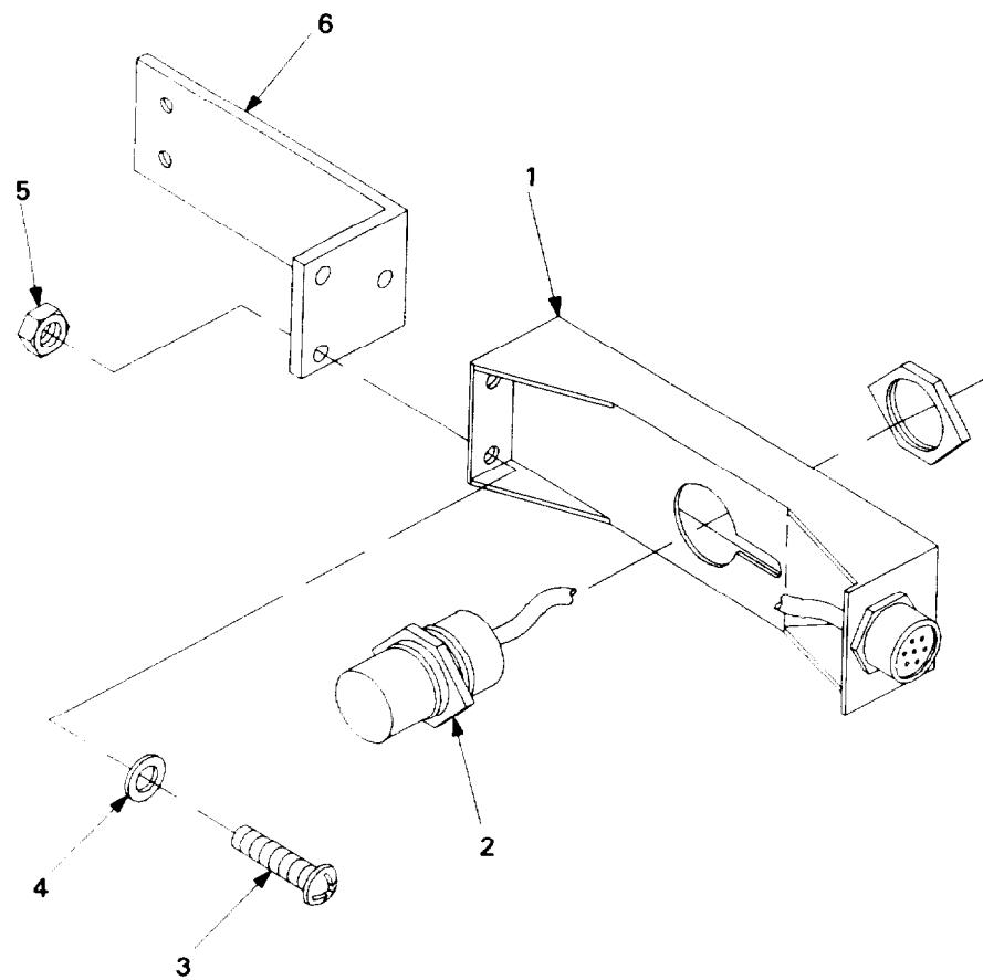
Figure 10. Bracket Assembly 9353990.
