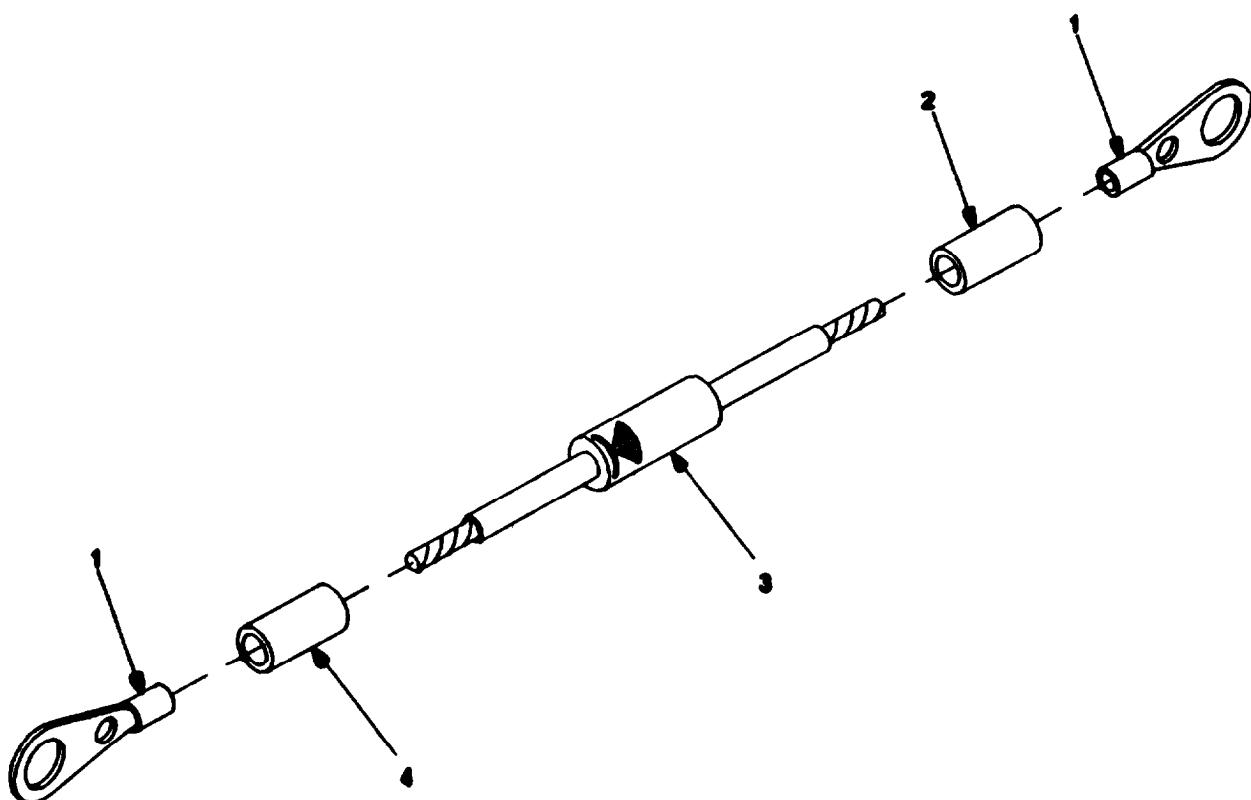
Figure 22. Jumper Diode (9353927-1)
