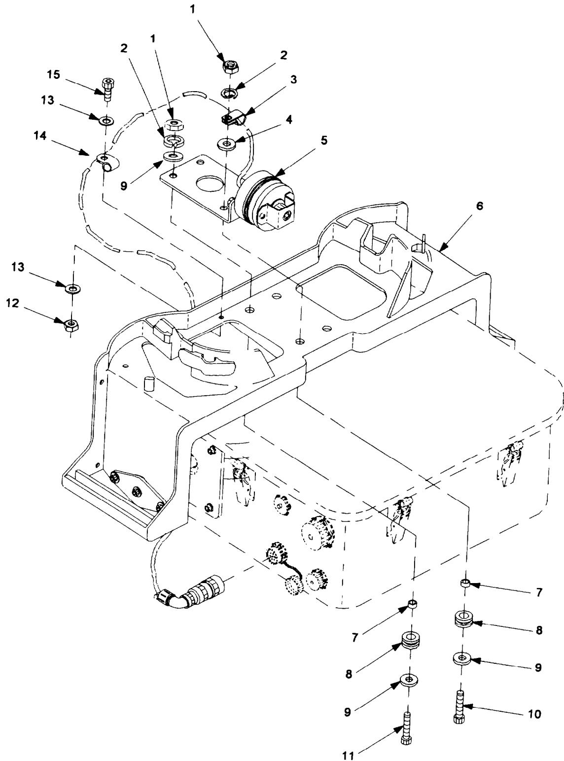
Figure 34. Target Arm Assembly 11829342.
