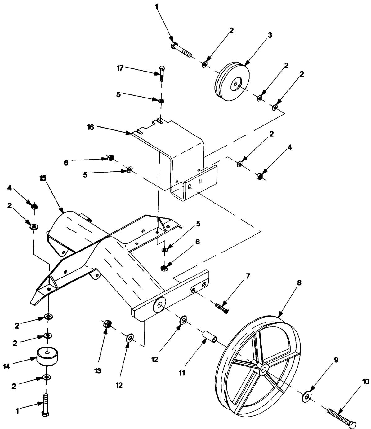
Figure 29. Trolley Assembly 11829747.
