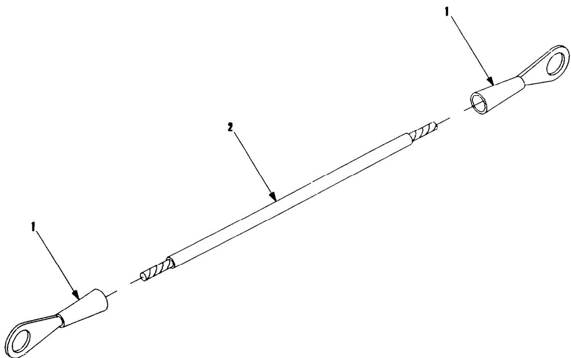
Figure 8. Wire, Bonding 9353984.
