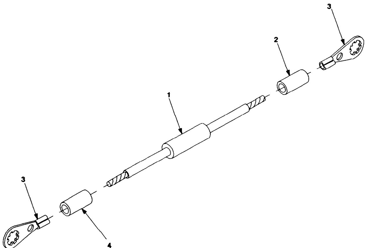
Figure 24. Resistor Assembly 9354191.
