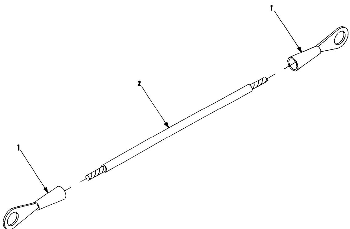
**Figure 6. Wire, Bonding 9353984.**
