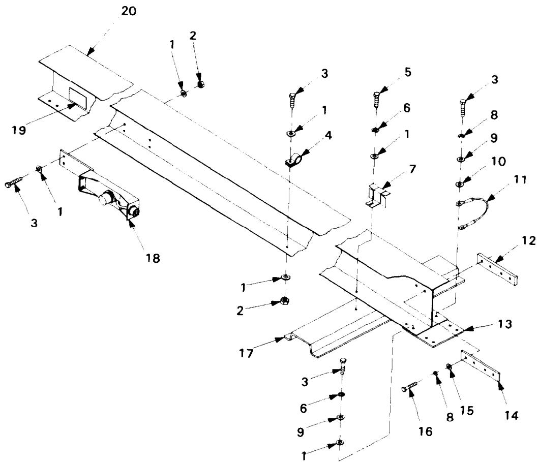
Figure 9. Track Assembly, Drive 9340981.
