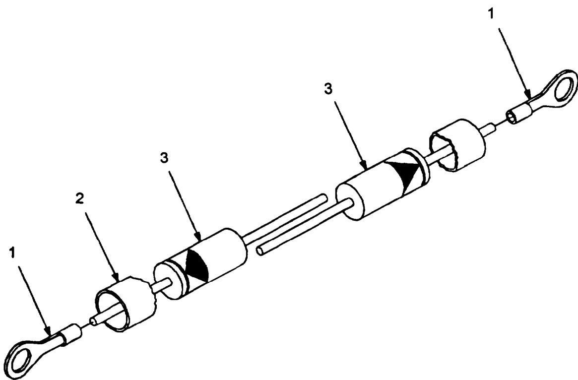
Figure 16. Suppressor Assembly 9387289.
