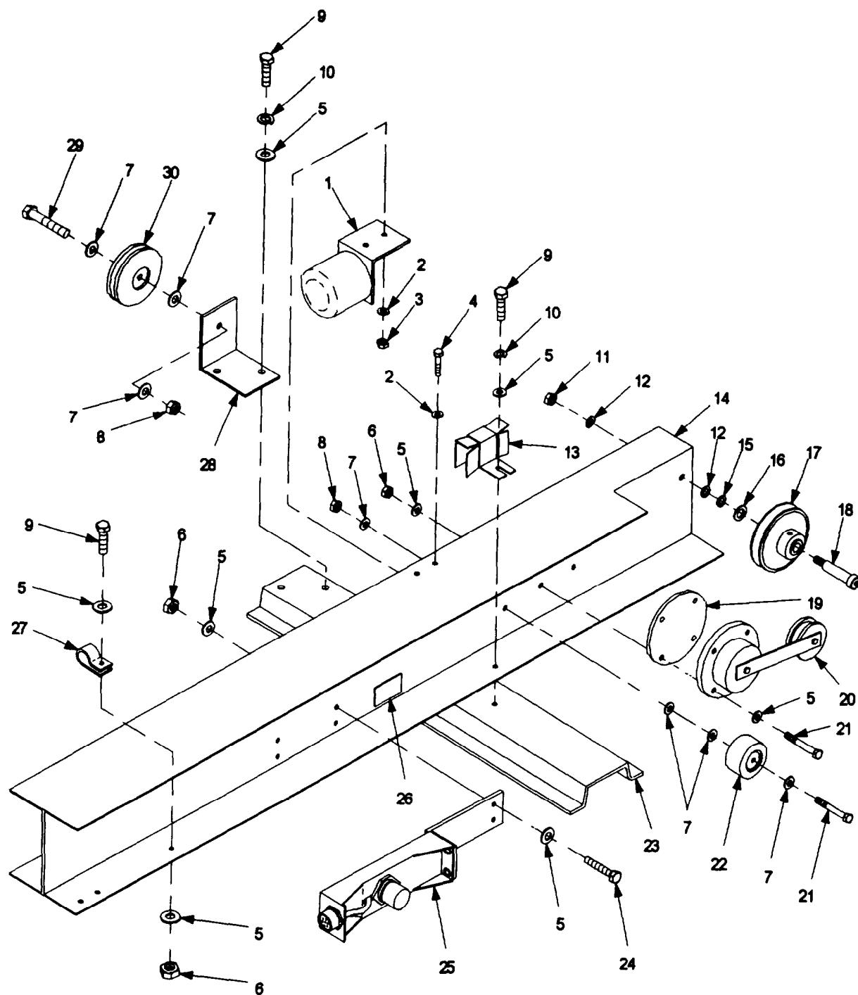
Figure 18. Track Assembly, Return 9340978.
