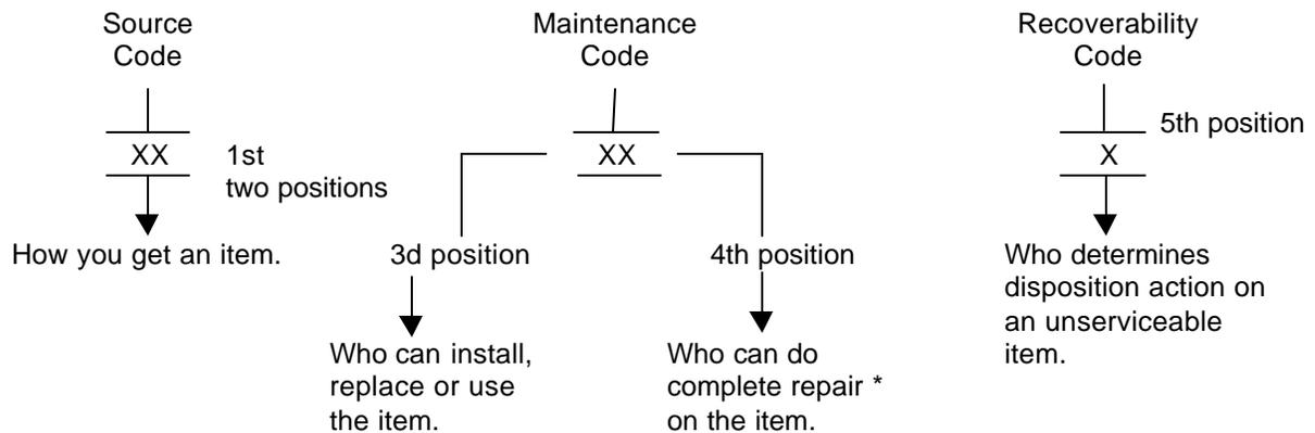
\*Complete Repair: Maintenance capacity, capability, and authority to perform all the corrective maintenance tasks of the "Repair" function in a use/user environment in order to restore serviceability to a failed item.
