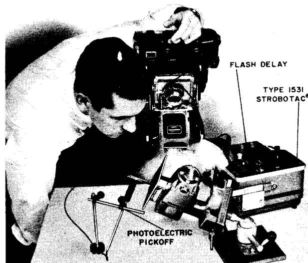
Figure 2-4. Stroboscope, Flash Delay, and Photoelectric Pickoff used for high-speed photography.
