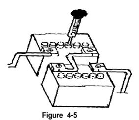
a. Use an hydrometer and draw enough fluid from battery cell to allow indicator to float freely (see Figure 4-5).
