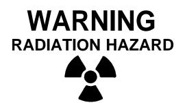
The antireflective coating on all infrared optics contains slightly radioactive thorium fluoride. Potential hazard may result from ingestion (swallowing or inhaling) of this coating material. Dispose of broken lenses and optics in accordance with AR 385-11.
