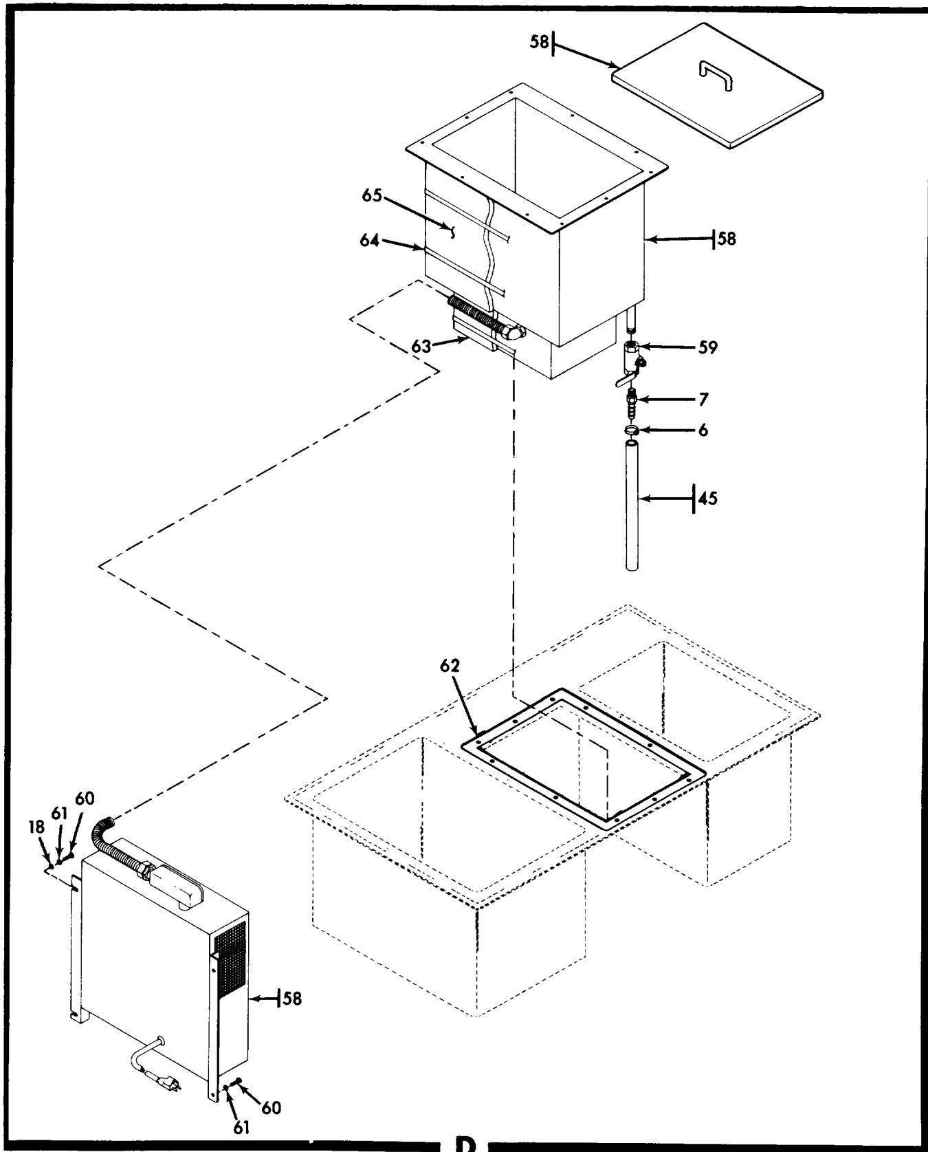
Figure 10. Cleaning Station (3304301-1) (Group 0206) (Sheet 4 of 7)
