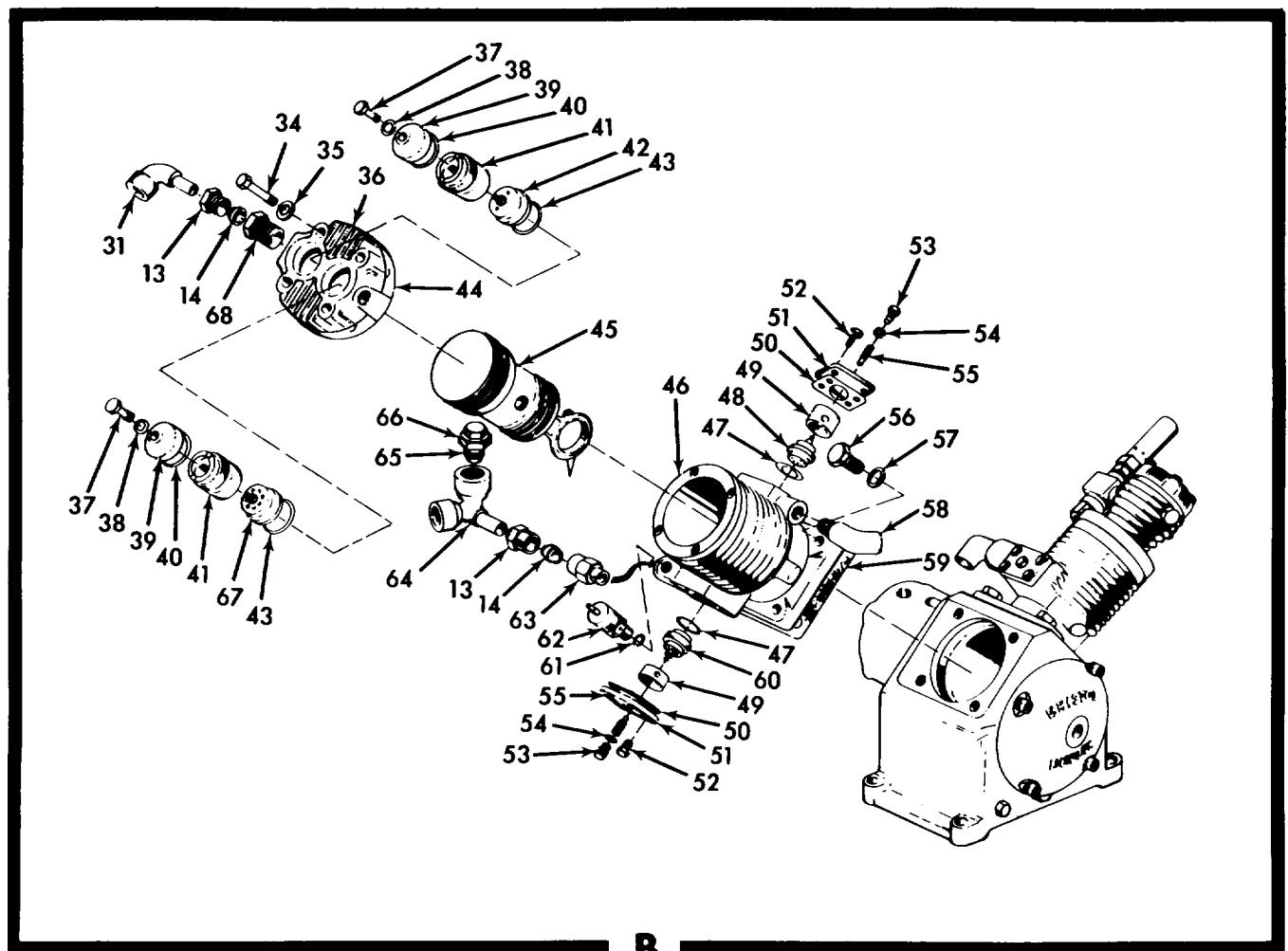
Figure 38. Compressor, Reciprocal (3304739-1) (Group 021302) (Sheet 2 of 3)
