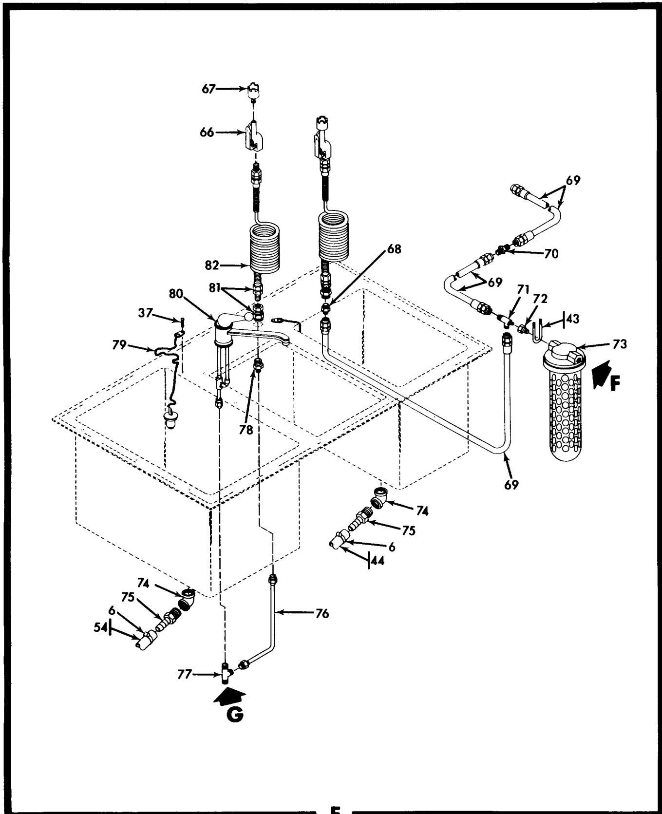
Figure 10. Cleaning Station (3304301-1) (Group 0206) (Sheet 5 of 7)
