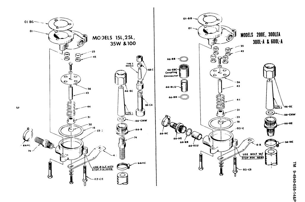
This sandblast is a Model 200 equippea with the mixing valve assembly used on a Model 100 sandblast to facilitate the use of 3/32", 7/64" and 1/8" nozzles and 1/21" I D sandblast hose.
