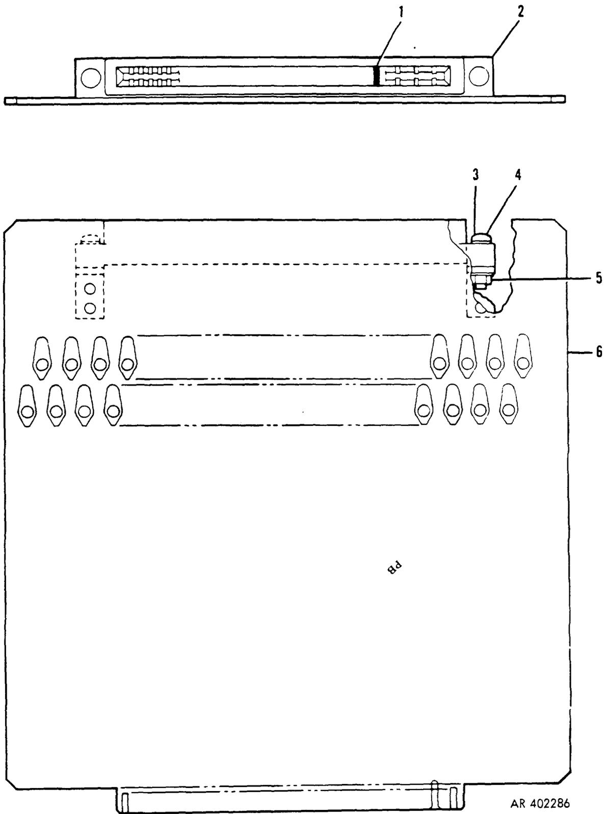
Figure 9. Low Voltage Power Supply Extender Card Assembly-10559515
