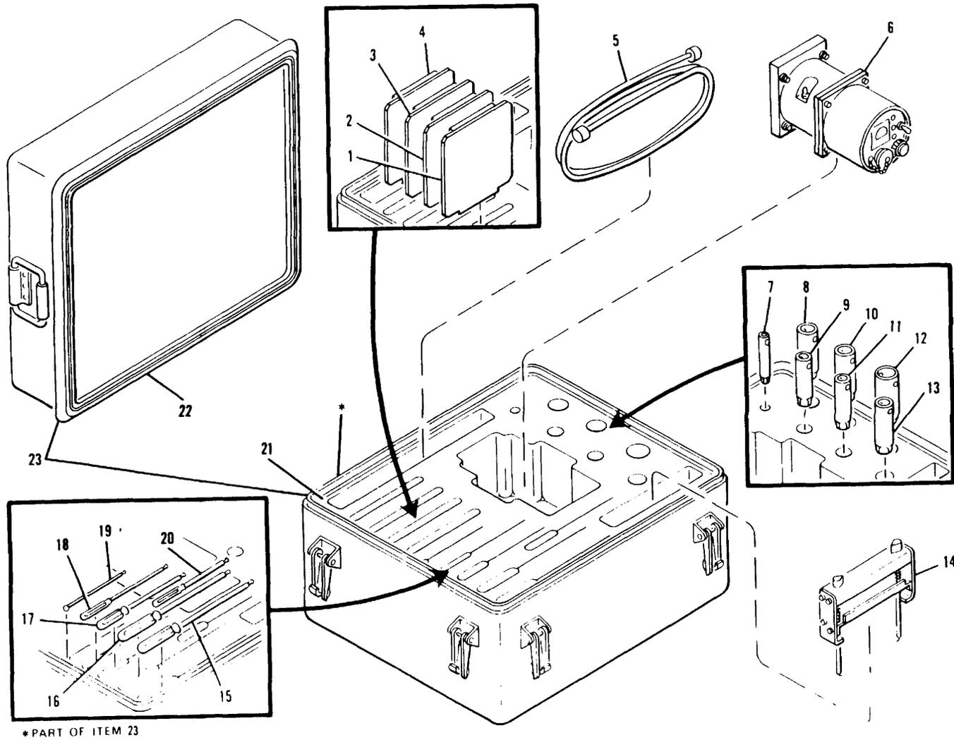
Figure 16. Common Special Tools and Test Equipment Carrying Case Assembly 10559658
