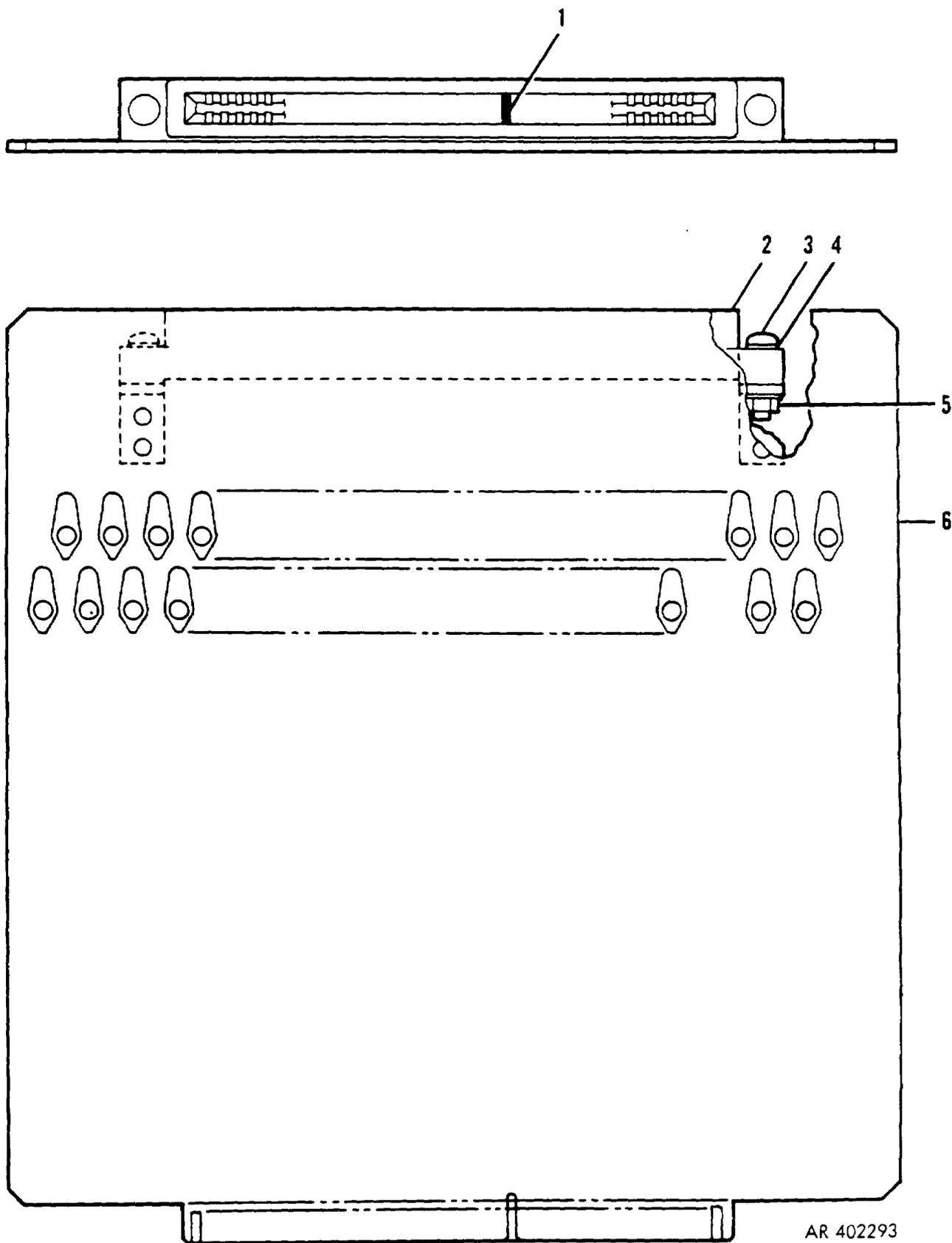
Figure 18. Minus 1600V Power Supply Extender Card Assembly-10559517
