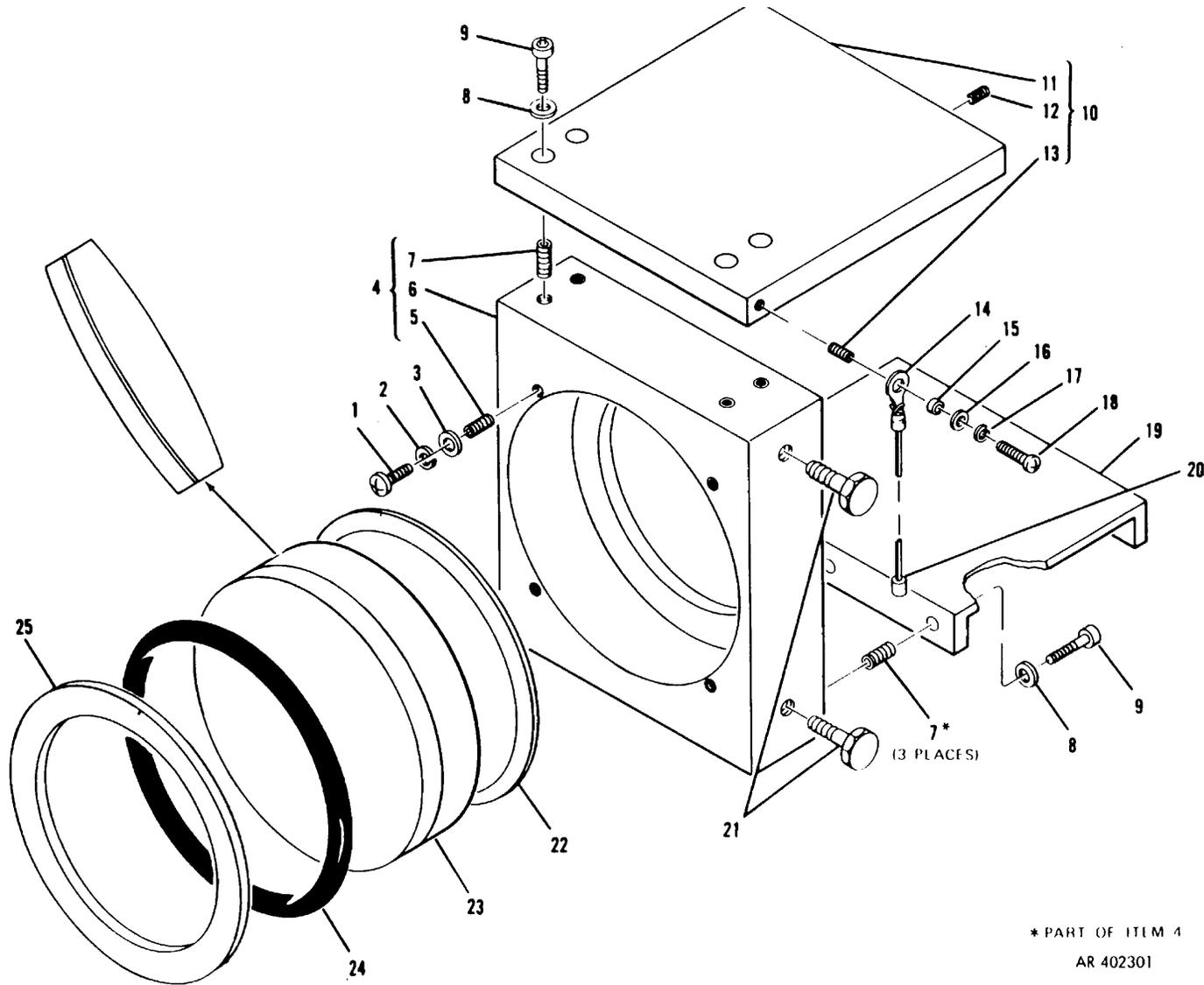
Figure 26. Alignment Lens Assembly 11741599
