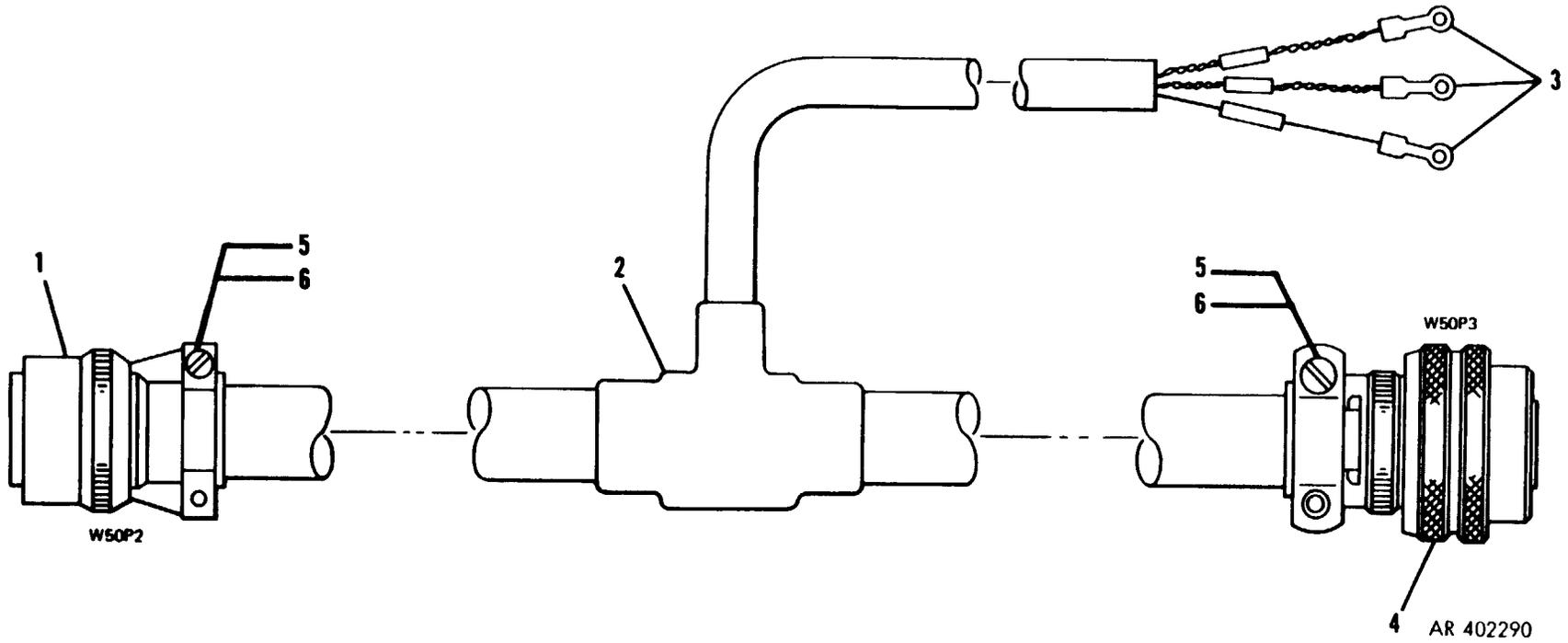
Figure 14. Test Cable Assembly-11737821
