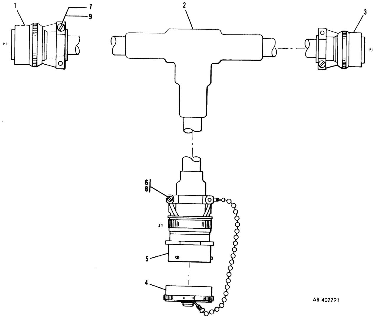
Figure 15. Pulse Forming Network Charge Meter Assembly 11745327
