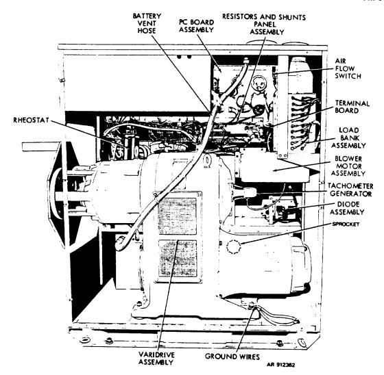
Figure 2-10. Test stand rear view showing components.
