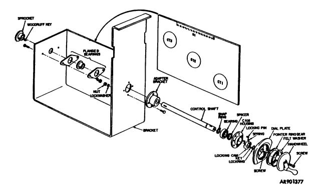
Figure 3-1. Speed control components and current transformers, exploded view.
