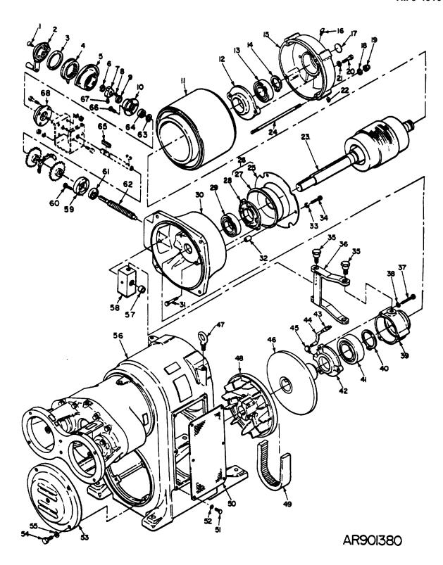
Figure 3-5. Varidrive assembly, exploded view (sheet 1 of 2).
