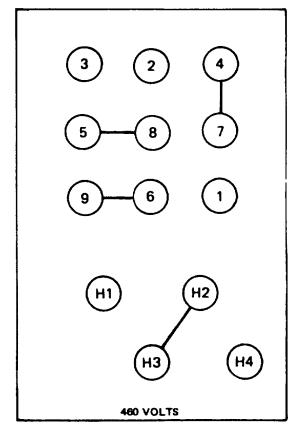
Figure 2-3. Link board assembly connections.
