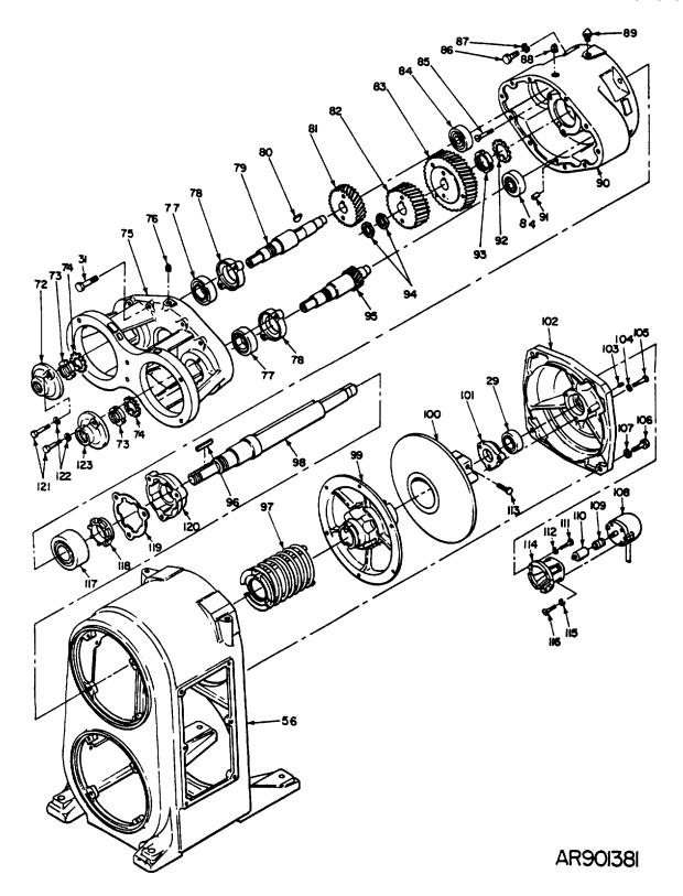
Figure 3-5. Varidrive assembly, exploded view (sheet 2 of 2).
