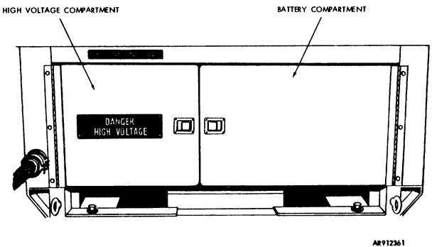
Figure 2-9. High voltage and battery components.
