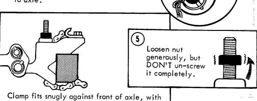
tension adjusting nut on TOP.
