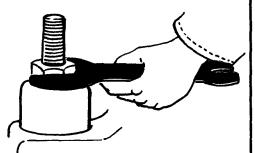
Make sure clamp and chain are firmly secured. A loose nut may allow them to work loose...
