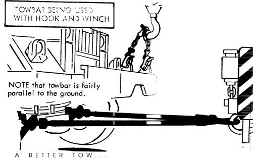
A set-up using both the TOWBAR and the WINCH offers **24** better maneuverability.
