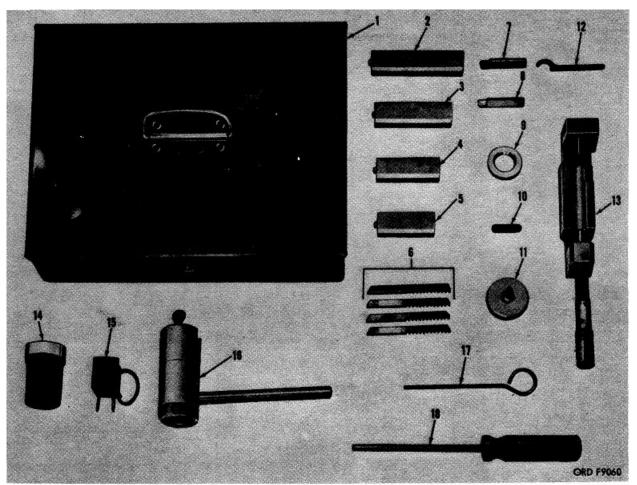
Figure 1. Tools and equipment for engine cylinder boring machine.
