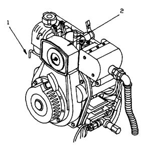
Figure 2-8. Engine Shutoff Screw Cock.
