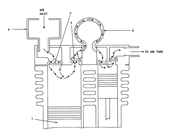
Figure 14. Air Compressor Pump Schematic.
