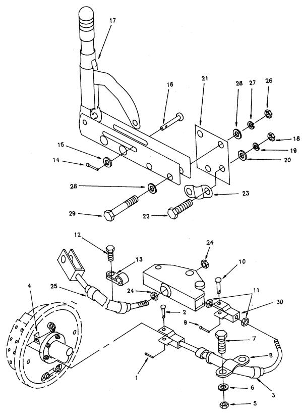
Figure 4-31. Parking Brake Assembly.
