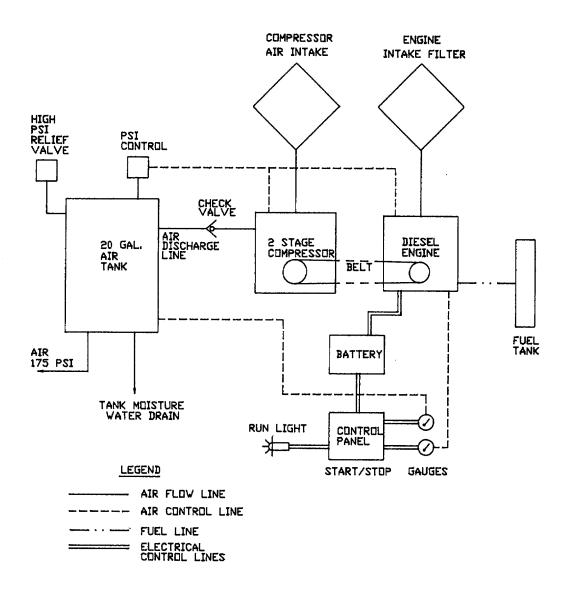
Figure 1-5. Compressor Flow Schematic.
