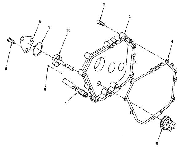
Figure 4-13. Rotary Pump and Diesel Engine Governor.
