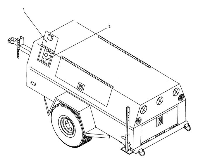
Figure 2-7. Frame Control Panel Location.
