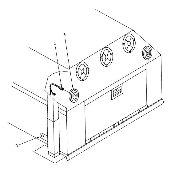
Figure 4-16. Vehicular Stop Light and Indicating Reflector.
