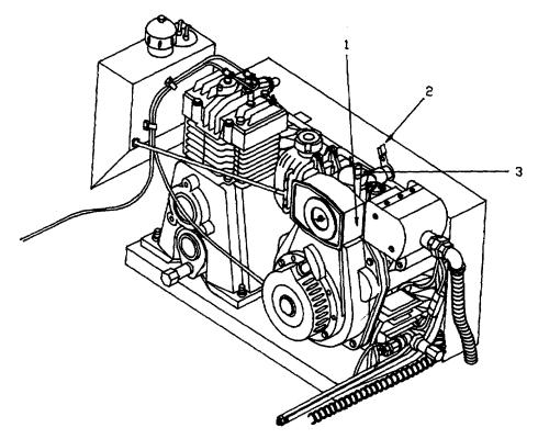
Figure 2-10. Engine Remote Control Lever.
