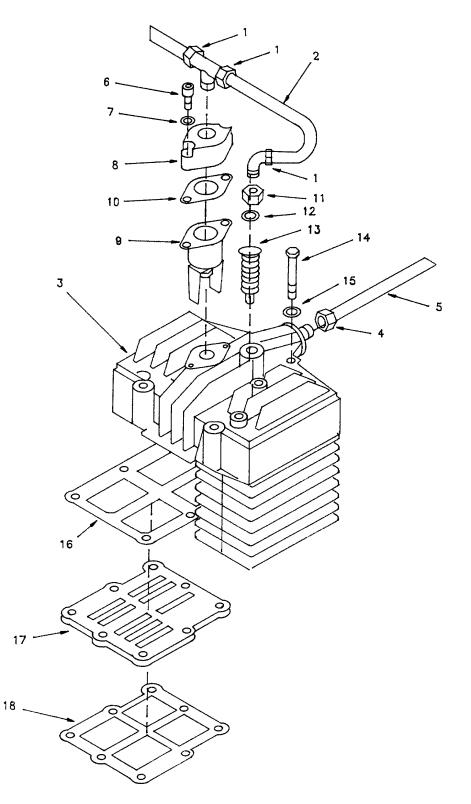
Figure 5-10. Compression Valve Plate and Unloaders.
