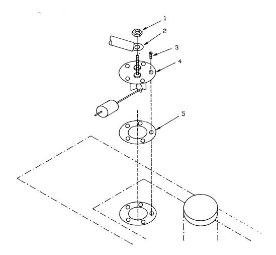
Figure 4-20. Liquid Level Switch.
