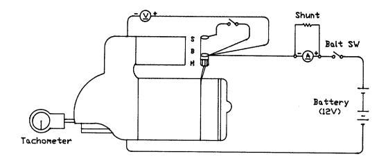
Figure 5-3. Engine Starter Motor Wire Diagram.
