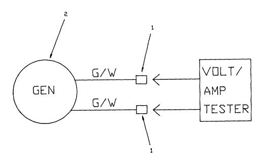
Figure 5-4. Generator Output Diagram.
