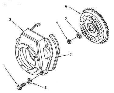
Figure 5-5. Cooling Fan Case and Flywheel.
