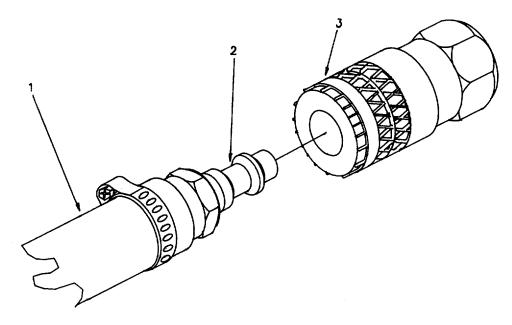
Figure 2-17. Hose Adaptors and Nonmetallic Hose.
