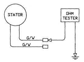
Figure 5-7. Stator Ground Test Diagram.
