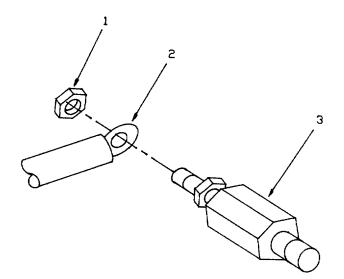
Figure 4-19. Temperature Transmitter.
