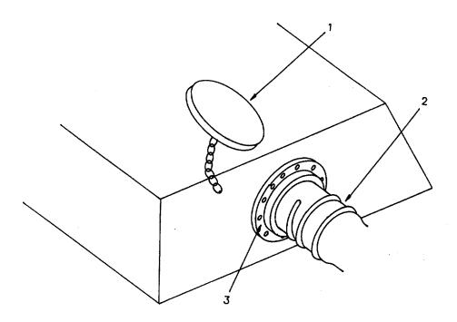
Figure 2-20. Heater Hose and Heater Inlet Adaptor.
