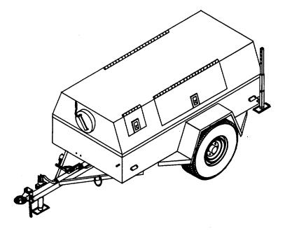
COMPRESSOR UNIT, RECIPROCATING 15 CFM, 175 PSI, DIESEL ENGINE DRIVEN, TRAILER MOUNTED MODEL CUE57-6DY-TM NSN: 4310-01-364-4316
