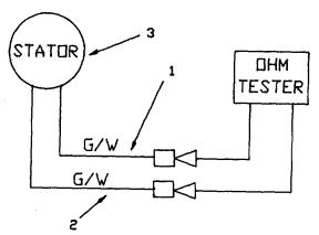
Figure 5-64. Stator Continuity Diagram.
