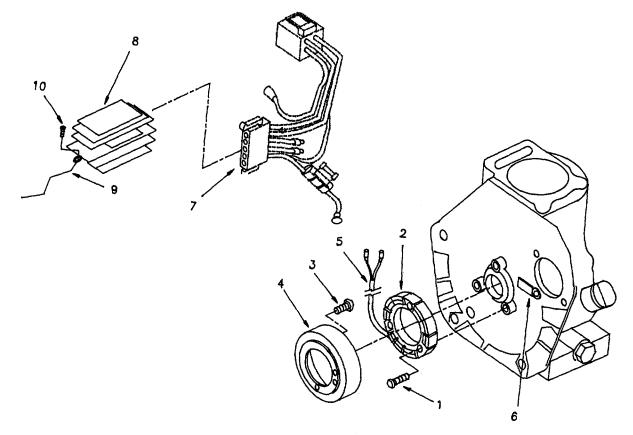
Figure 5-8. Engine Generator and Current Limiter.
