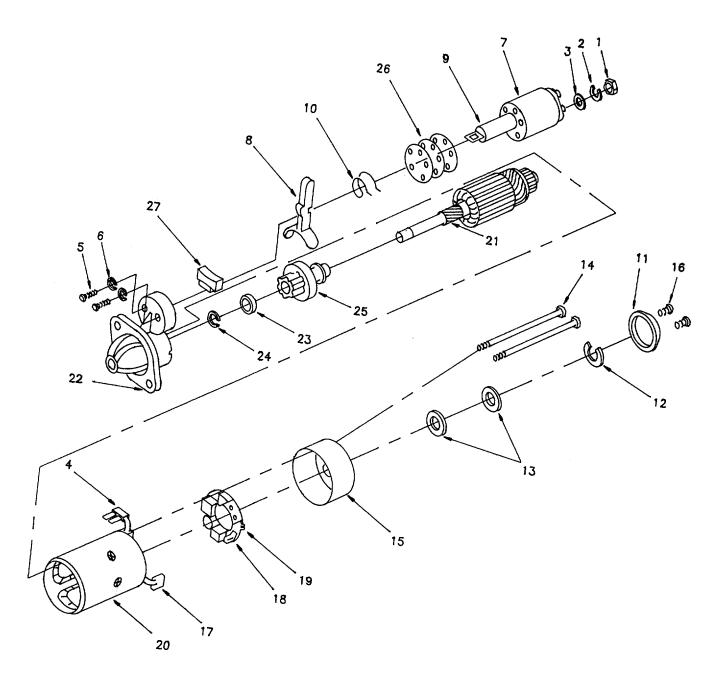
Figure 5-1. Engine Starter Motor.
