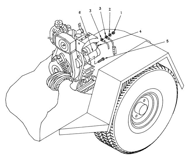
Figure 4-7. Engine Starter Motor.
