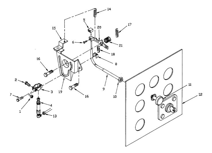
Figure 4-21. Knob, Cable Assembly, and Speed Control.
