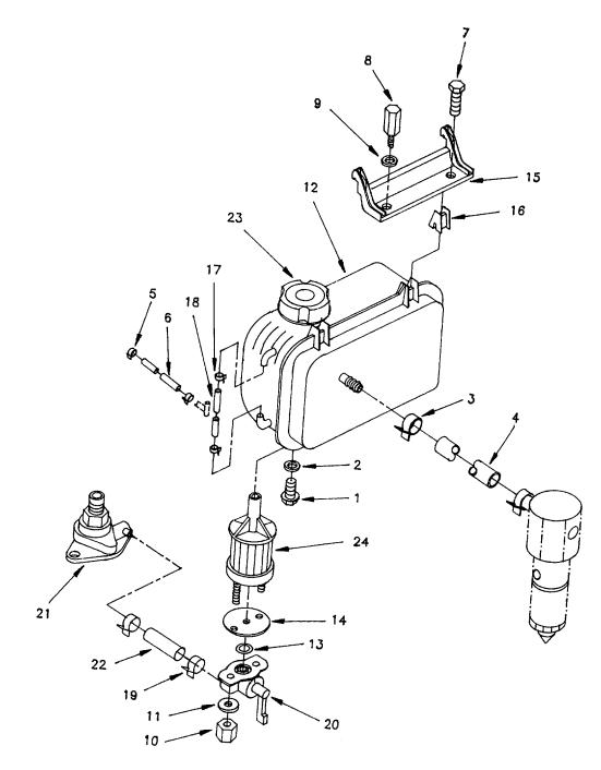
Figure 4-10. Fuel Tank Assembly.
