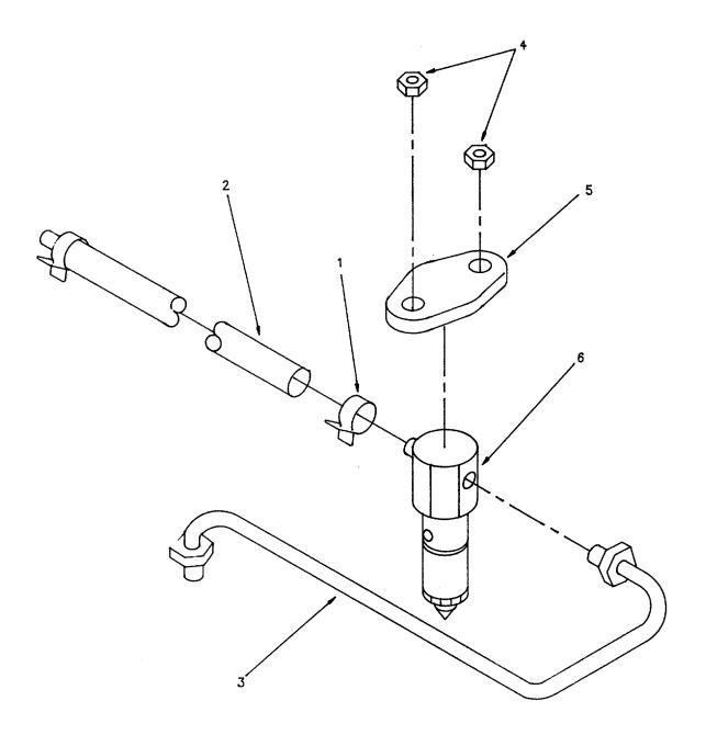
Figure 4-11. Fuel Injector Assembly.
