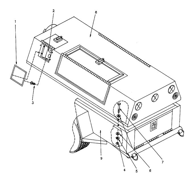
Figure 4-1. Complete Top Hood Assembly Removed.
