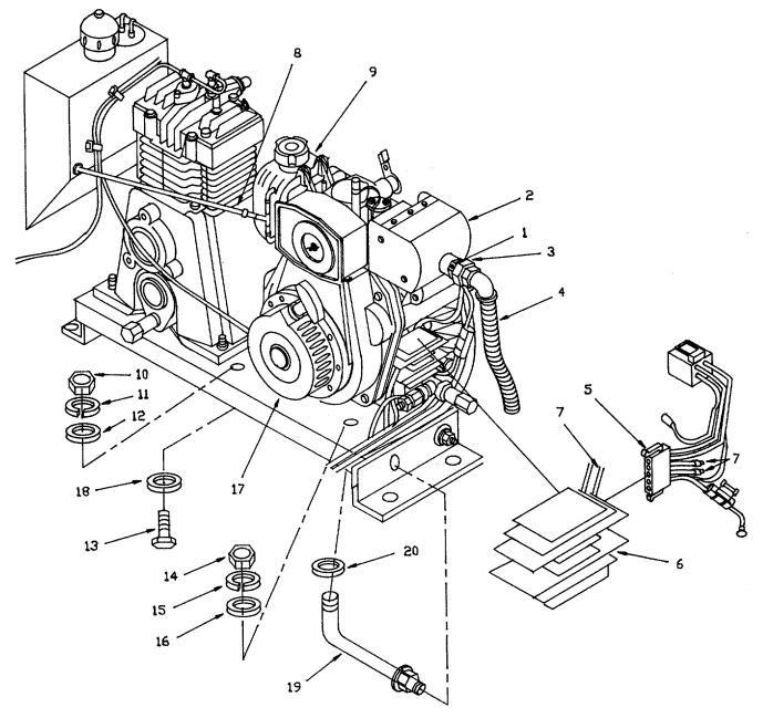
Figure 4-4. Engine Assembly.
