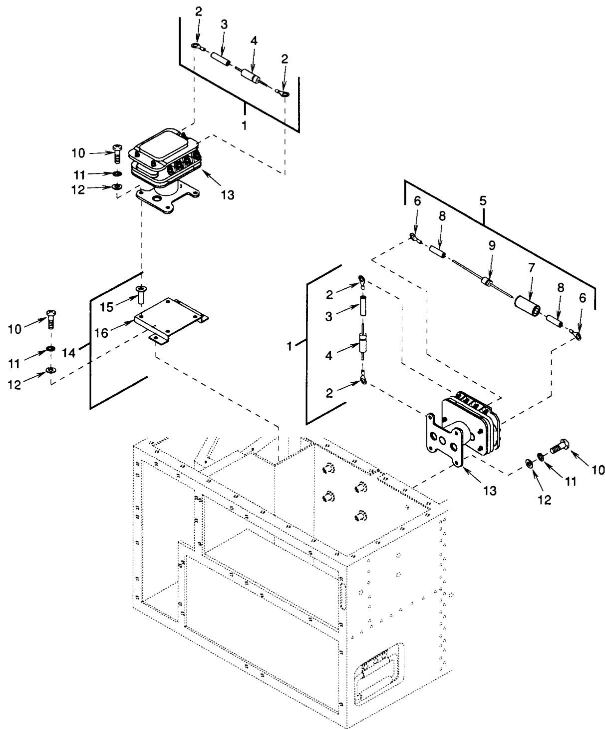
**Figure 14. Relays and Diodes**
