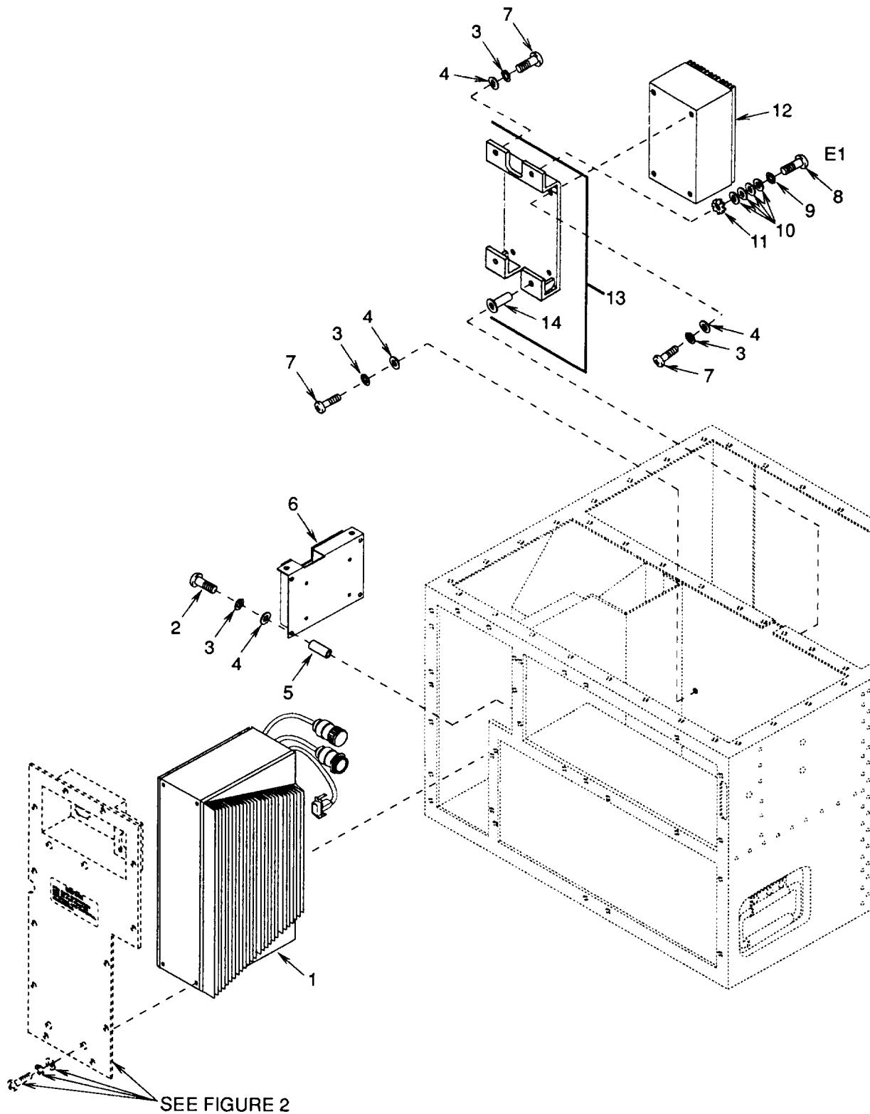
Figure 8. Motor Controller, Logic Box, and EMI Filter
