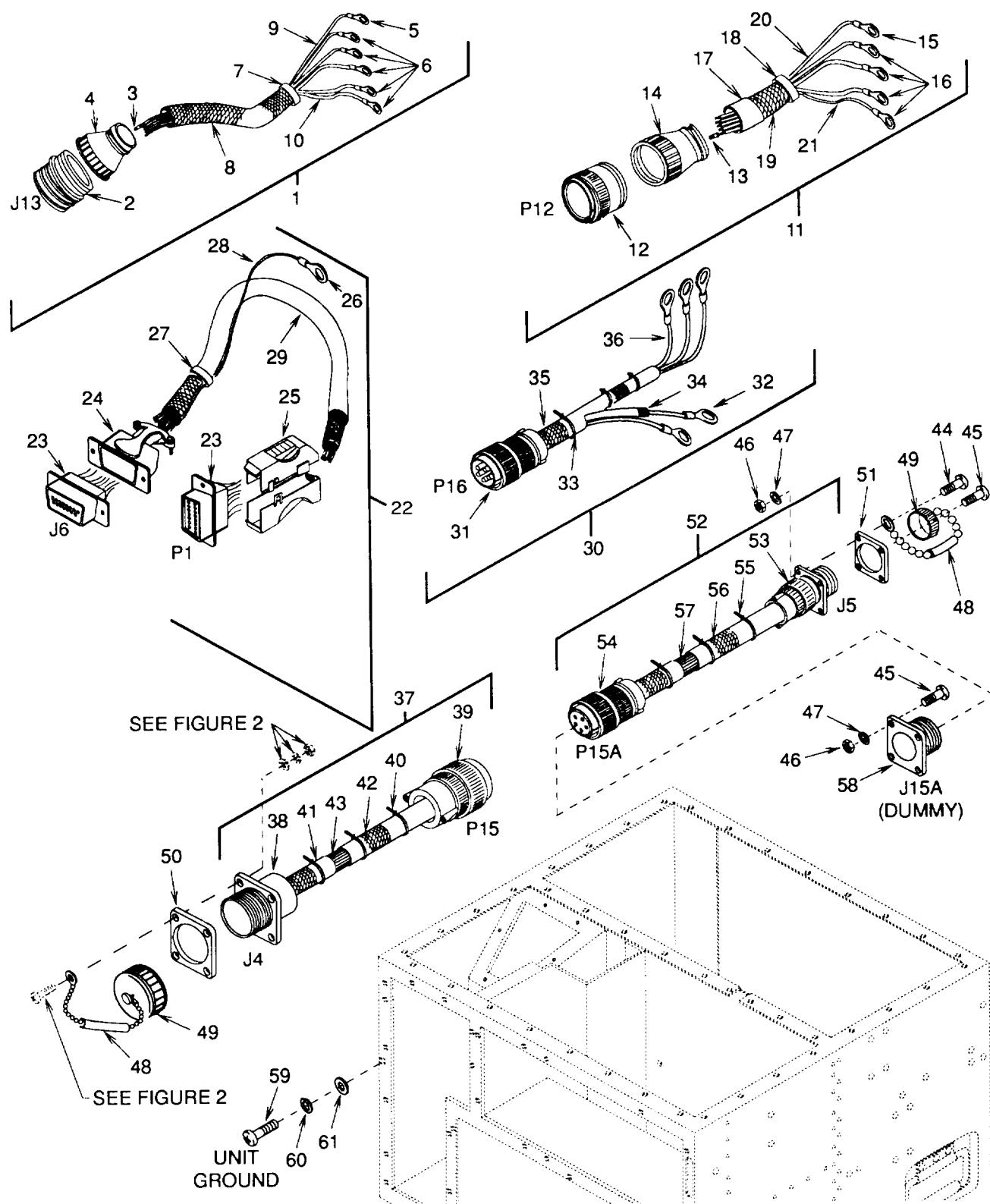
Figure 9. Wiring Harnesses
