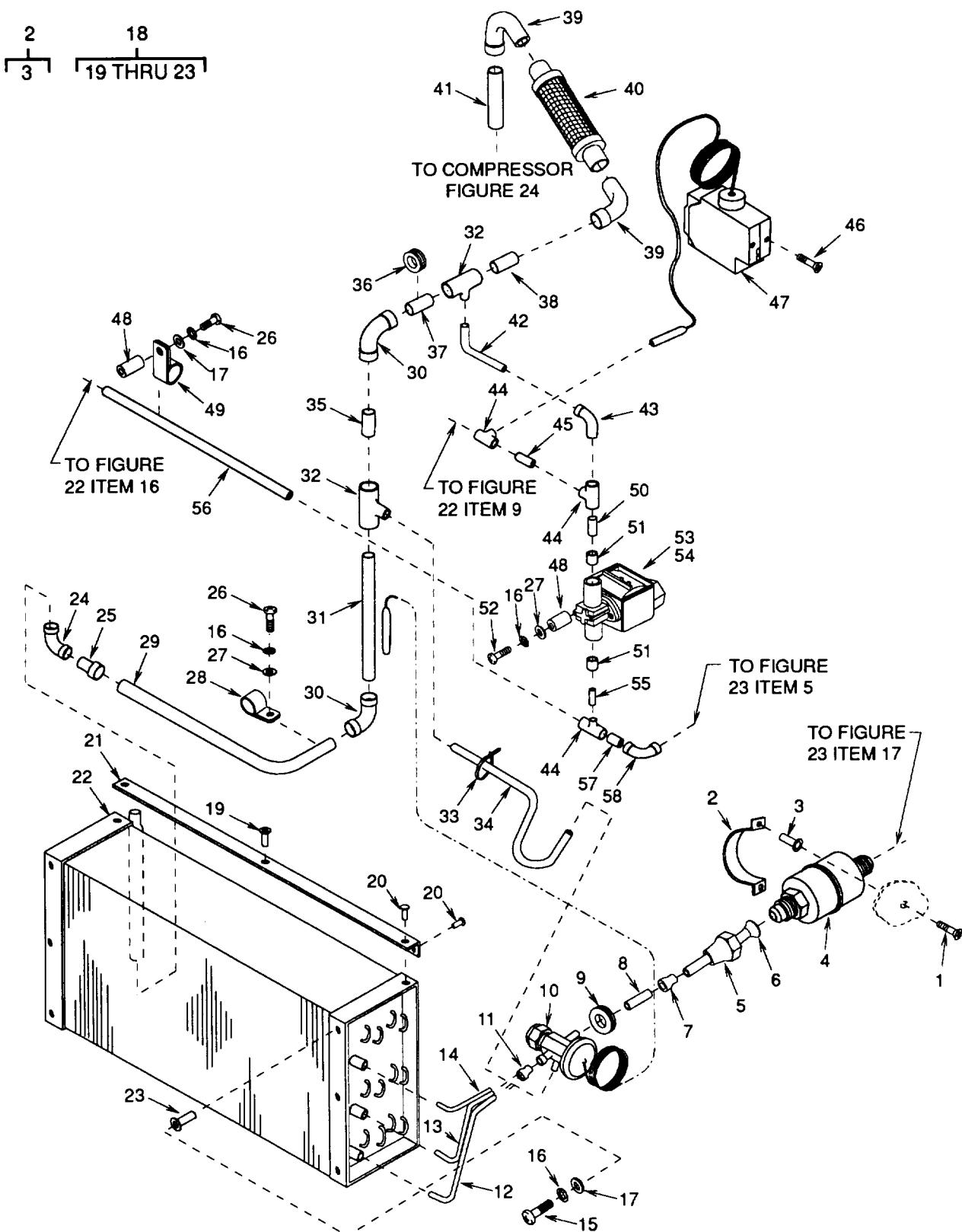
Figure 21. Evaporator Coil and Piping
