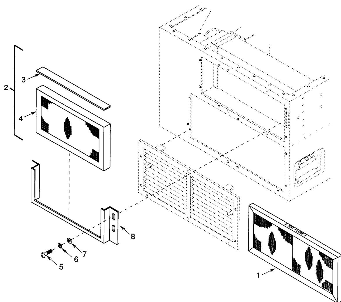
Figure 4. Filter and Mist Eliminator
