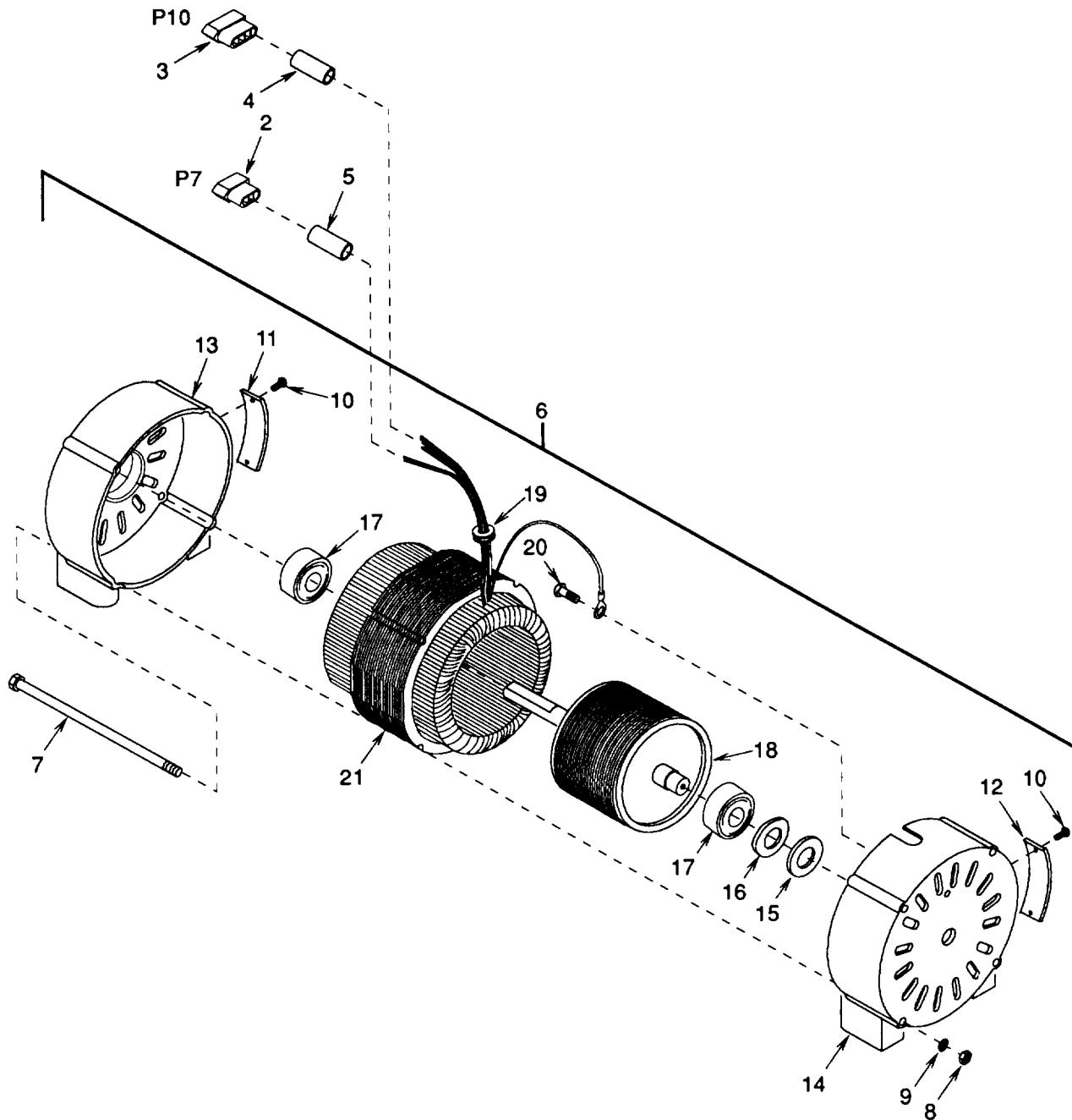
Figure 20. Motor Assembly, Condenser Fan
