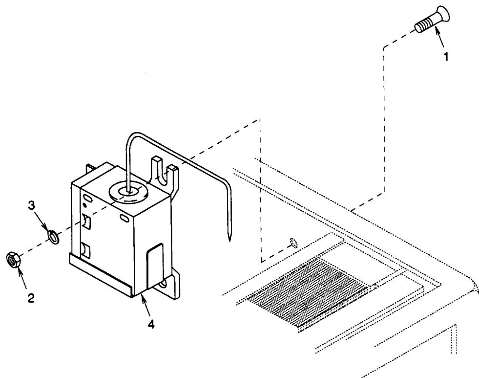
Figure 12. Coil Frost Switch
