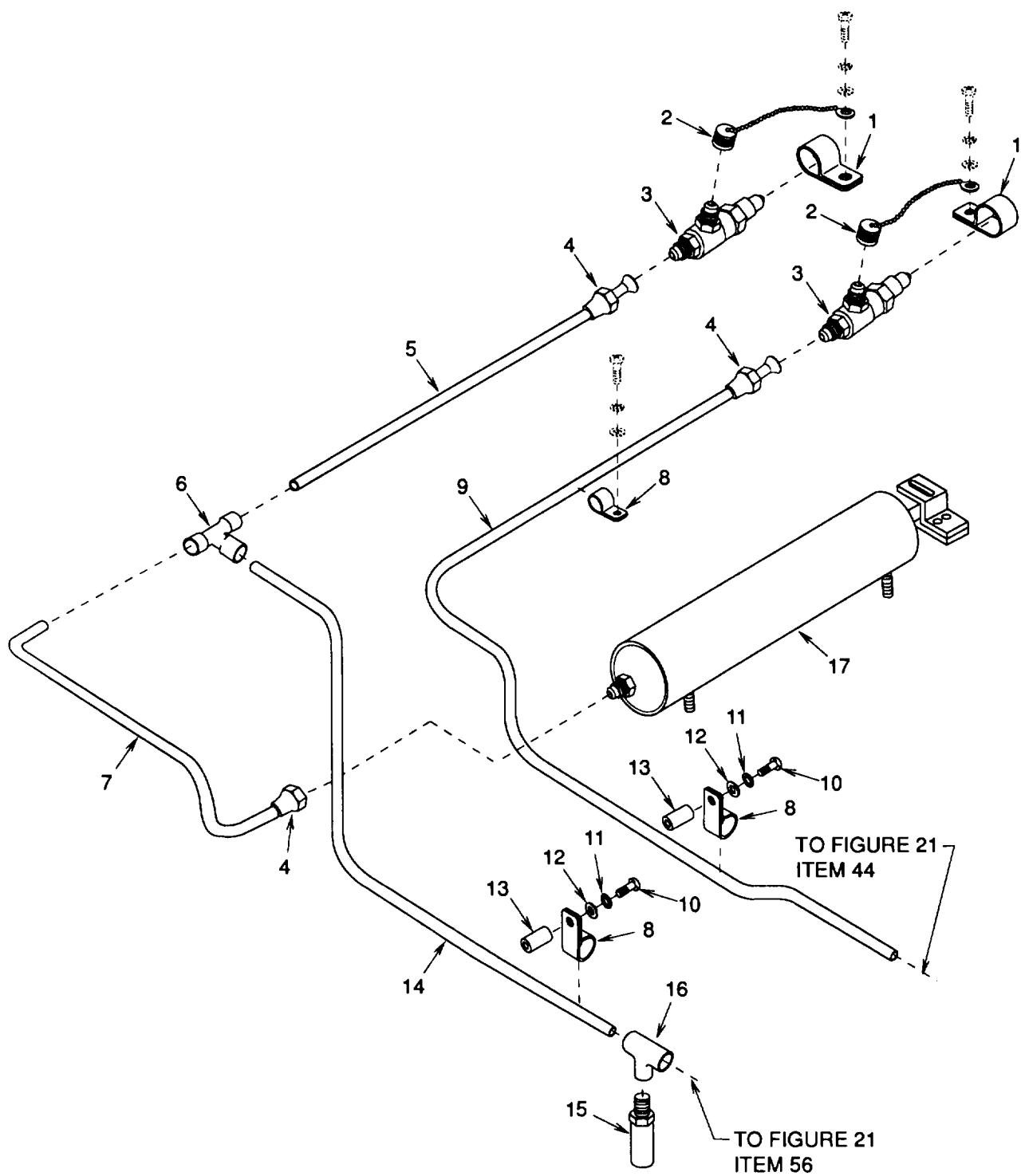
Figure 22. Charging Valves, Relief Valve, and Actuating Cylinder
