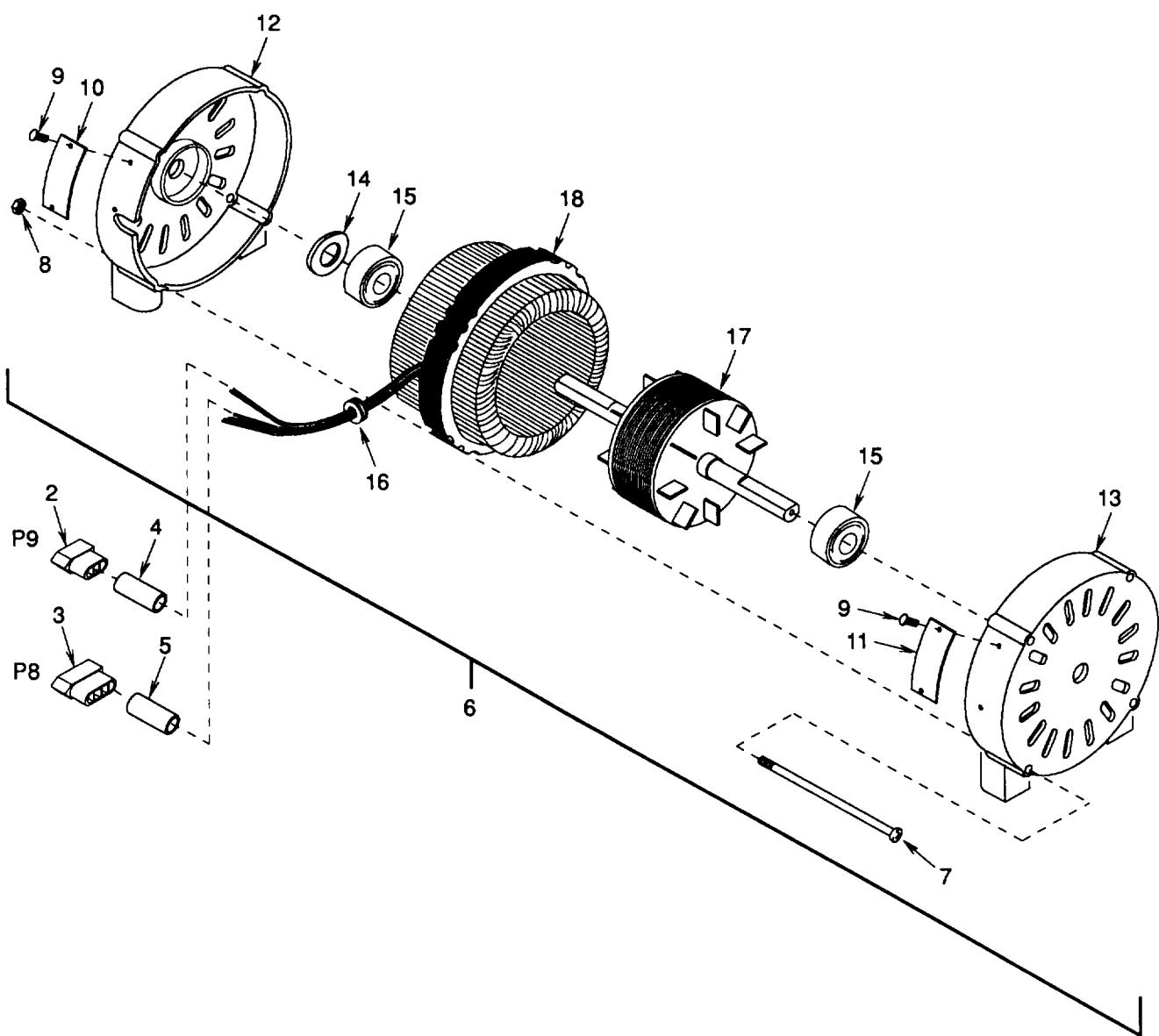
Figure 17. Motor Assembly, Evaporator Fan
