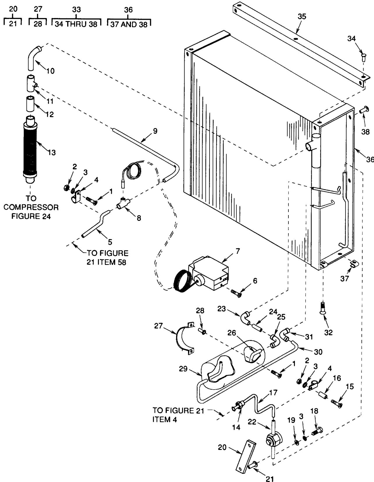
Figure 23. Condenser Coil and Piping
