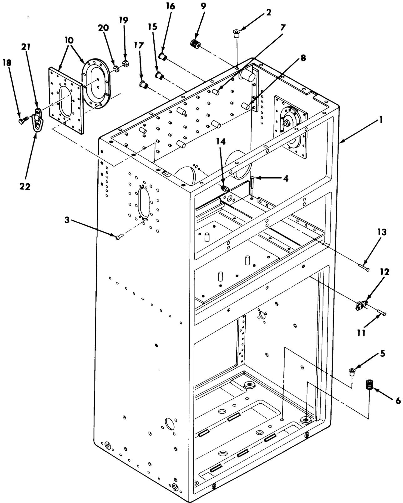
Figure 23 Casing Hardware
