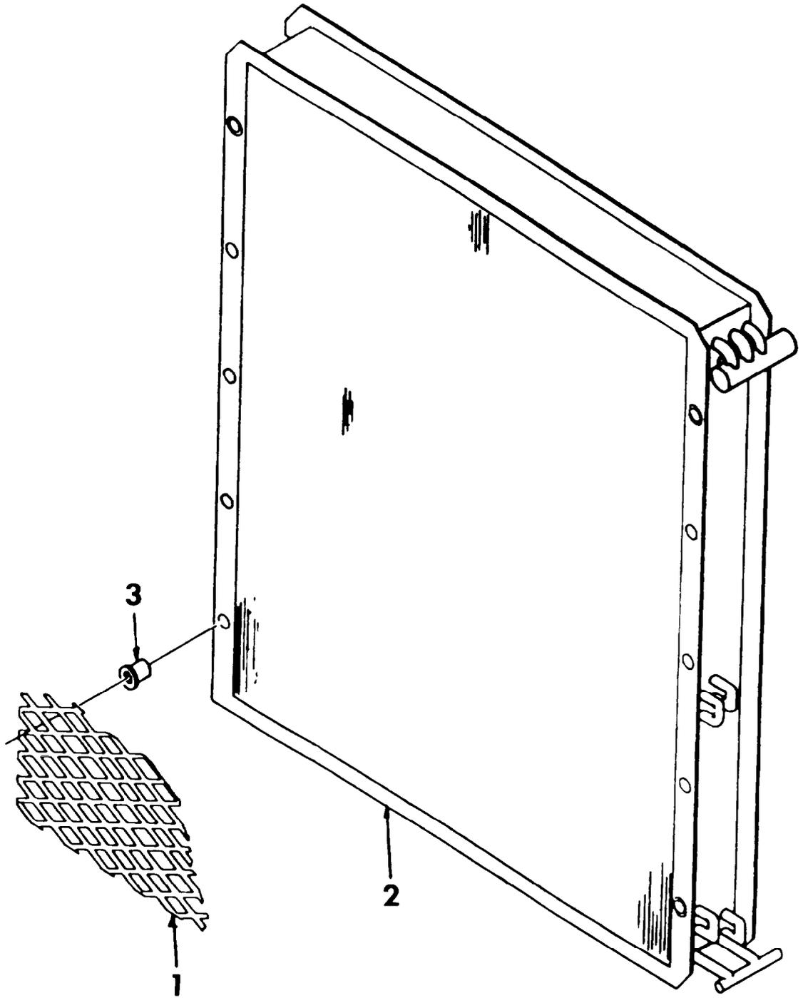
Figure 22 Condenser Coil and Guard
