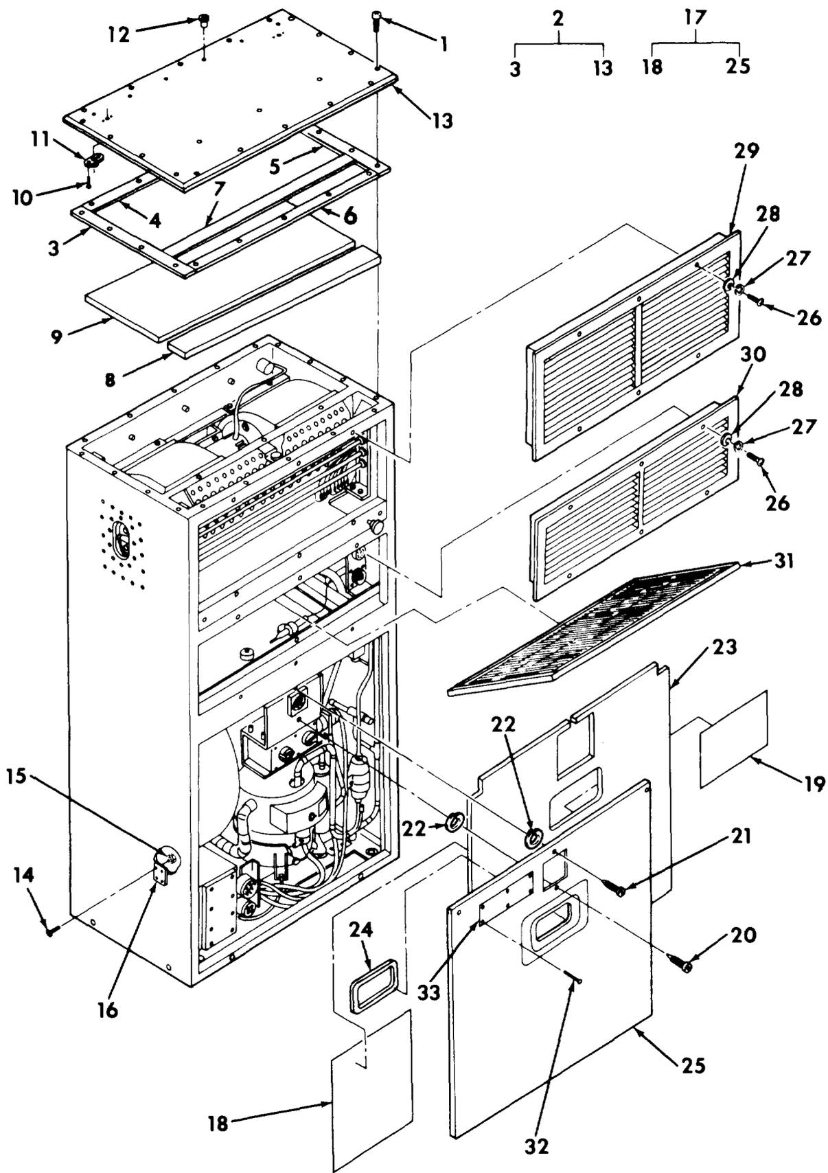
Figure 2 Top, Front and Left Side Outside Panels
