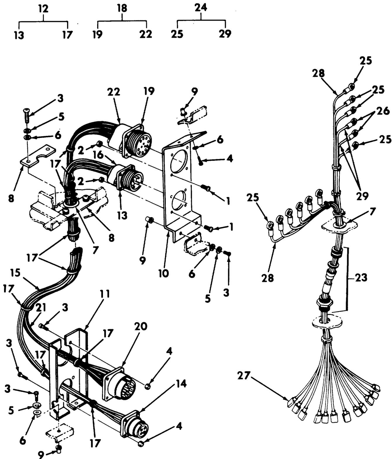
Figure 11 Auxiliary and Terminal Boards Wiring Harnesses
