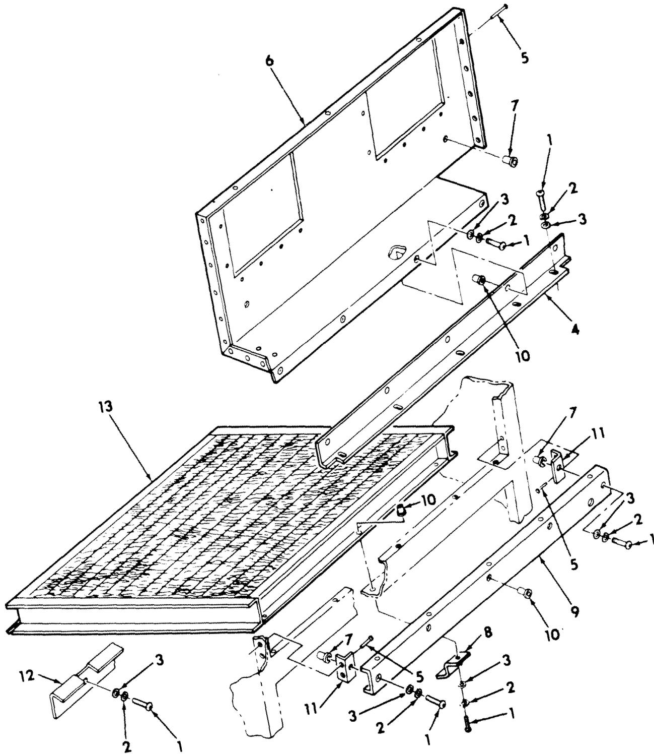
Figure 18 Evaporator Coil and Structure
