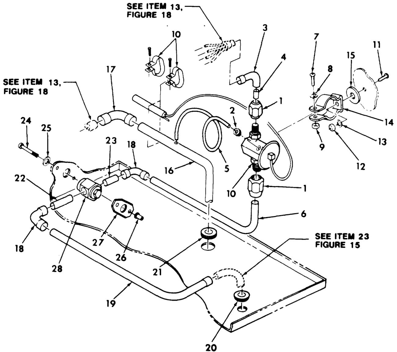
Figure 17 Expansion Valve and Sight Glass
