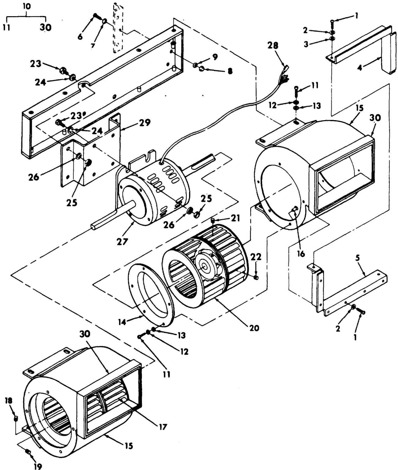
Figure 4 Evaporator Fan Assembly
