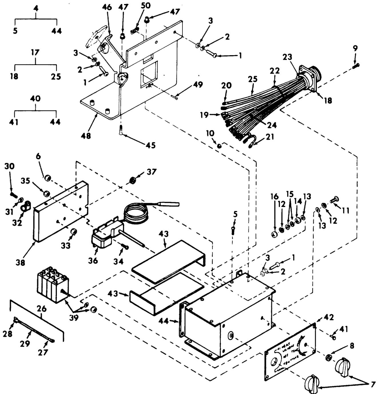
Figure 13 Control Panel Assembly
