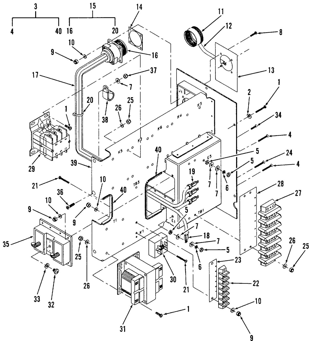
Figure 8. Junction Box Assembly (Sheet 1 of 2)
