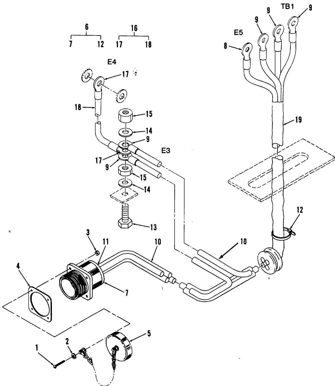
Figure 12. Auxiliary Power Connector Assembly
