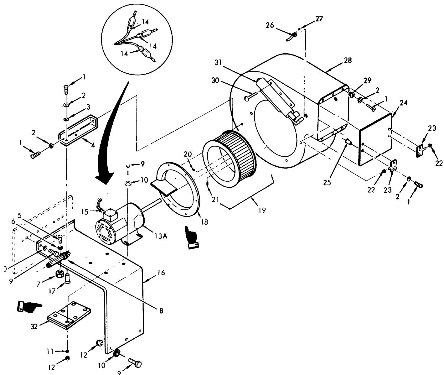
Figure 3. Condenser Fan Motor, Fan Scroll and Motor Support
