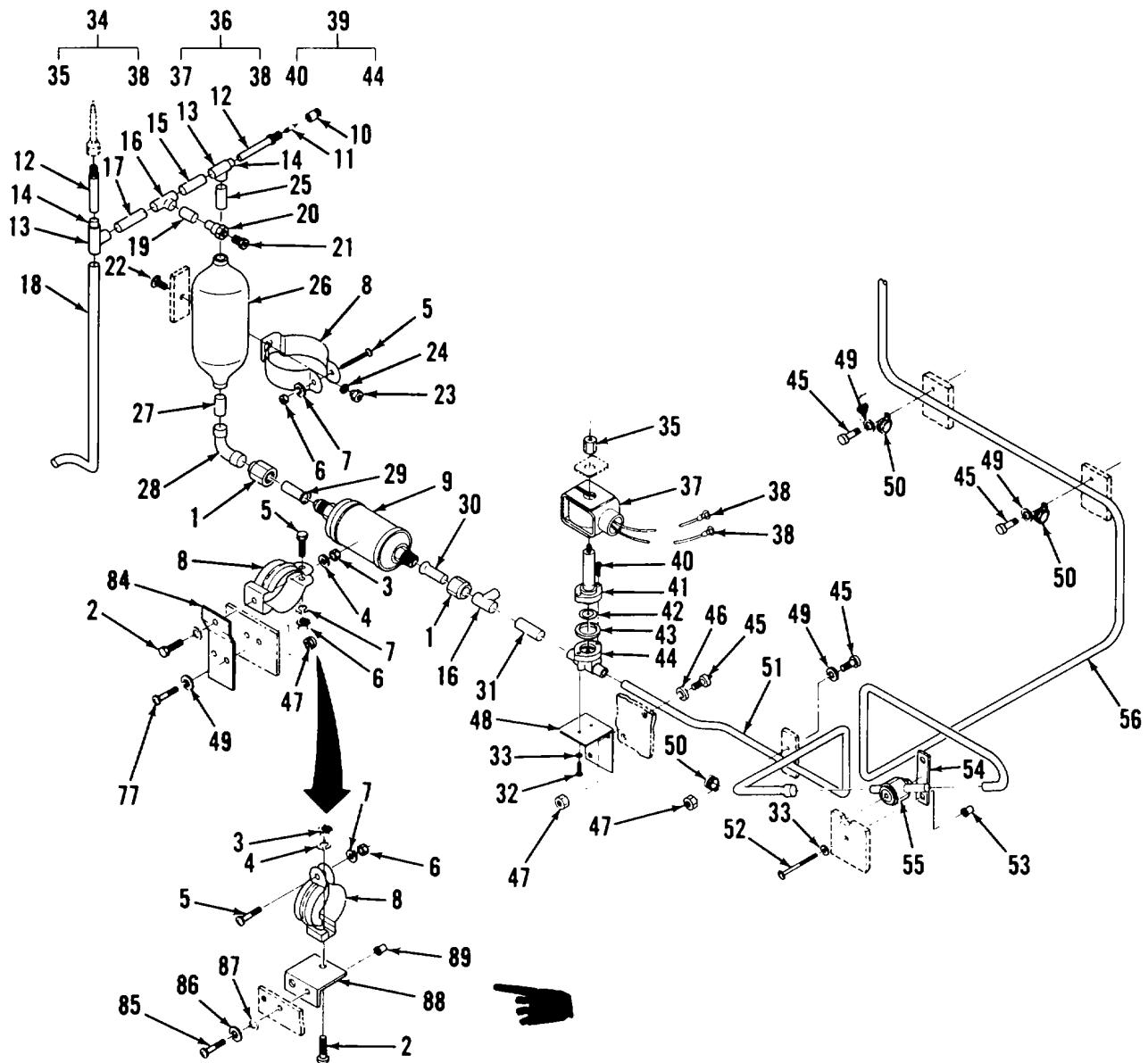
Figure 13. Refrigeration Valves and Related Tubing (Sheet 1 of 2)
