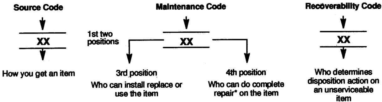
\* Complete Repair: Maintenance capacity, capability, and authority to perform all corrective maintenance tasks of the "Repair" function in a use/user environment in order to restore serviceability to a failed item.
