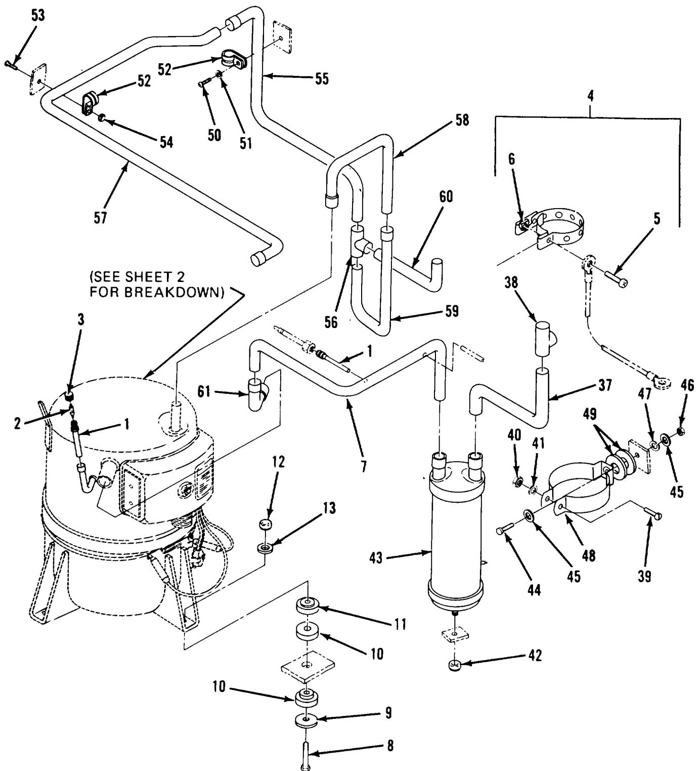
**Figure 16A.. Compressor, Accumulator and Related Tubing
