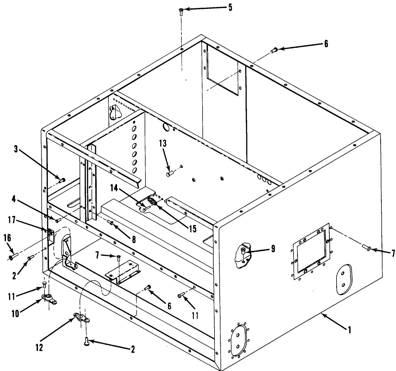
Figure 18. Casing, Hardware and Insulation (Sheet 1 of 2)
