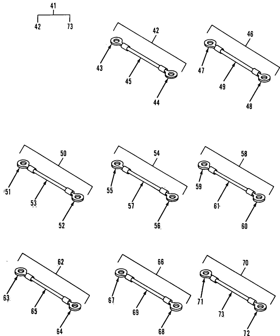
Figure 8. Junction Box Assembly (Sheet 2 of 2)
