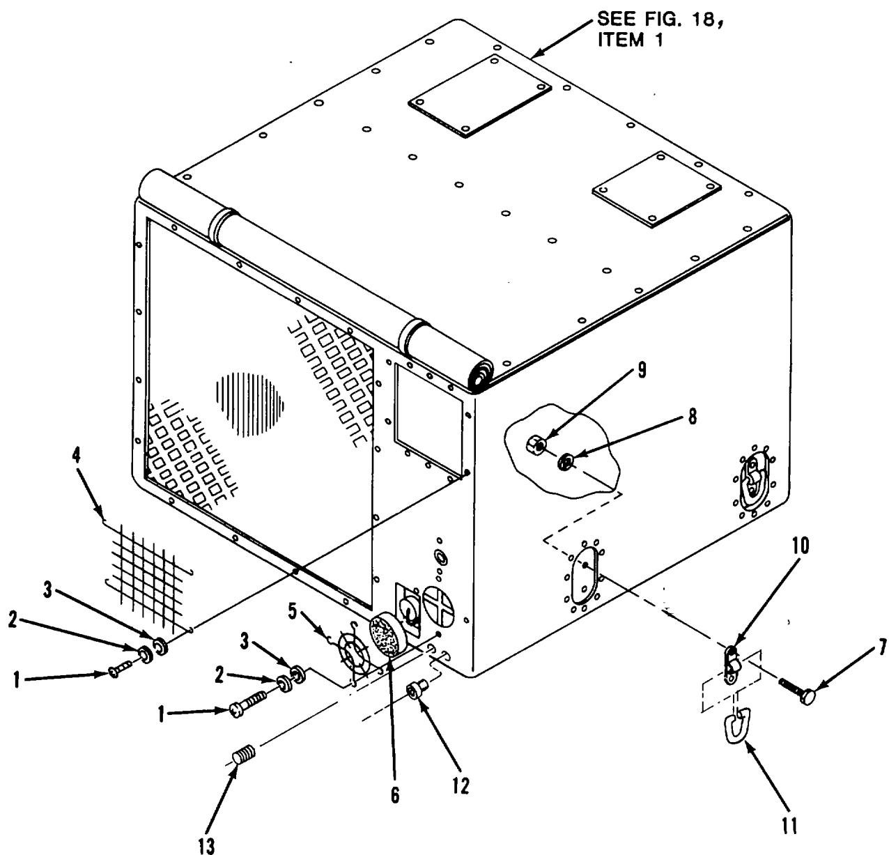
Figure 2. Rear Covers and Lifting Rings
