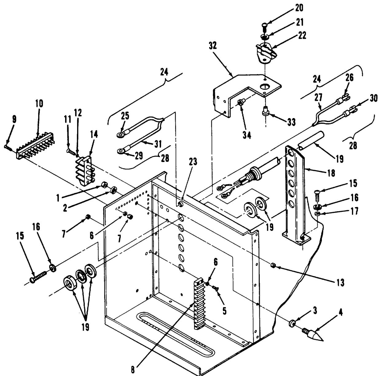
Figure 11. Terminal Boards, Heating Elements and Thermostatic Switch
