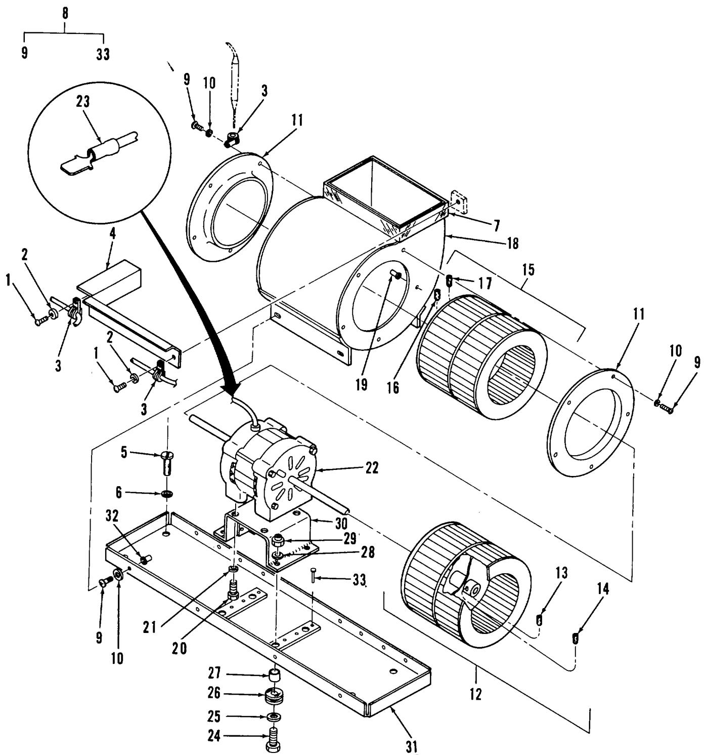
Figure 5. Evaporator Fan Assembly
