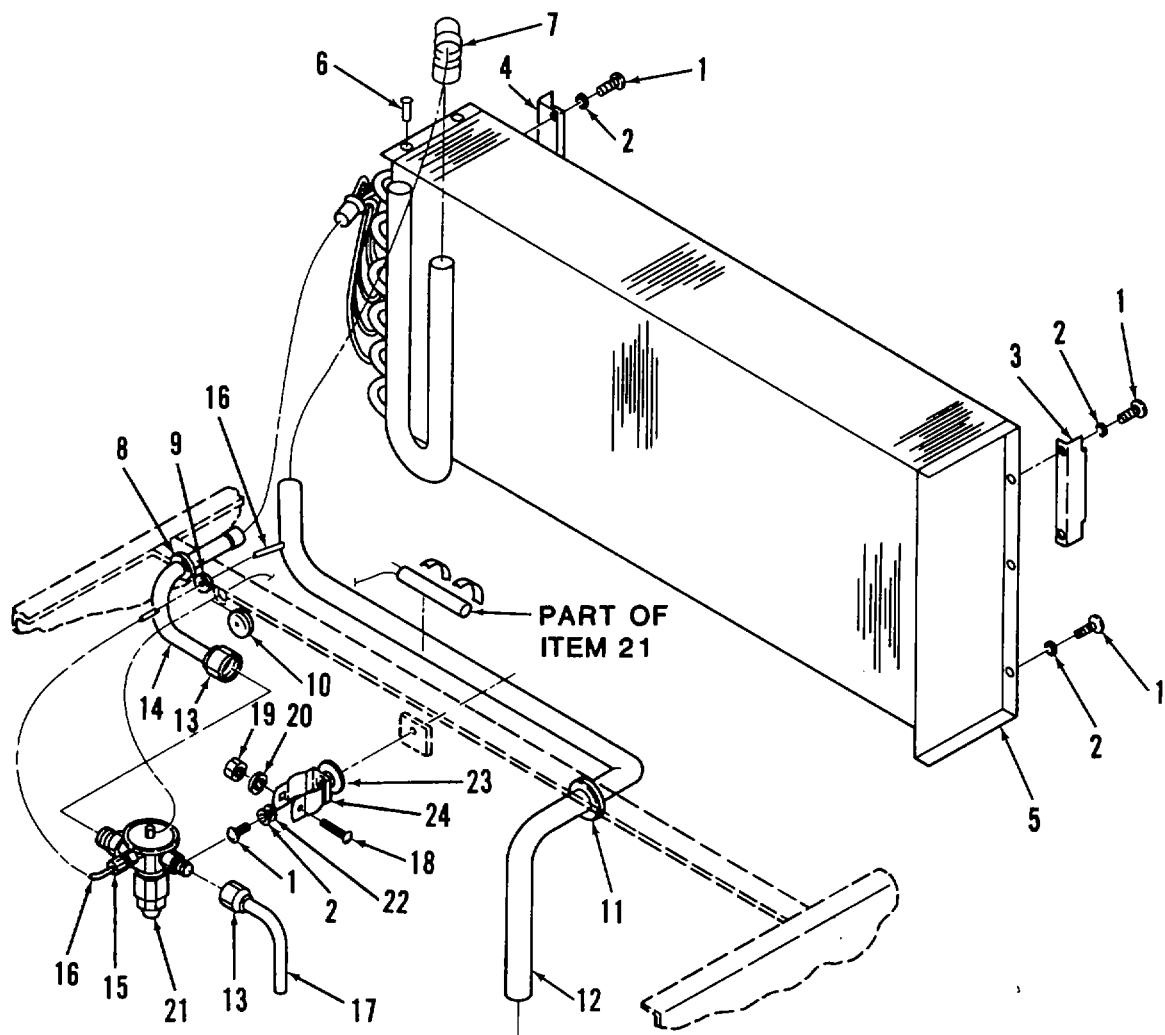
Figure 15. Evaporator Coil, Thermoexpansion Valve and Related Tubing
