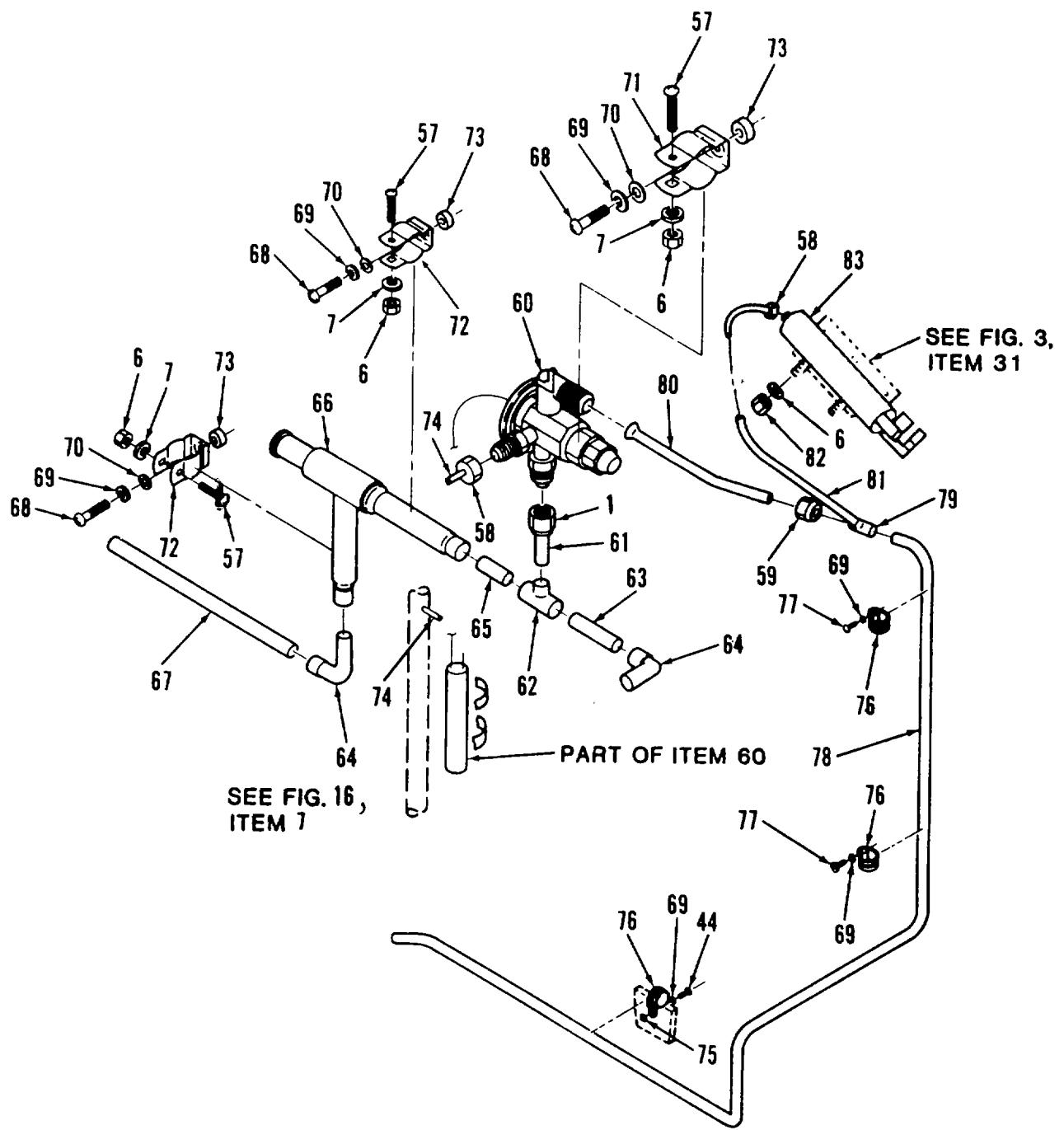
Figure 13. Refrigeration Valves and Related Tubing (Sheet 2 of 2)
