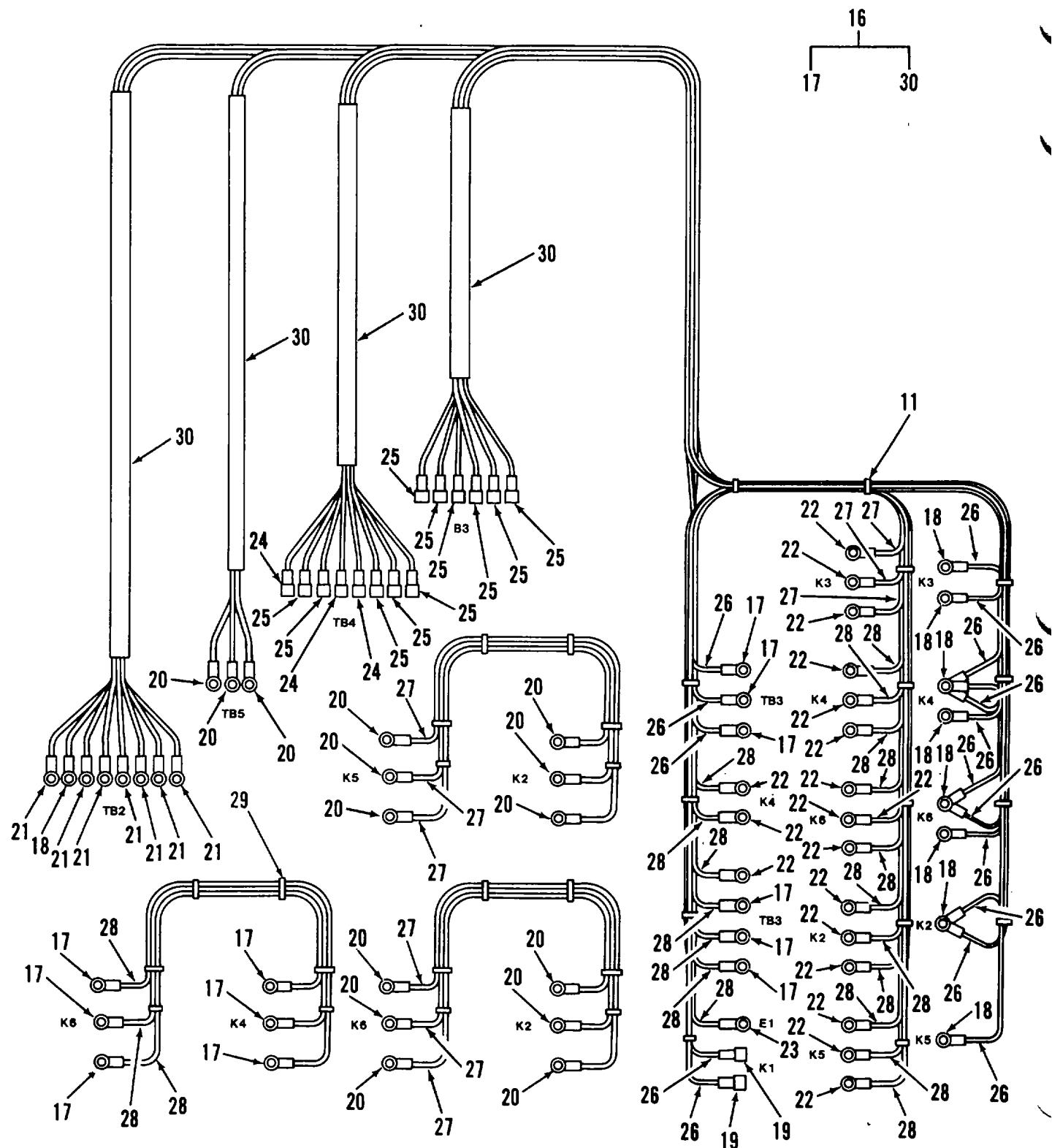
Figure 9. Junction Box Wiring Harness (Sheet 2 of 2)
