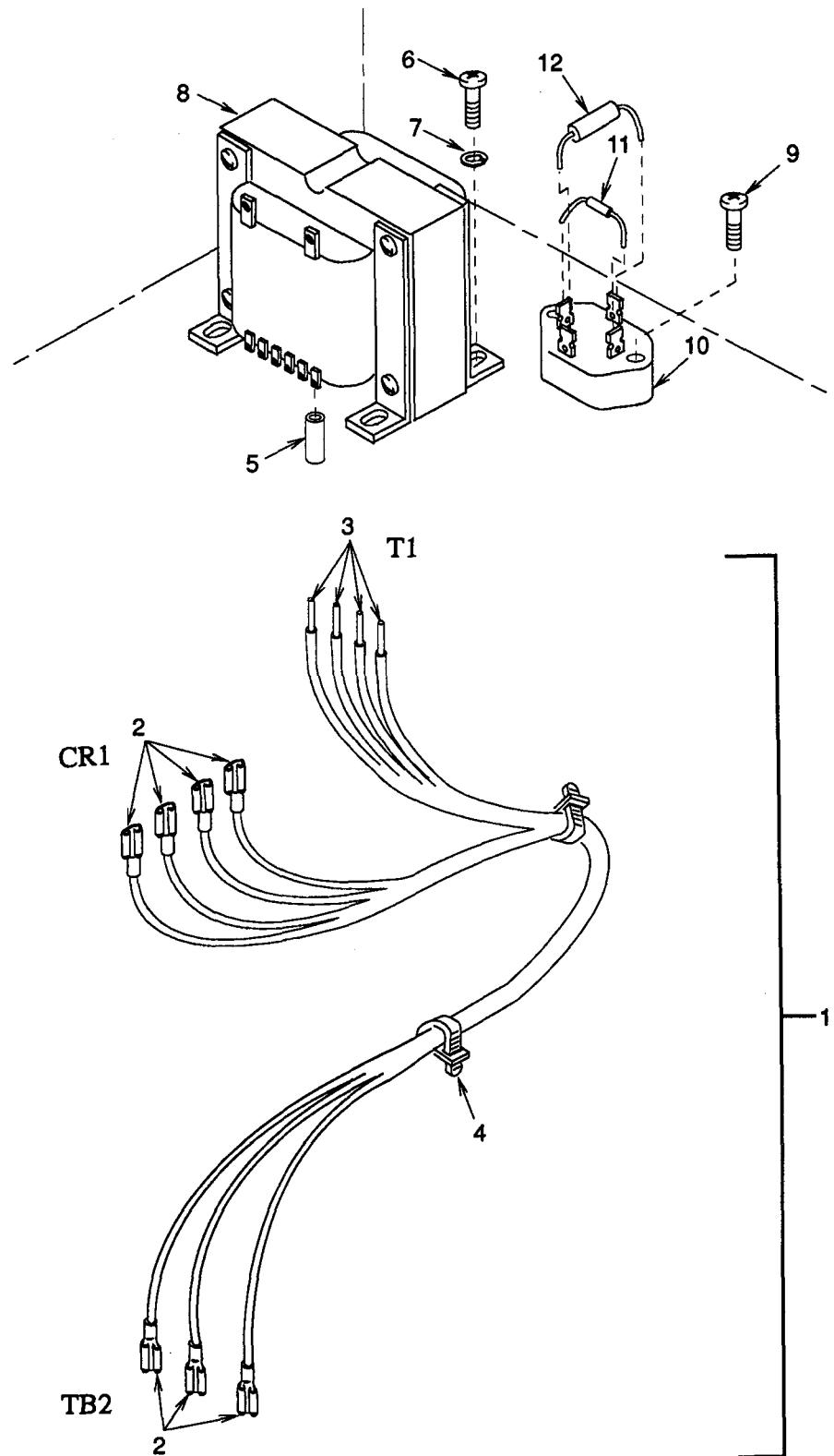
Figure 18 - Rectifier and Transformer Assembly
