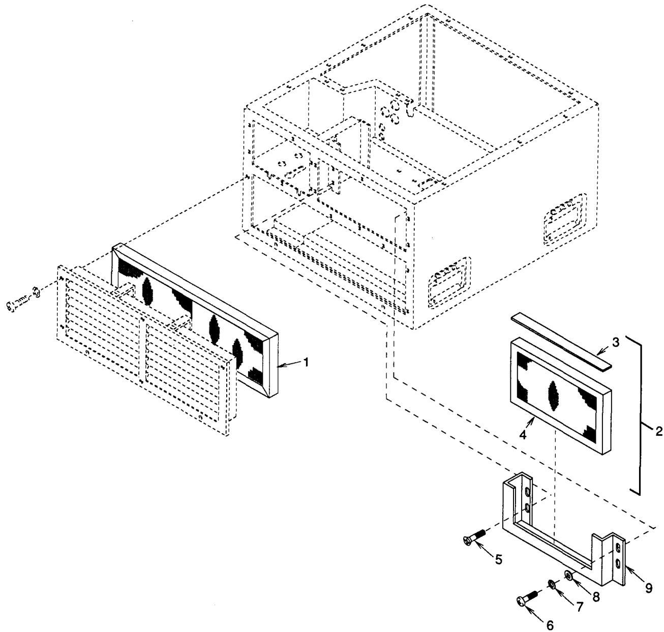
Figure 6. Air Filter and Mist Eliminator
