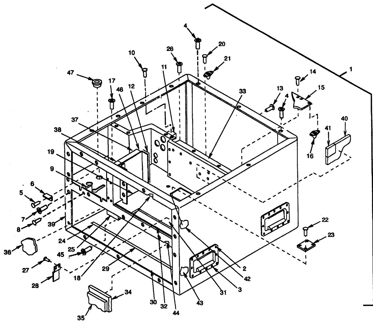
Figure 32. Housing Assembly.
