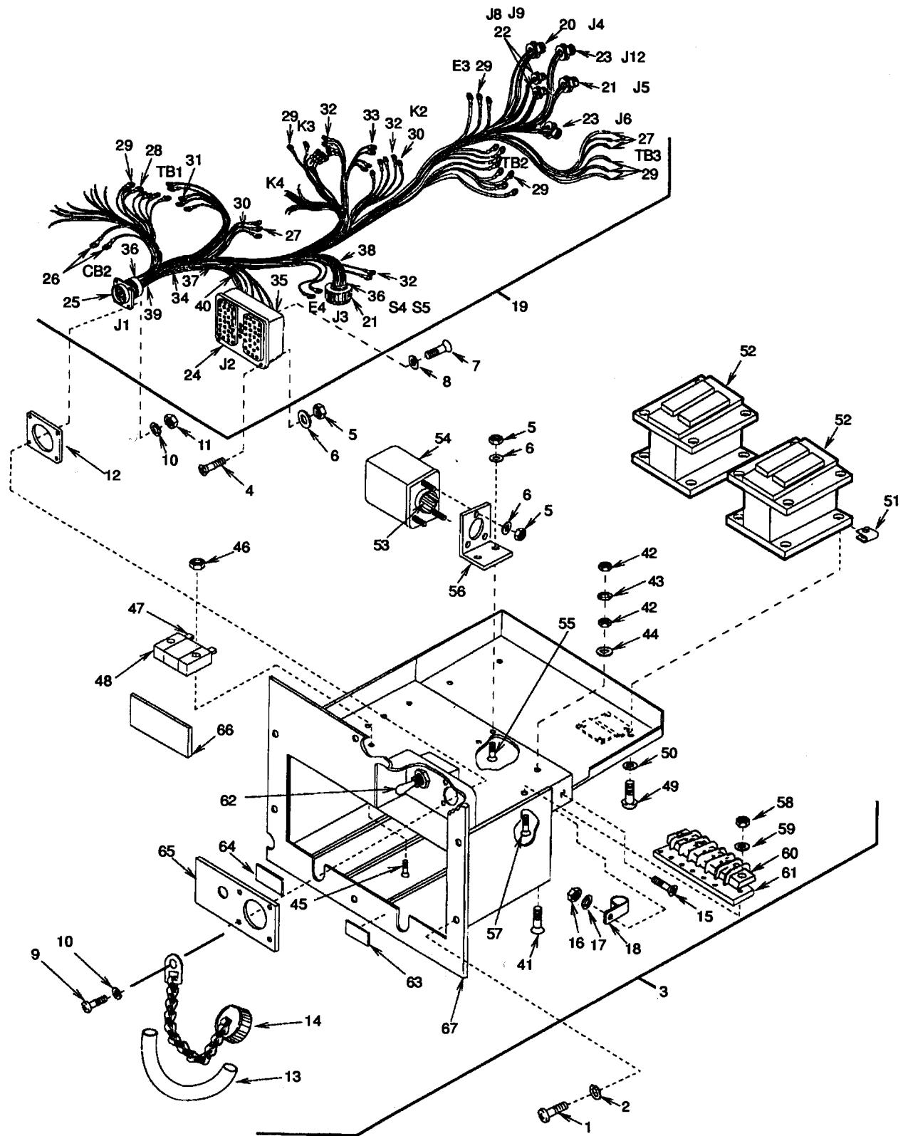
Figure 13. Junction Box and Wiring Harness (Model F9000H-1S).
