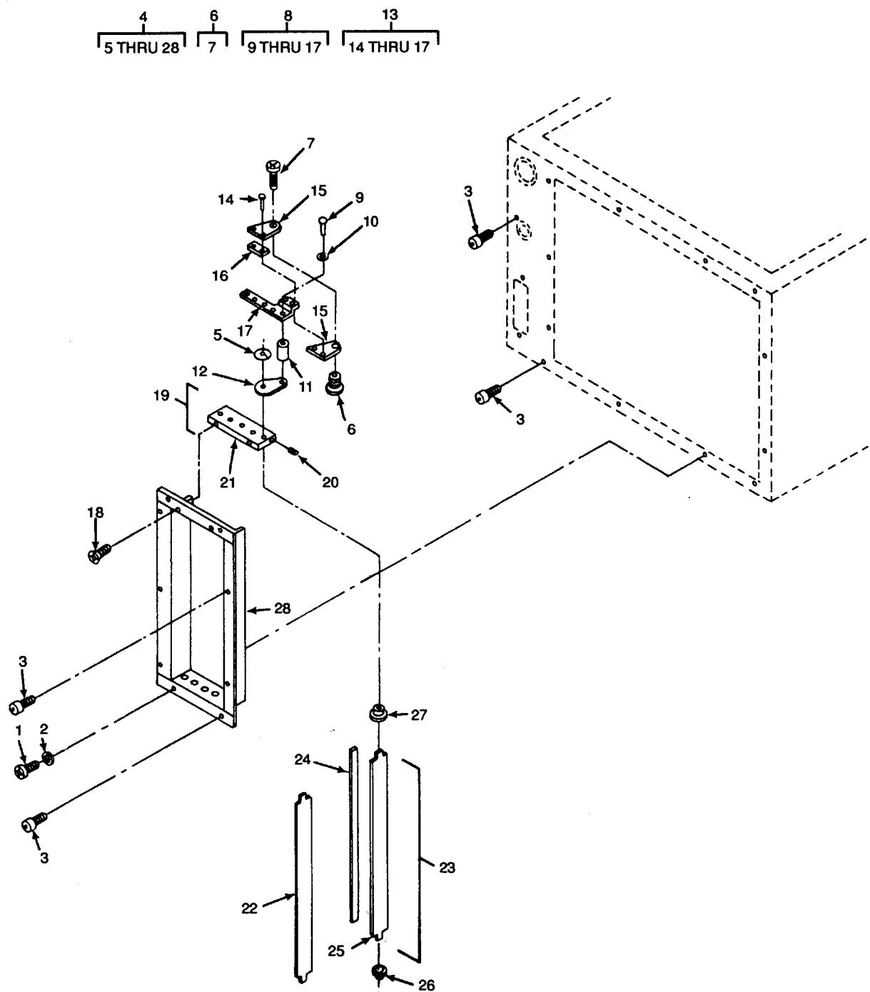
Figure 7. Condenser Air Discharge Louver and Linkage.
