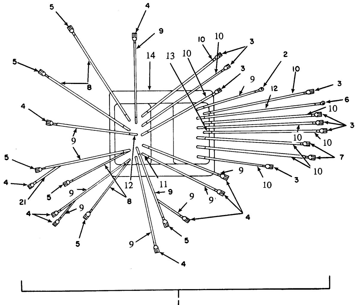
Figure 11 - Control Module Wiring Harness
