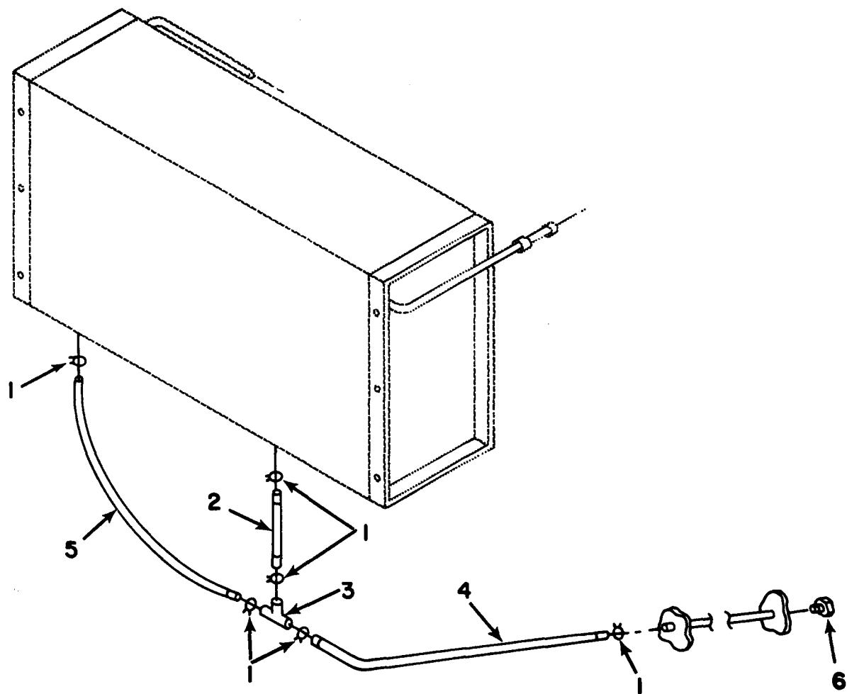
**Figure 9 - Condensate Drain Tubes**
