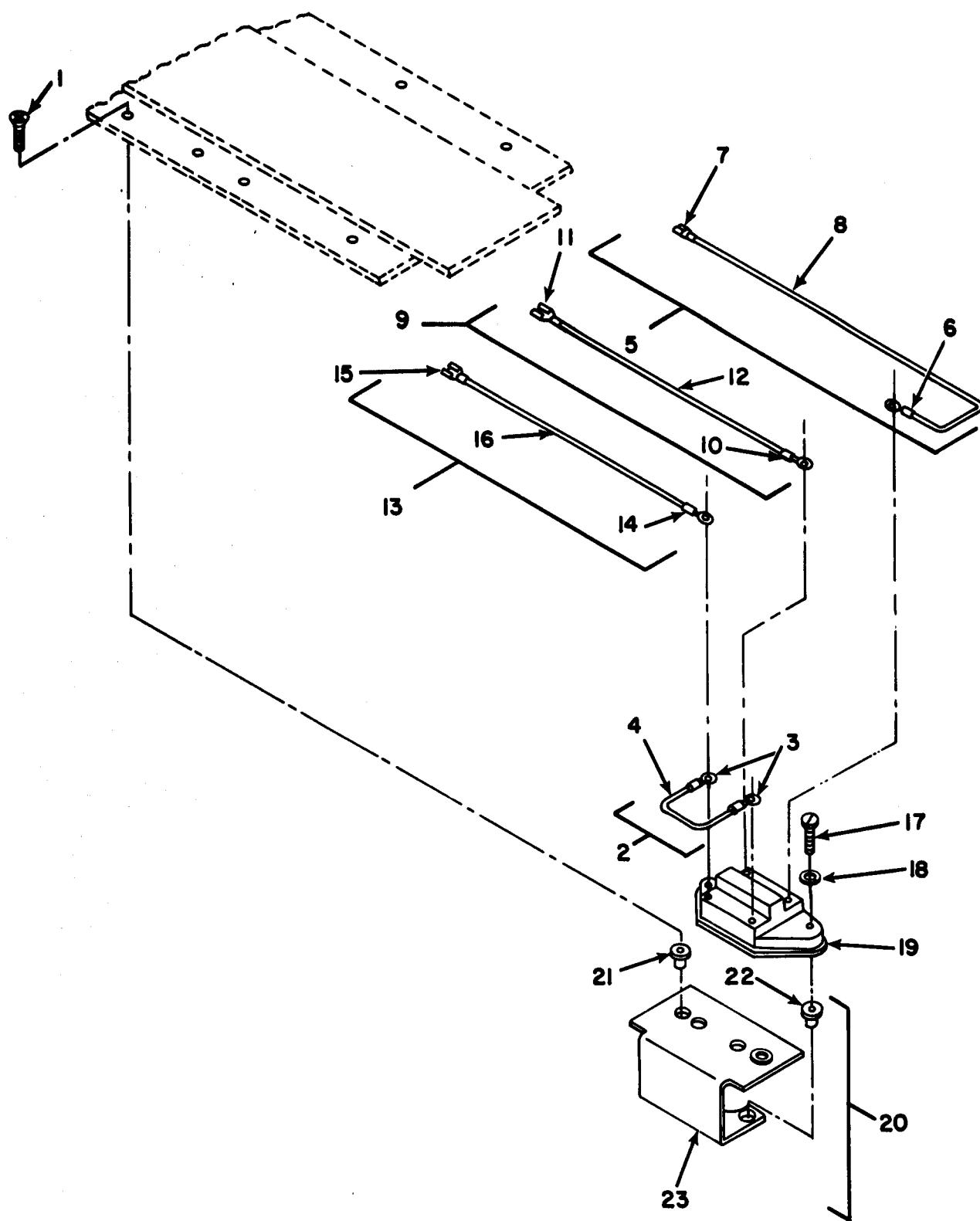
Figure 22 - Heater Thermostat
