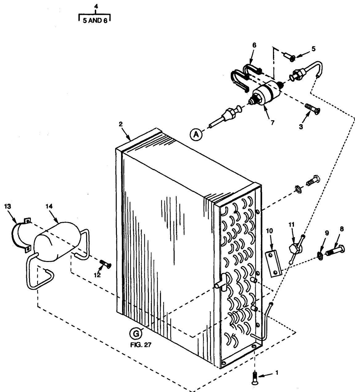
Figure 29. Condenser, Dehydrator, and Liquid Indicator.
