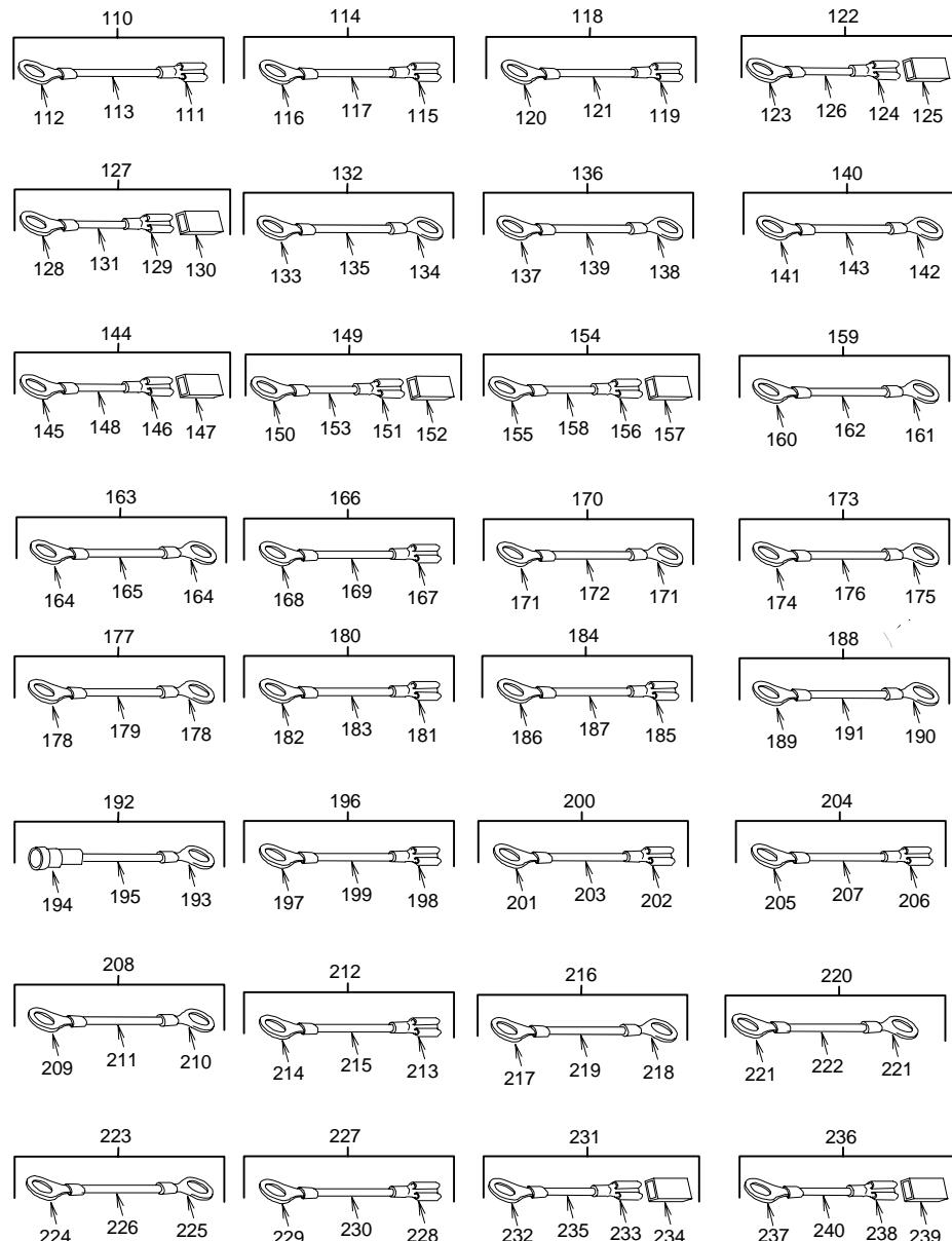
Figure 3. Control Box Wires and Cables (Sheet 2 of 3)
