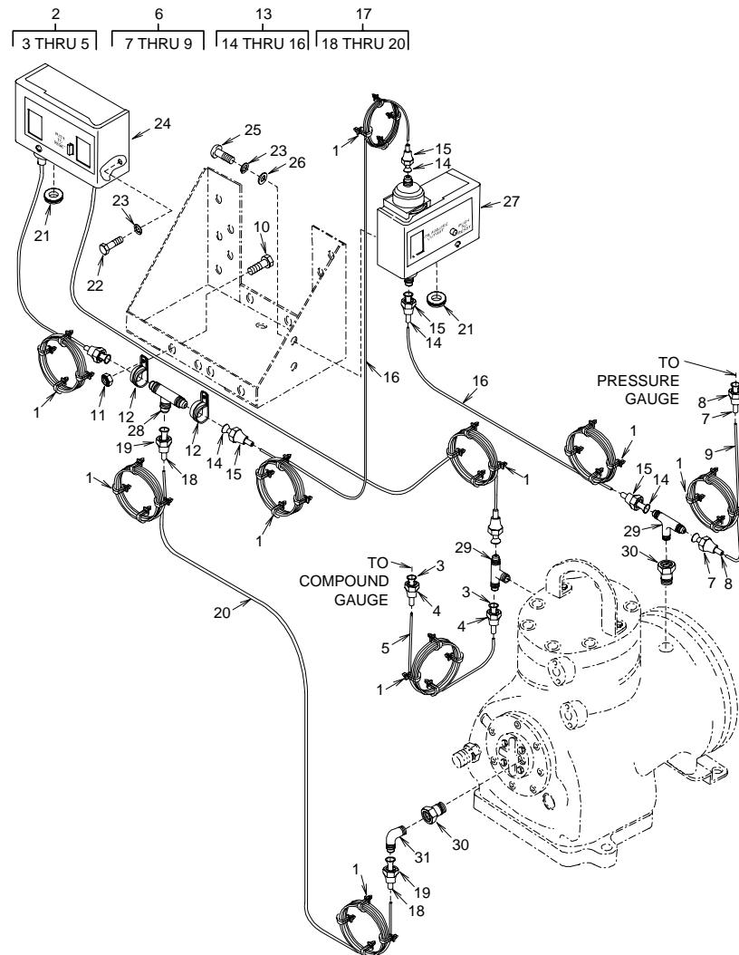
Figure 8. Pressure Switches
