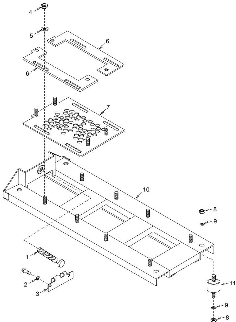
Figure 23. Engine And Compressor Base
