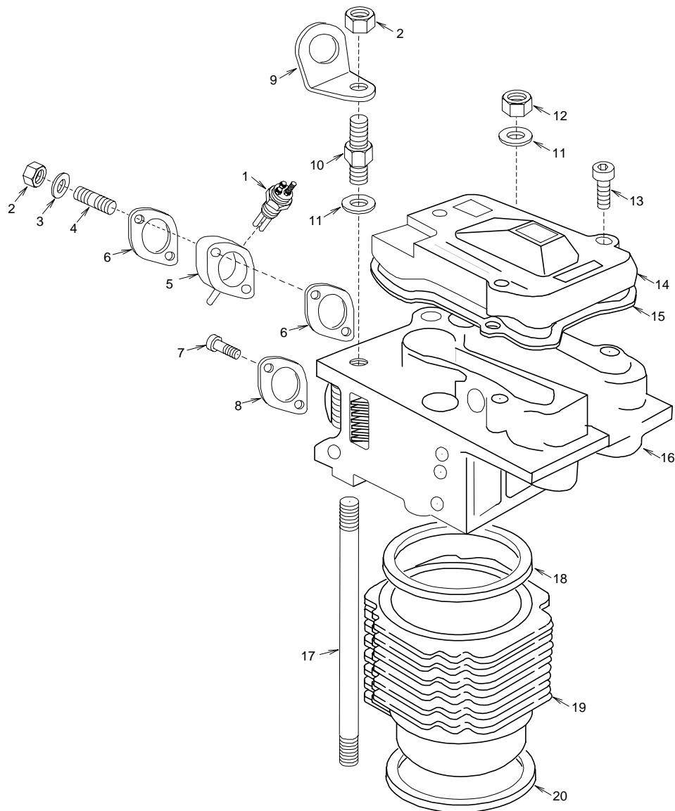
Figure 19. Cylinder Head
