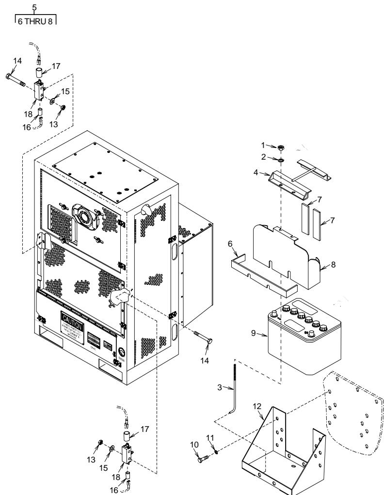
Figure 5. Battery and Door Switches
