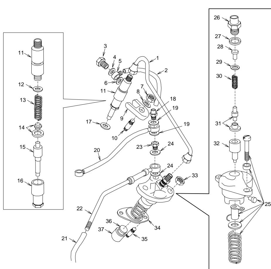
Figure 18. Injector and Injection Pump
