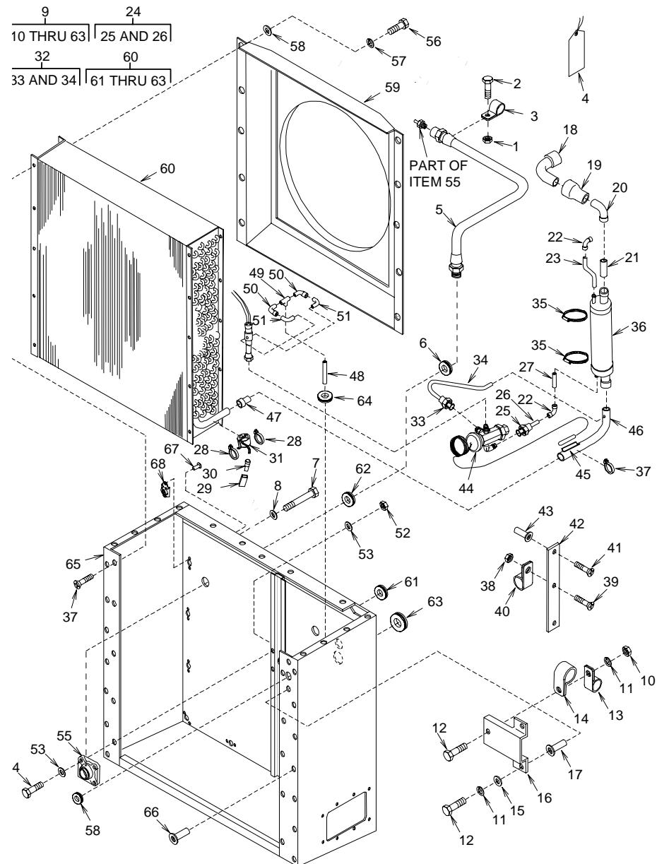
Figure 10. Evaporator Assembly
