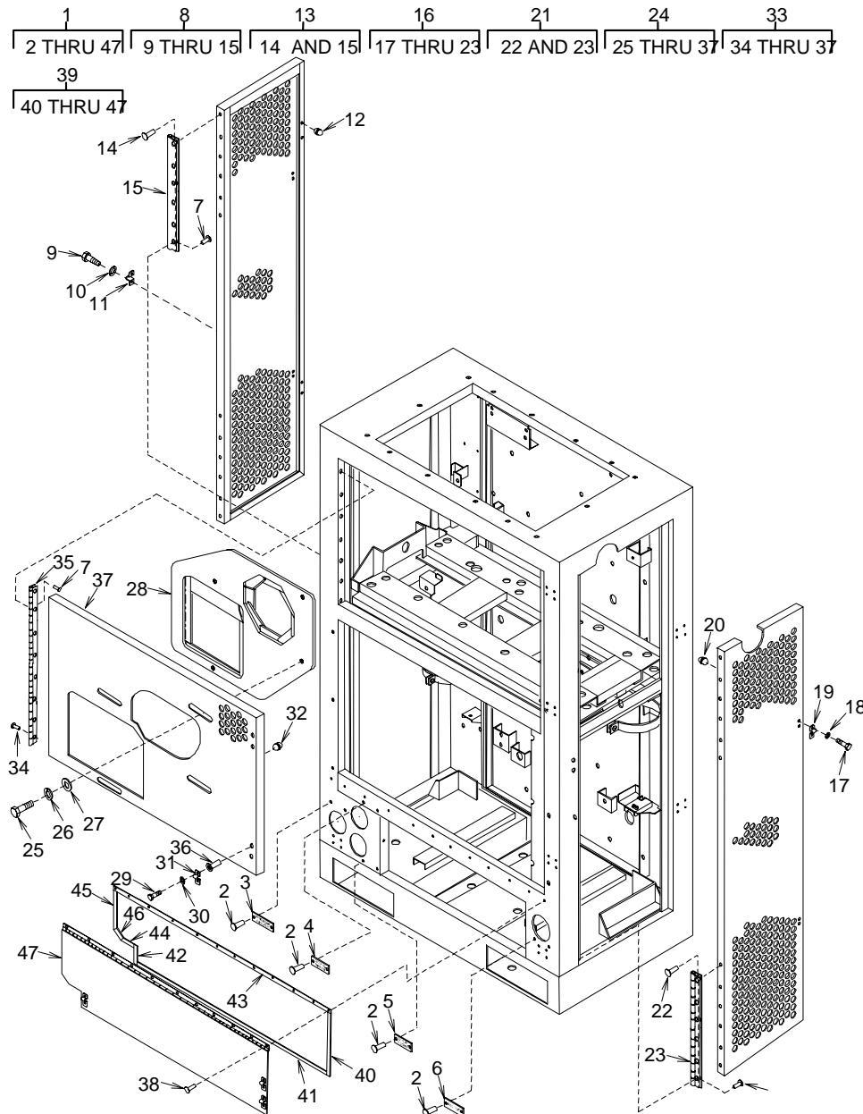
Figure 27. Unit Marking and Condenser Frame
