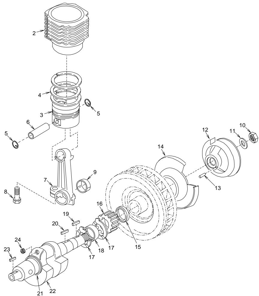
Figure 21. Crankshaft, Piston, and Flywheel
