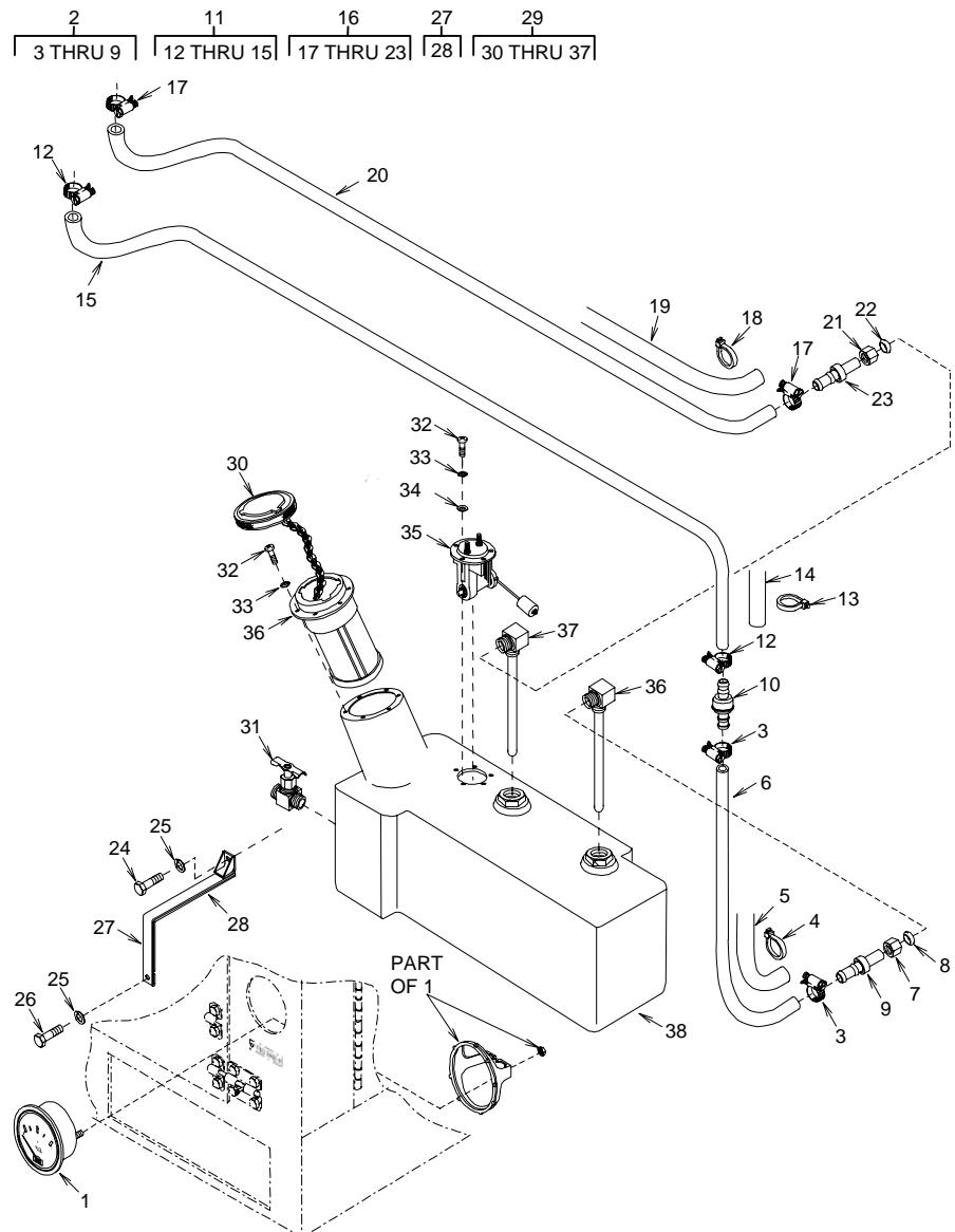
Figure 24. Fuel Tank, Gage and Hoses
