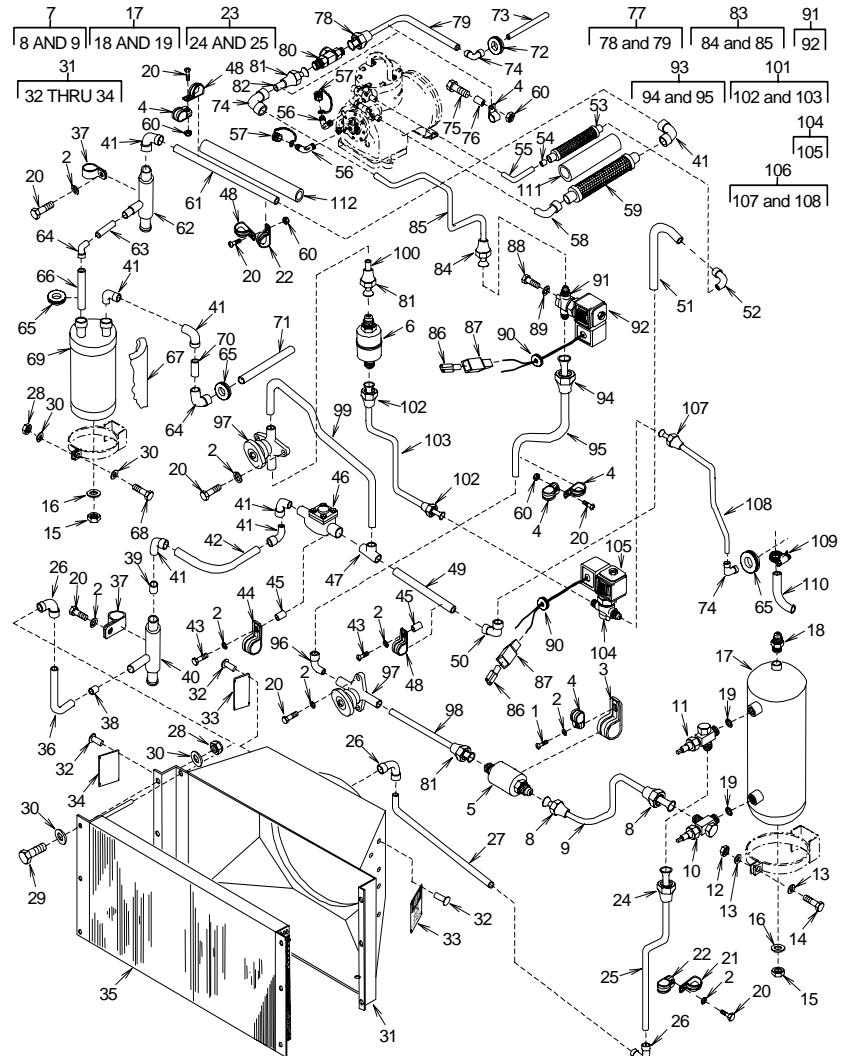
Figure 7. Refrigerant Piping, Condenser Section
