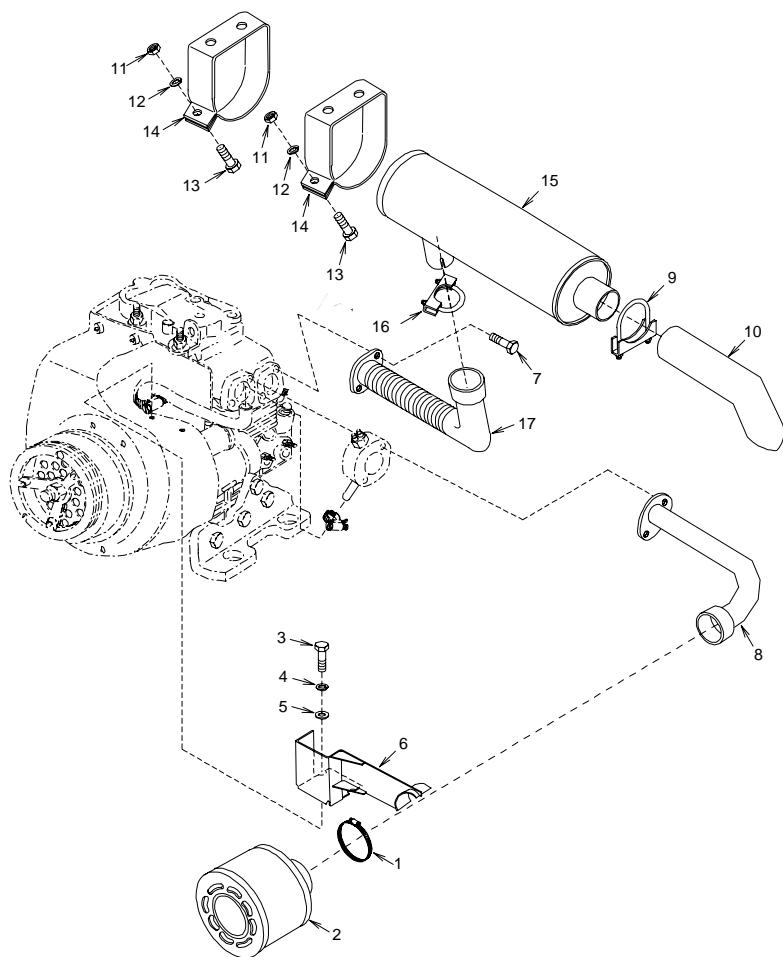
**Figure 13 Muffler and Air Cleaner**
