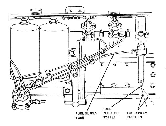
Figure 9-4. Fuel Injector Nozzle Spray Pattern
