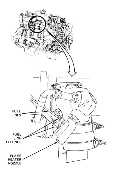
Figure 9-2. Flame Heater Nozzle, Fuel Lines, and Fittings for LDS-465-1, LDS-465-1A and LDS-465-2
