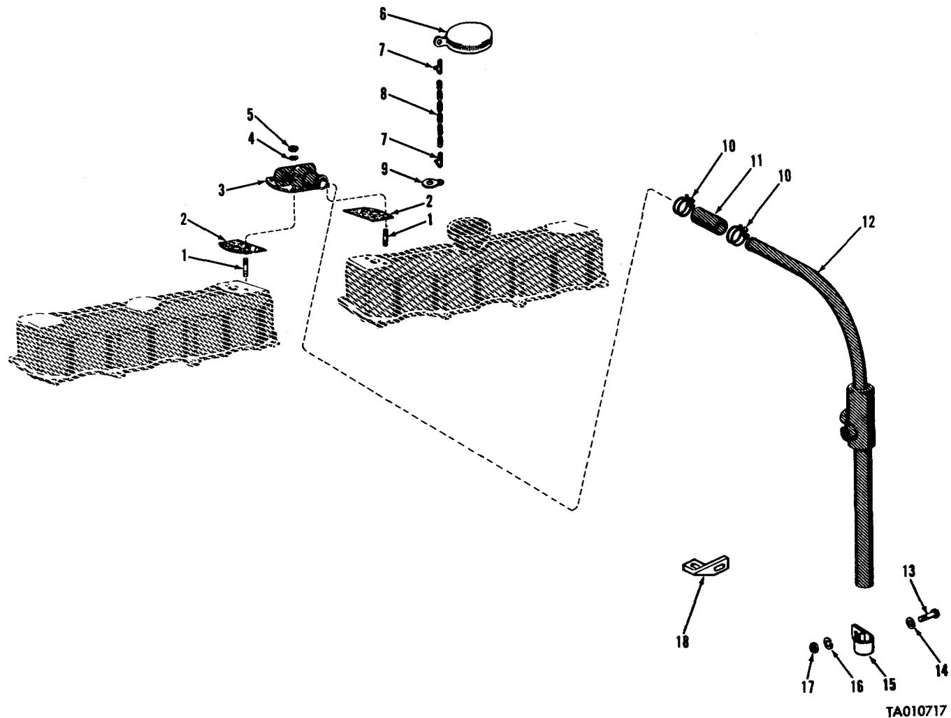
**Figure 11. Engine Crankcase Breather System and Associated Parts.**
