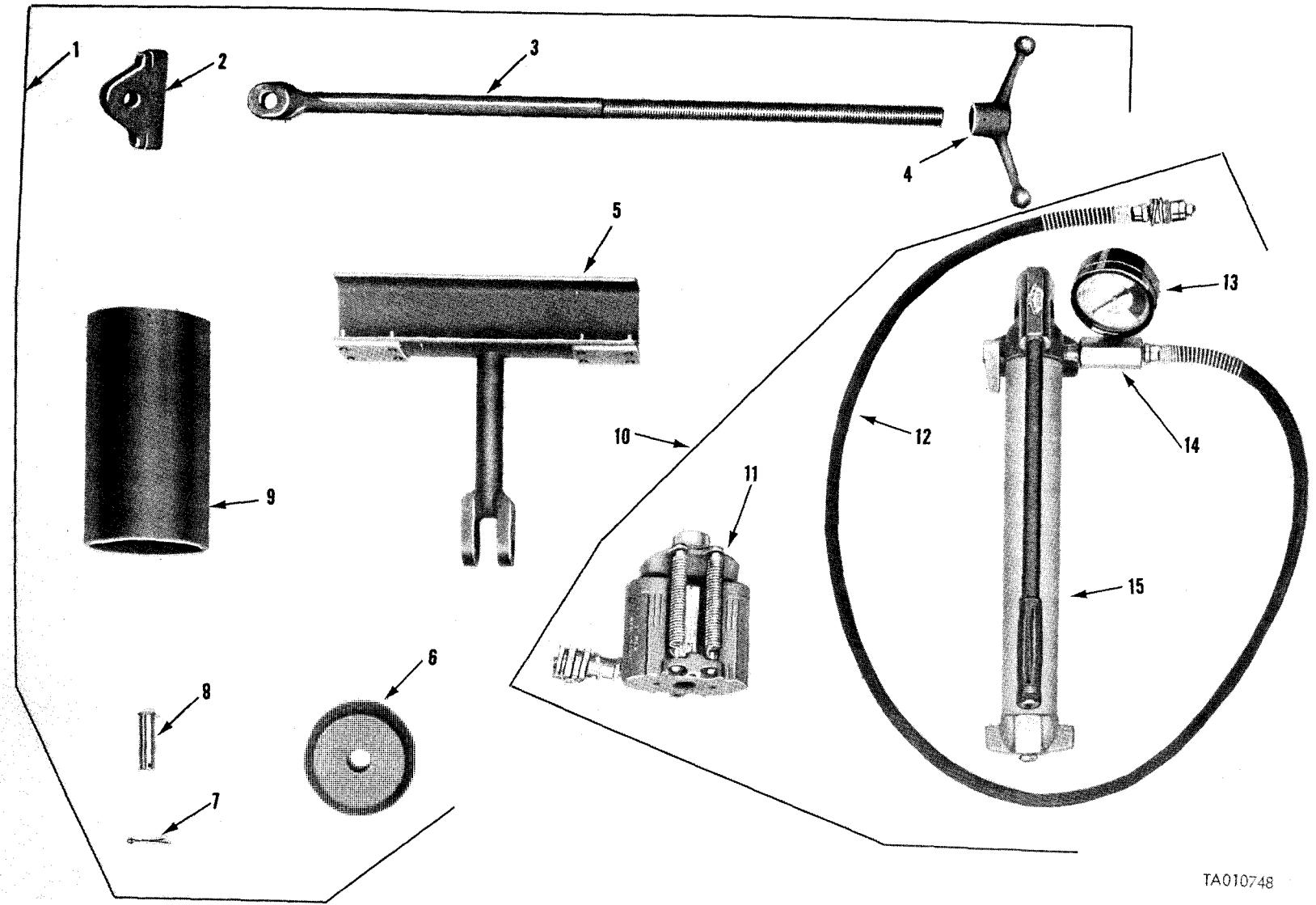
Figure 40. Remover and Replacer Kit, Cylinder Sleeve.
