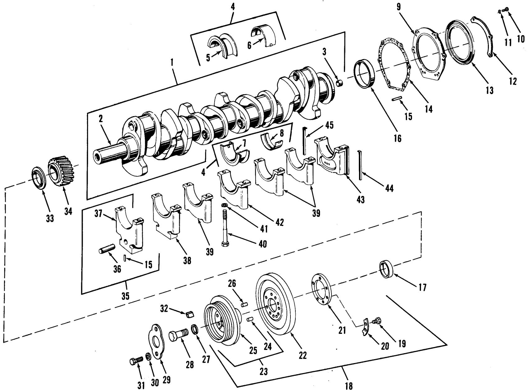
Figure 3. Crankshaft, Main Bearings and Associated Parts.
