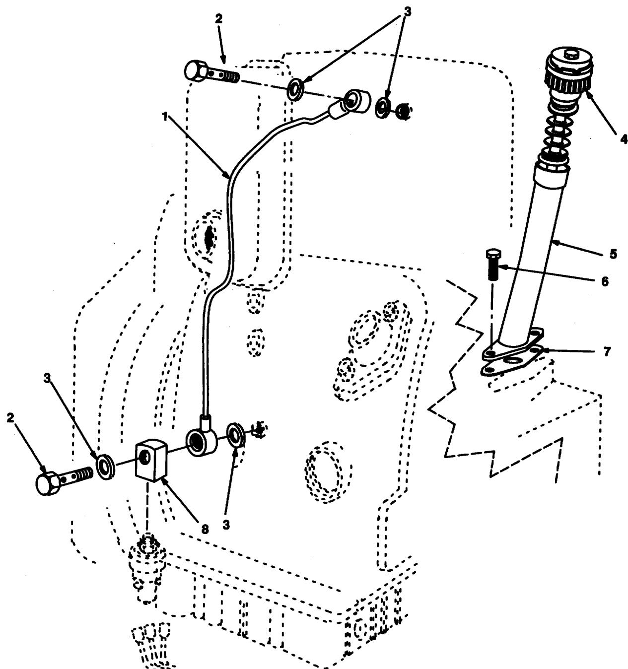
FIGURE 41. OIL FILLER AND LUBRICATION SYSTEM (Sheet 1 of 2)
