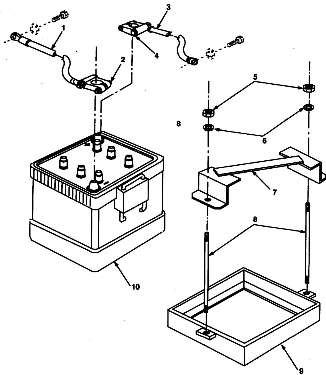
FIGURE 3. BATTERY, CABLES AND HOLD-DOWN CLAMP.
