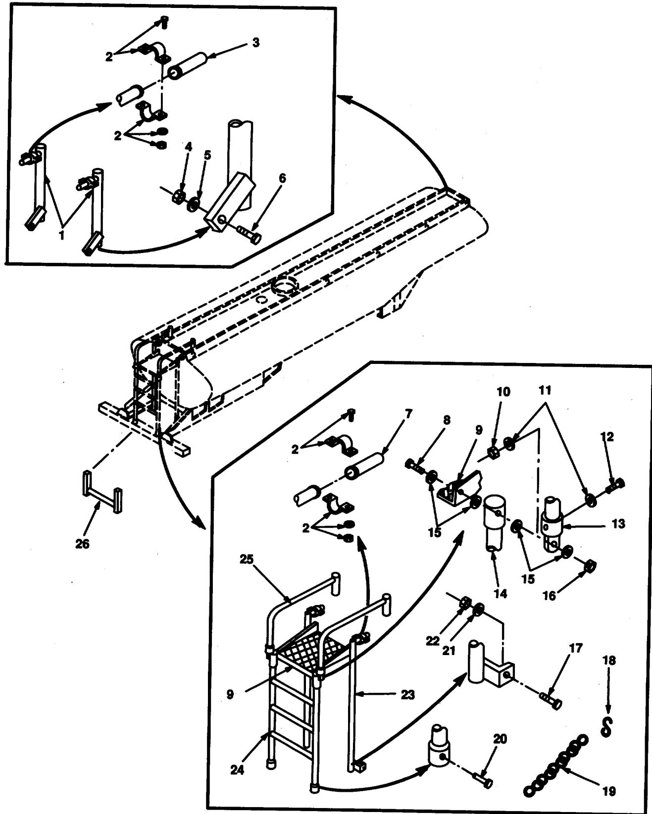
FIGURE 34. LADDER AND DRAIN ASSEMBLY.
