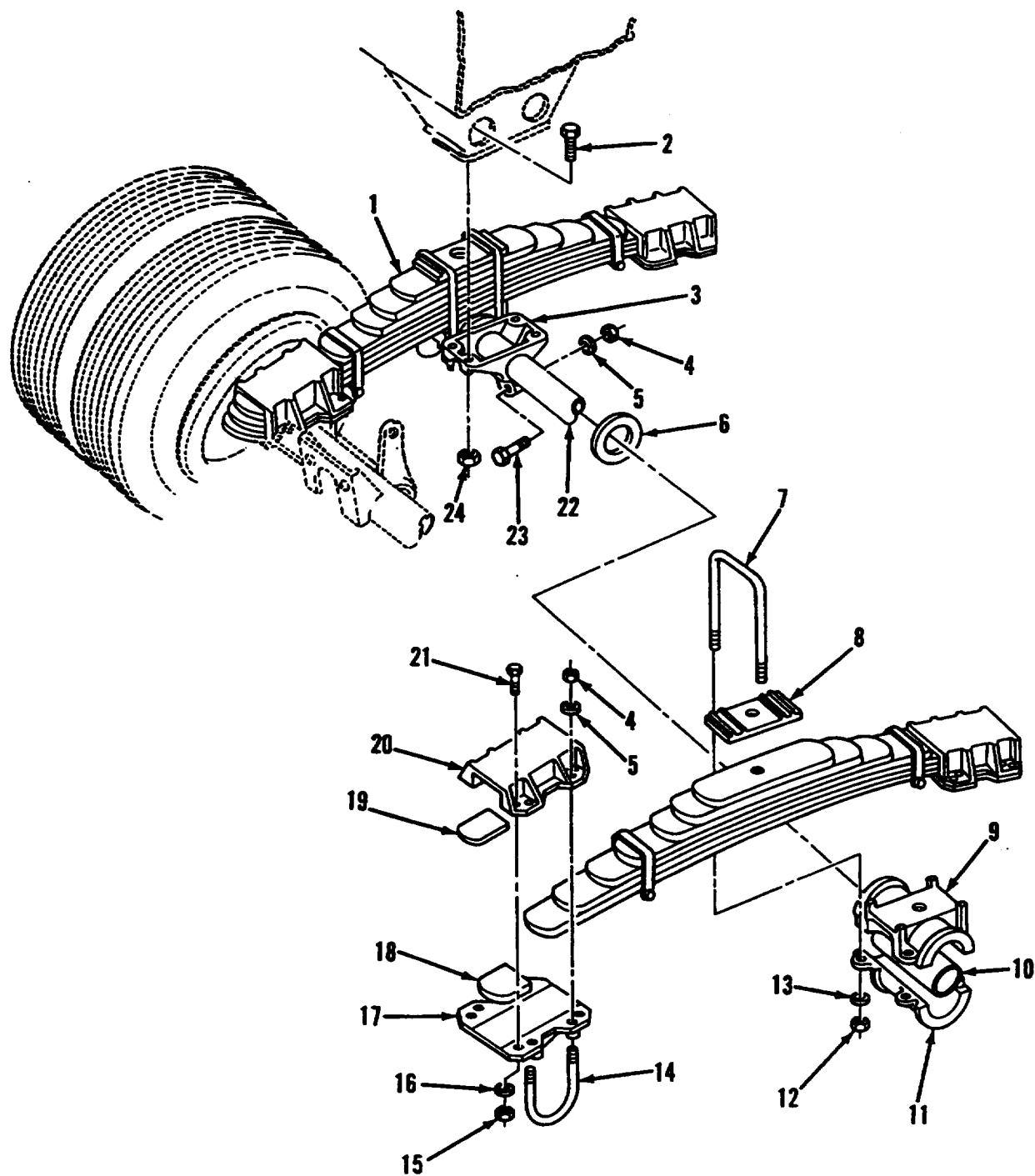
FIGURE 28. SUSPENSION ASSEMBLY
