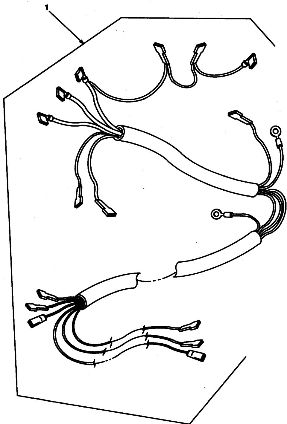
FIGURE 52. ENGINE WIRING HARNESS.
