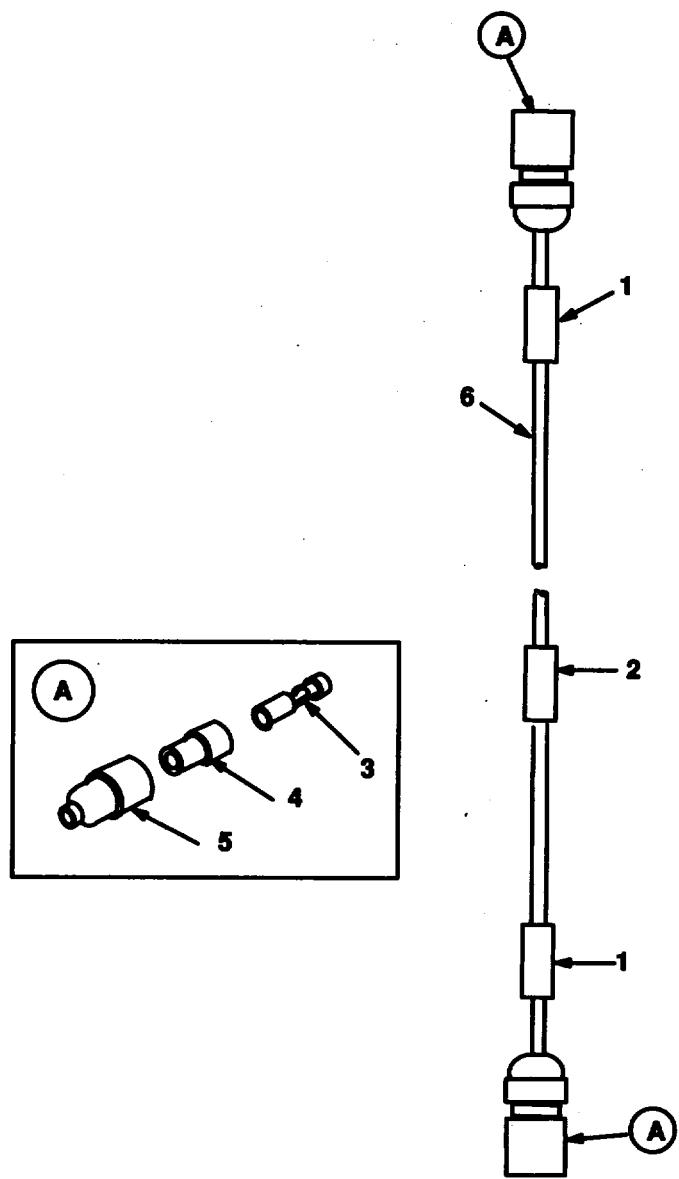
FIGURE 11. WIRING HARNESS COMPONENTS.
