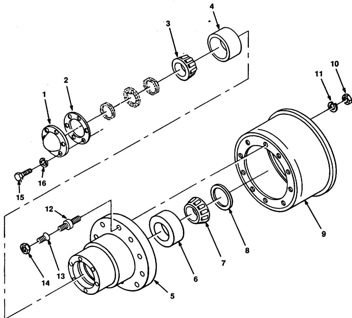
FIGURE 21. HUB AND DRUM ASSEMBLY
