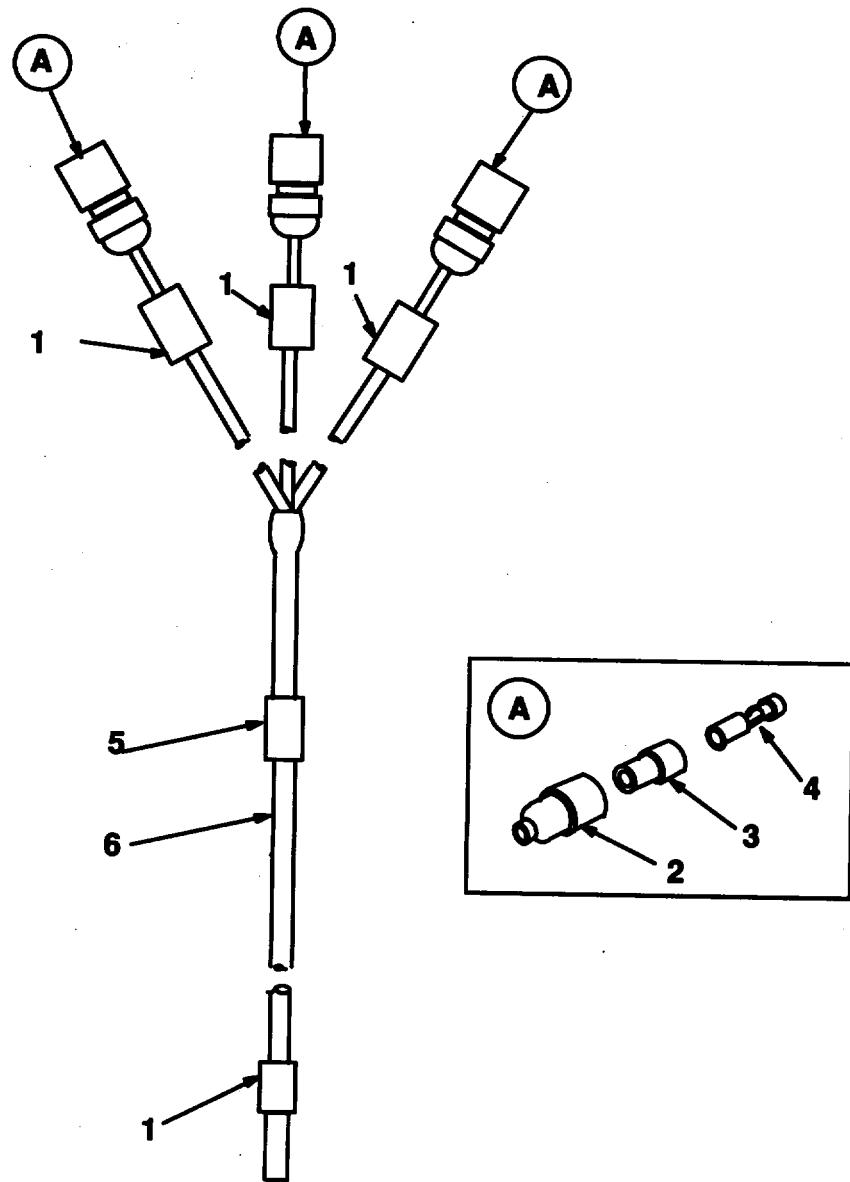
FIGURE 10. WIRING HARNESS COMPONENTS.
