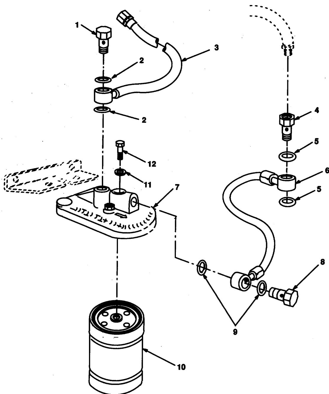
FIGURE 45. FUEL- WATER SEPARATOR
