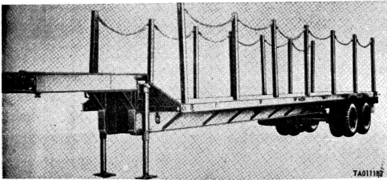
Figure 5. Semitrailer, low bed: wrecker, M269A1-left front view.
