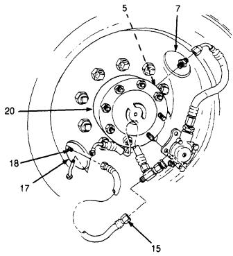
(2) If replacing inner tire, connect hose (15) to inner wheel valve
