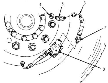
(5) Remove protective plug from wheel valve (8) and install on wheel valve of defective tire.
