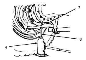
(b) For rear tire replacement, place jack (4) so jack ram (3) is under equalizing beam (6) inboard of equalizing beam end adapter (5).
