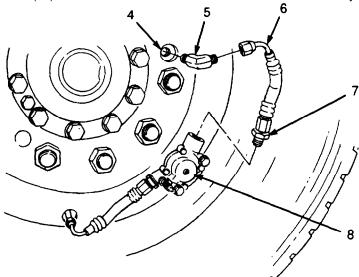
(10) Remove wheel nuts and wheel and tire assembly.
