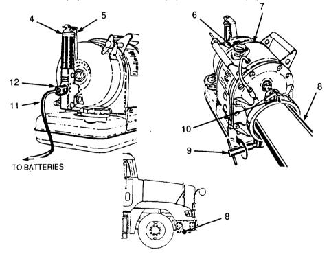
(12) To turn heater off, close fuel regulator (6) completely. When pulsating stops, heater is off.
