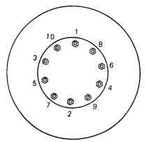
WHEEL NUT TIGHTENING PATTERN
