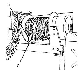
(3) To pay out wire rope, pull up and hold line control lever (4) in LINE OUT position. Winch unwinds in low speed. Have crew member walk end of wire rope out.
