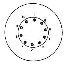
(10) Remove two hub nuts (11) at 4 and 5 o'clock position.
