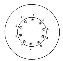
WHEEL NUT TIGHTENING PATTERN
