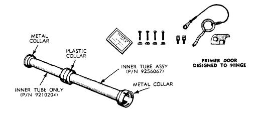
• INNER TUBE ASSEMBLY OR SUBCALIBER TUBE IS ALUMINUM WITH A SMOOTH BORE MACHINED TO ACCEPT THE SUBCALIBER. 35MM, PRACTICE ROCKET
