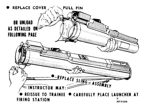
TO UNLOAD KEEP LAUNCHER ON TARGET.
