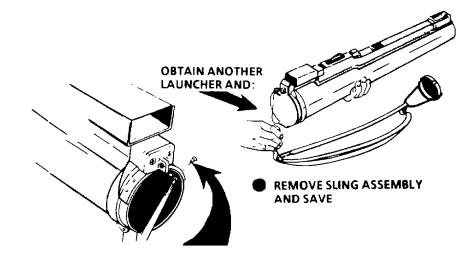
PUNCH OUT RIVETS SECURING INNER TUBE TO LAUNCHER (OUTER TUBE), USE 1/16" PUNCH DISCARD RIVETS
