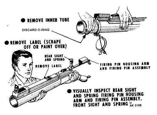
• IF ASSEMBLY IS USABLE, THE SUBCALIBER TUBE IS PLACED INTO THE <u>MODIFIED OUTER TUBE</u>. THE <u>INNER TUBE</u> IS PLACED OVER THE REAR OF THE <u>SUBCALIBER TUBE</u> AND THE ENTIRE ASSEMBLY IS TELESCOPED INTO THE CLOSED POSITION.
