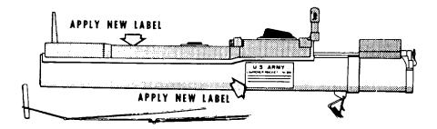
IF COMPLETED LAUNCHER IS FREE OF MECHANICAL DEFECTS APPLY LABEL. LABEL IS PRESSURE SENSITIVE, SELF-ADHERING. PEEL OFF BACKING AND APPLY LABEL TO DRY SURFACE ONLY.
