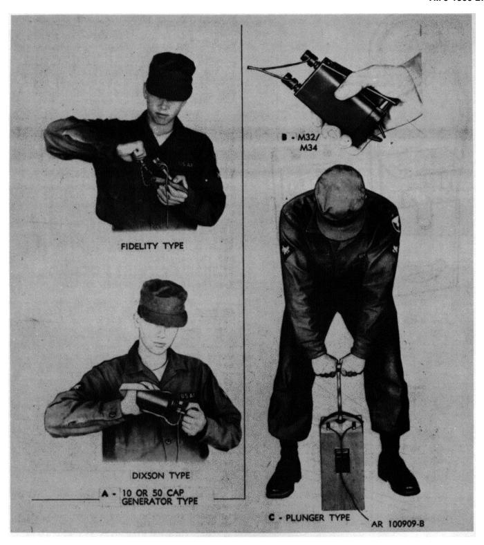
Figure 4-20. Actuating blasting machines.
