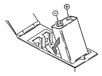
FIGURE 3-9. Torso Harness Battery Installation
