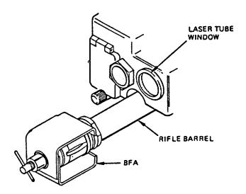
FIGURE 2-9. BLANK-FIRE Attachment (typical)
