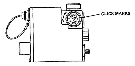
FIGURE 2-14. Laser Adjustor 'Click' Marks
