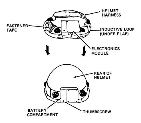
FIGURE 3-3. Attaching the Helmet Harness
