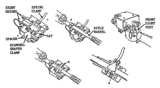
FIGURE 2-8. Installing the SAT on the M16A2 Using the Universal Bracket
