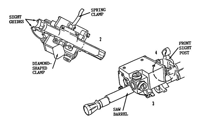
FIGURE 2-6. Installing the SAT on the SAW Barrel
