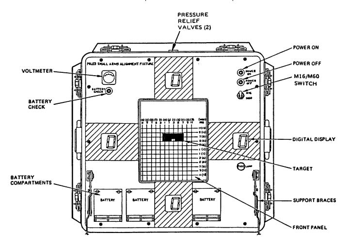
FIGURE 4-1. Small Arms Alignment Fixture Assembly (P/N 11835282)
