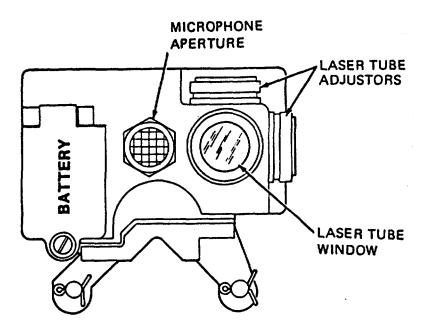
FIGURE 2-2. Inspecting and Cleaning the SAT
