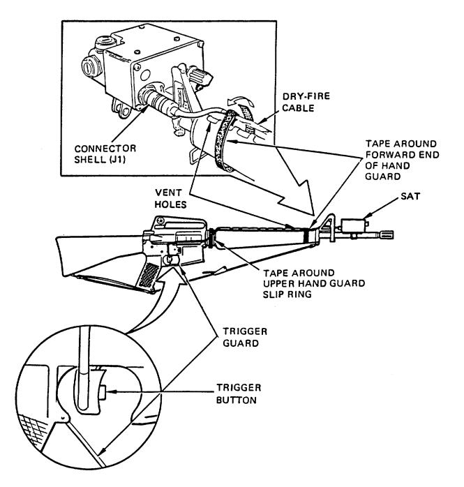
FIGURE 2-11. DRY-FIRE Cable Installation
