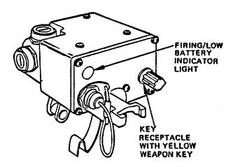
FIGURE 2-10. SAT Rear View
