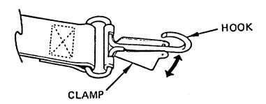
FIGURE 3-5. Securing Clamp
