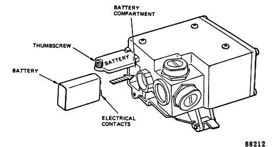
FIGURE 2-3. SAT Battery Installation
