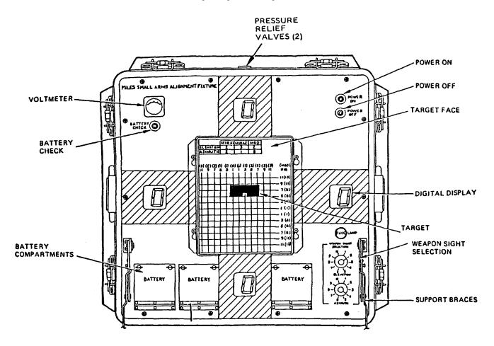
FIGURE 4-2. Small Arms Alignment Fixture Assembly (P/N 9353020)
