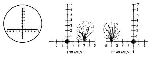
Fire corrections can be made by viewing the impact area and determining angular corrections by use of the left or right horizontal reticle scale. USE OF RETICLE (CONT'D)
