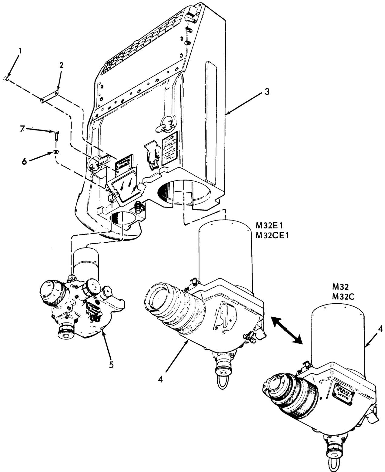
Figure 1. Tank periscope, M32 10514284, M32C 10516600, M32E1 11747400, and M32CE1 11747440
