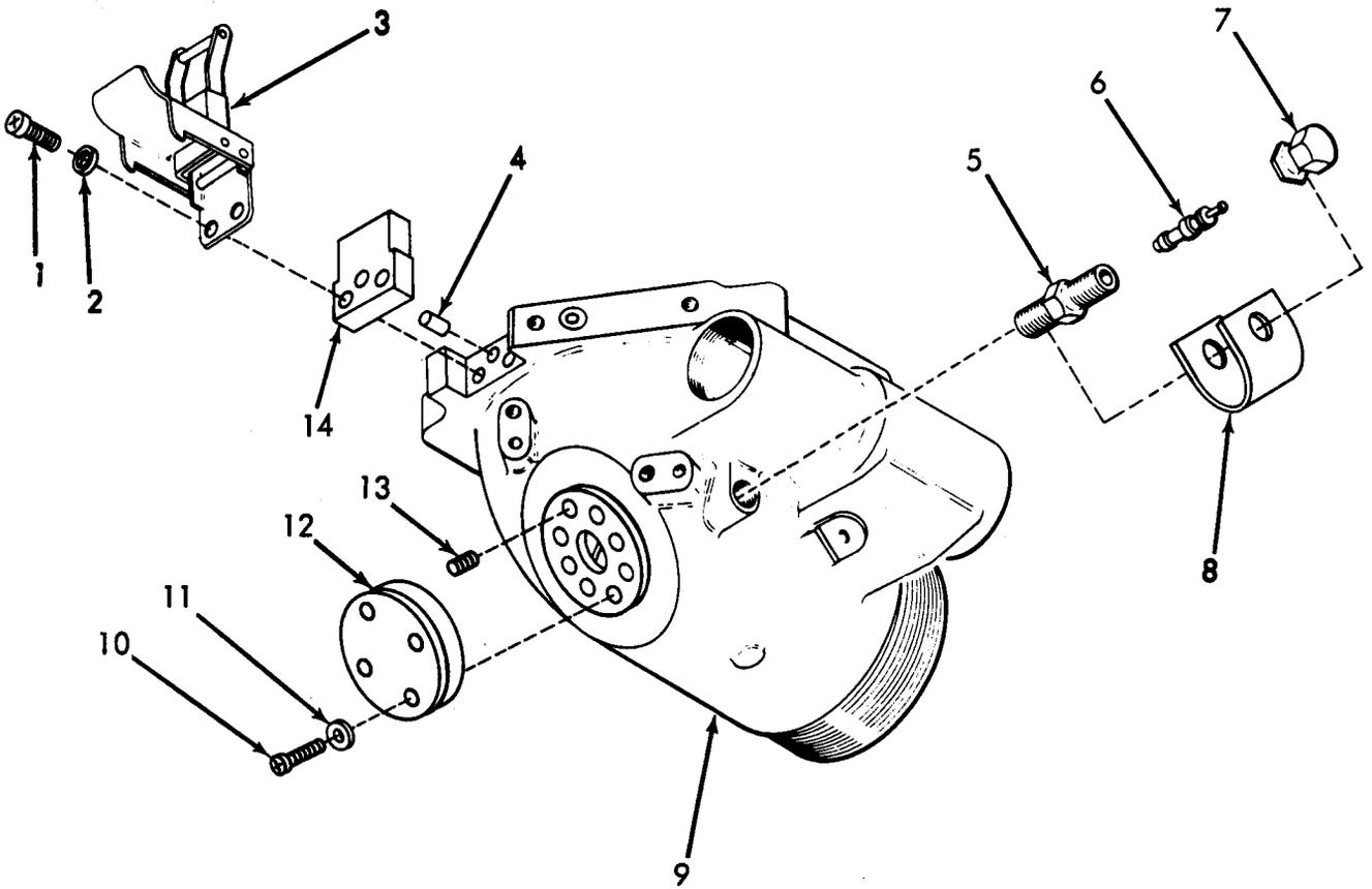
Figure 9. Body assembly (infrared) 11743800 (partial view-bottom)
