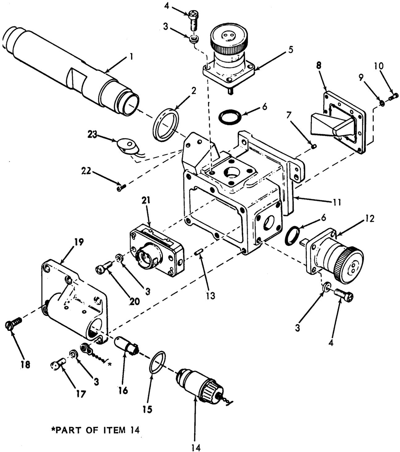
Figure 10. Body assembly (infrared) 11743800 (partial view-back)
