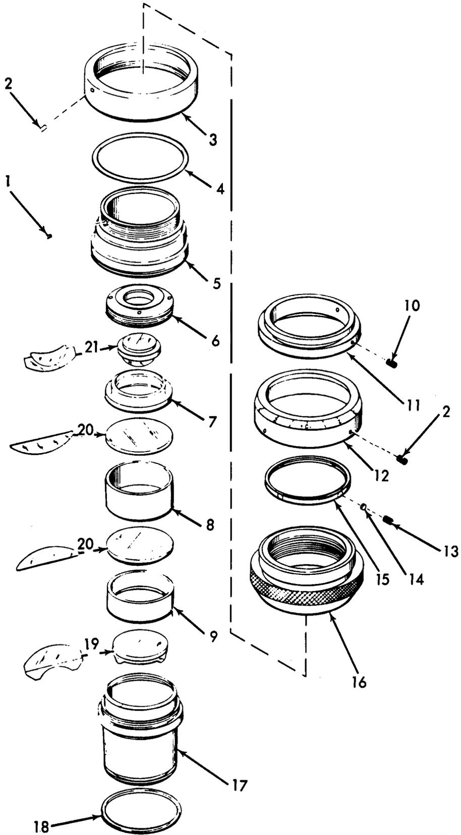
Figure 19. Eyepiece assembly 11733402
