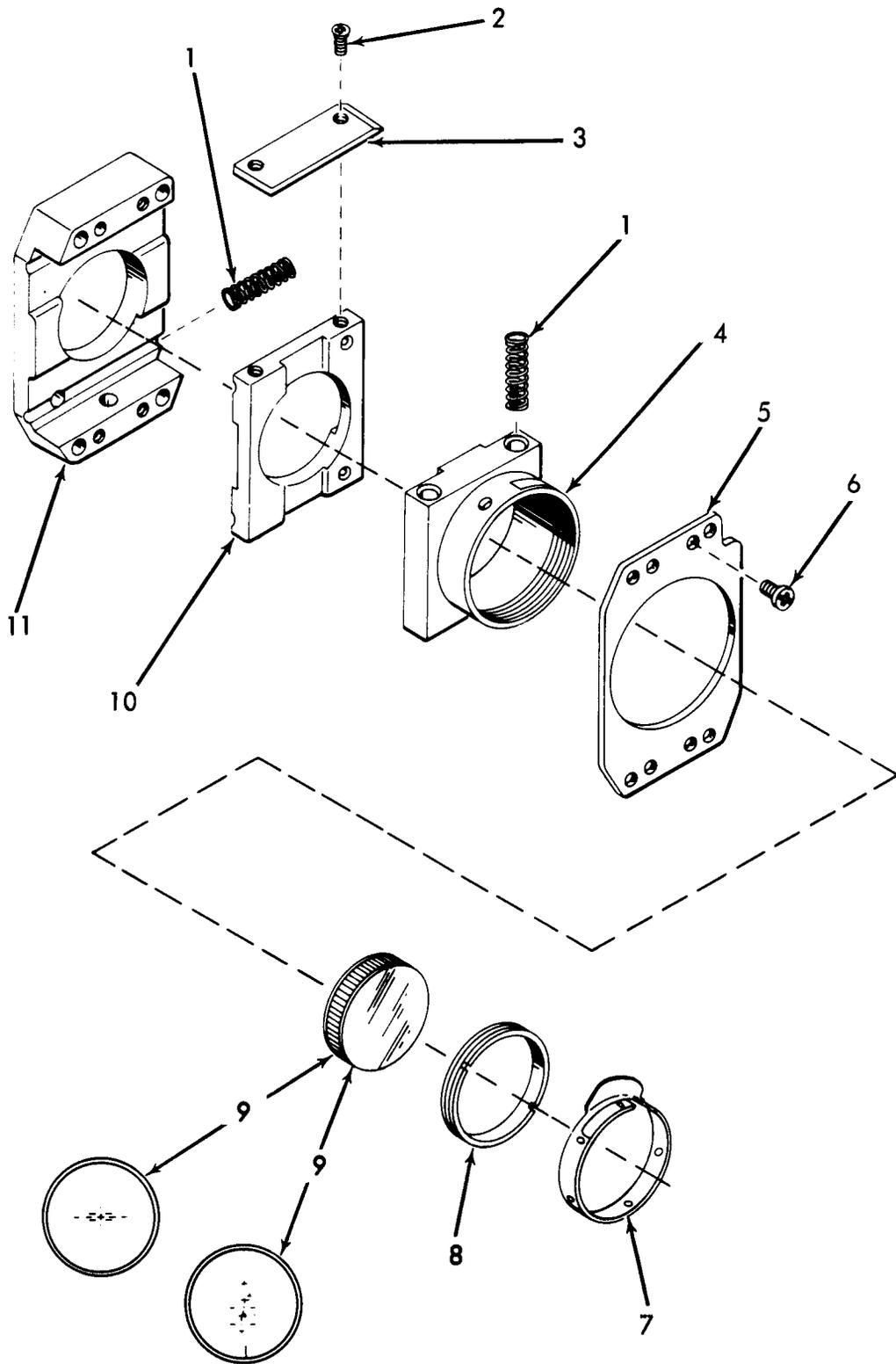
Figure 6. Optical cell assembly 10516366 and 8289218
