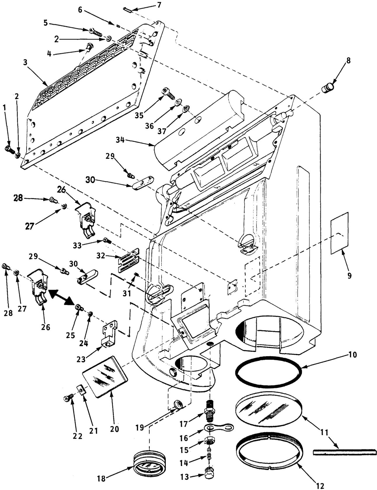
Figure 2. Head assembly 11727486, 10541990, and 11747439 (partial view-back)
