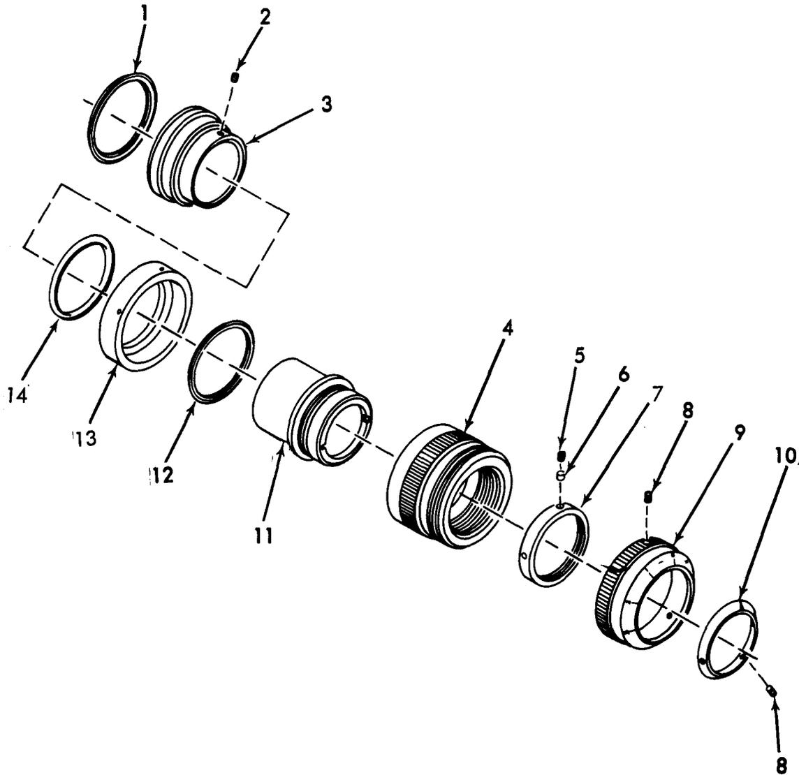
Figure 12. Eyepiece assembly 10516734
