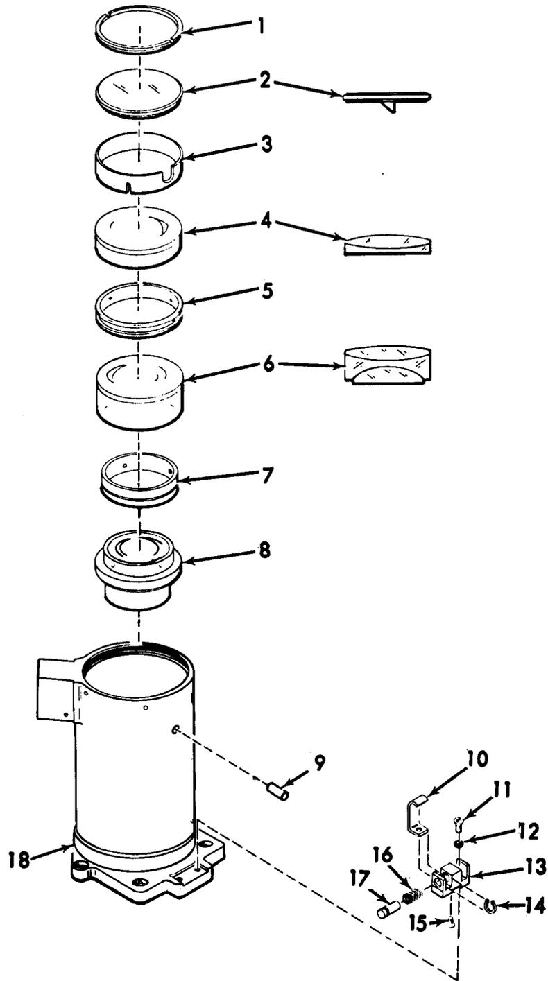
Figure 18. Prism cell 11733403
