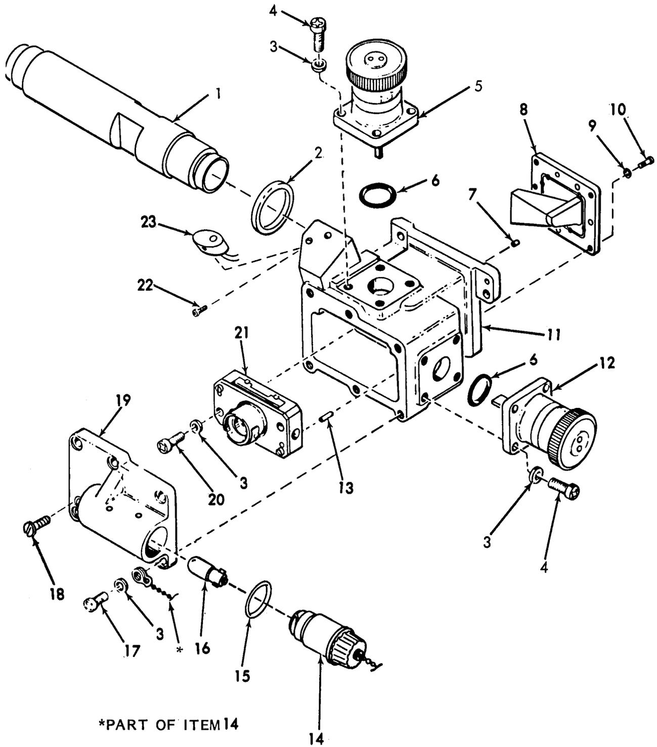
Figure 17. Elbow telescope (passive) 11733401 (partial view-back)
