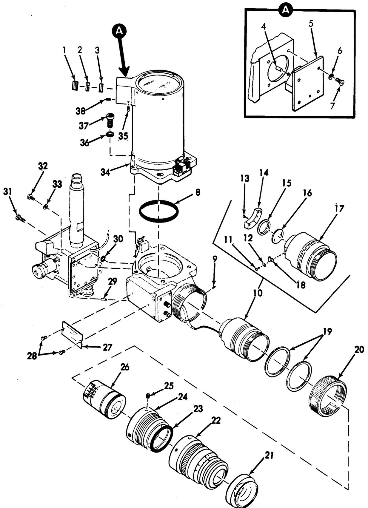
Figure 14. Elbow assembly (passive) 11733401 and Adapter assembly 11733480
