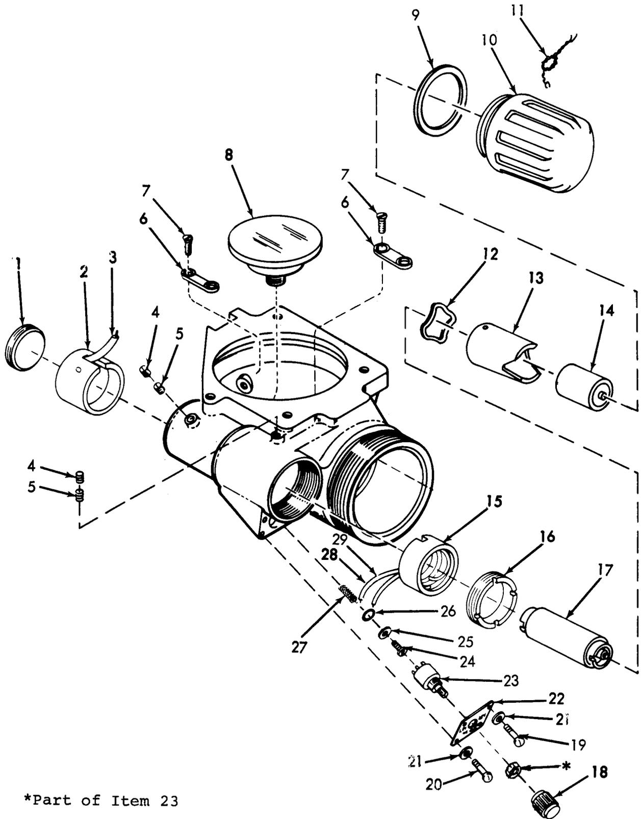
Figure 8. Body assembly (infrared) 11743800 (partial view-top)
