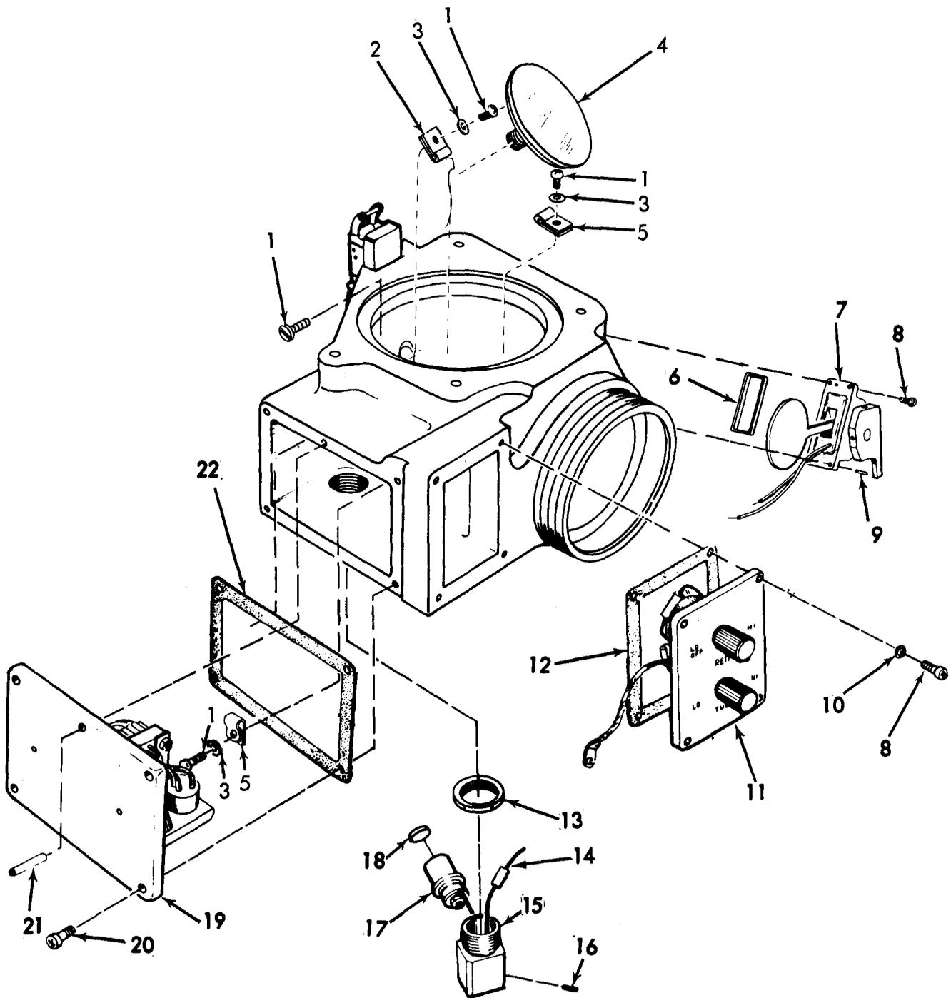
Figure 15. Elbow assembly (passive) 11733401 (partial view-top)
