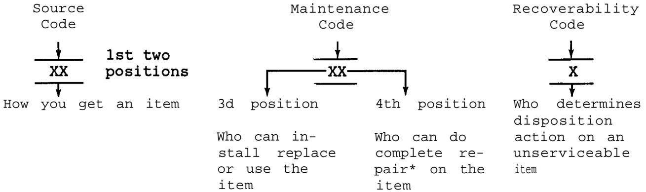
\*Complete Repair: Maintenance capacity, capability, and authority to perform all corrective maintenance tasks of the "Repair" function in a use/user environment in order to restore serviceability to a failed item.
