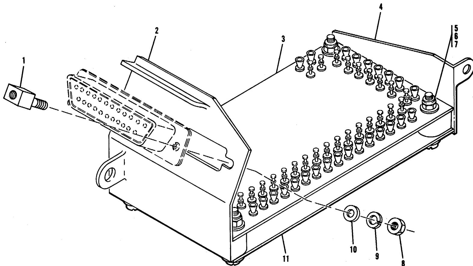
Figure 45. Readout Circuit Assembly 11737350 (A79A2)-partial exploded view.
