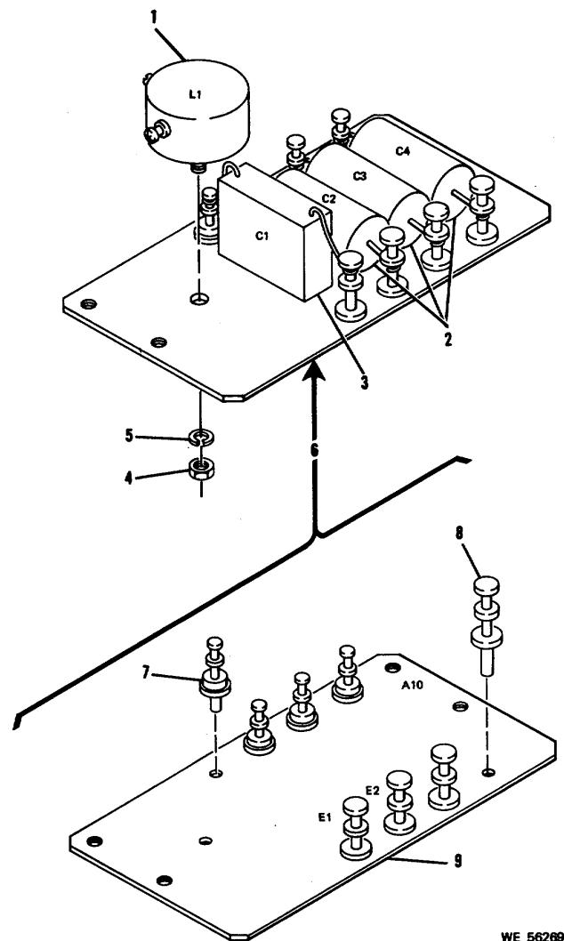
Figure 13. Q Switch Filter 11741557 (A76A10)--partial exploded view.
