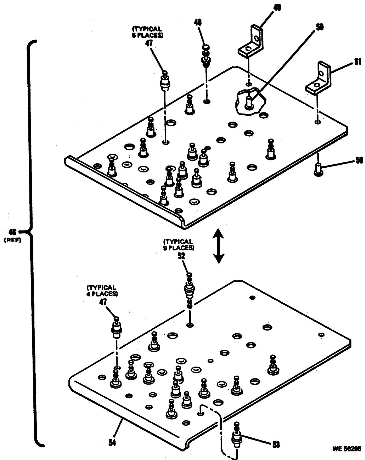
Figure 39. Electronic Component Assembly 11738850 (A78A2) - partial Exploded view (Sheet 2 of 2)
