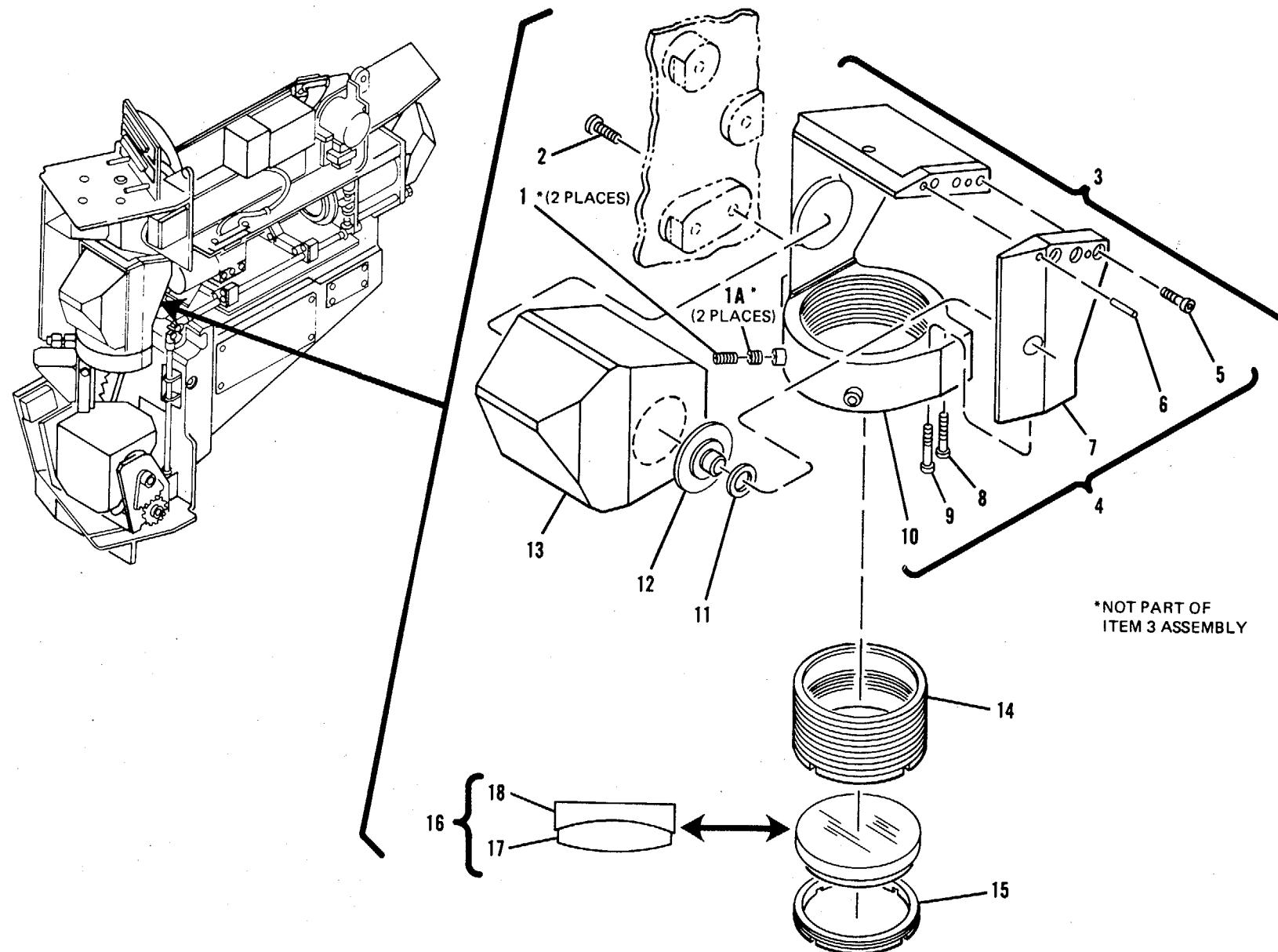
Figure 7. Optical Bench Assembly 11737374-explored view. (Sheet 1 of 5)
