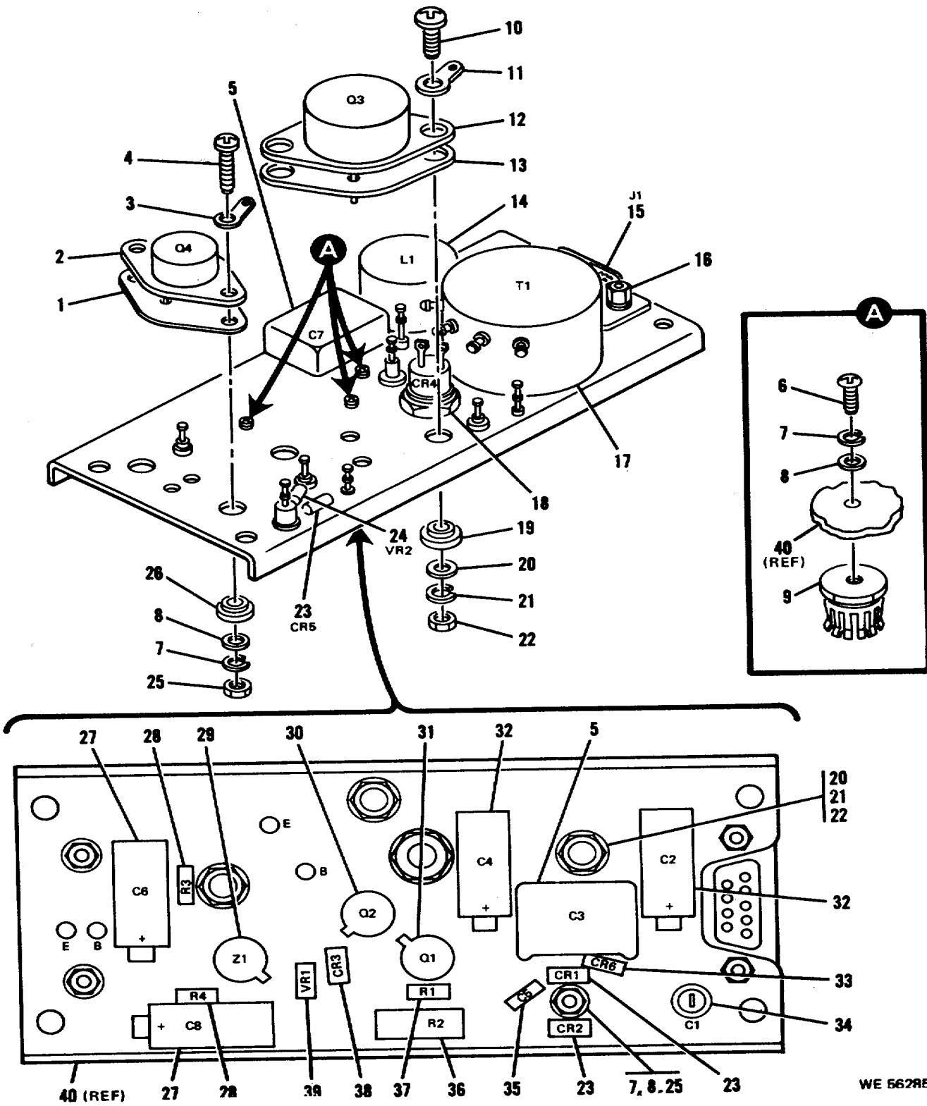
Figure 28. Preregulator Electronic Component Assembly 11737807 (A77A10)-partial exploded view. (Sheet 1 of 2)
