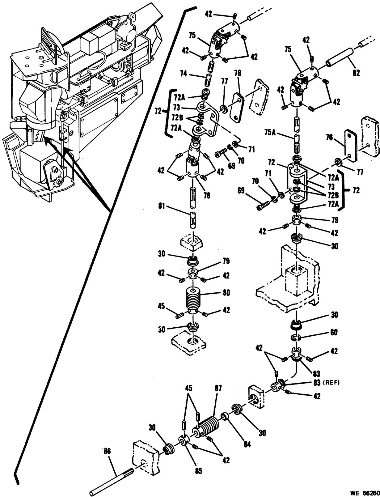
Figure 7. Optical Bench Assembly 11737374 - exploded view. (Sheet 4 of 5)
