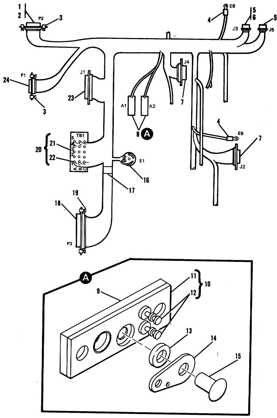
Figure 14. Wiring Harness 11737445 (W1)--partial exploded view.
