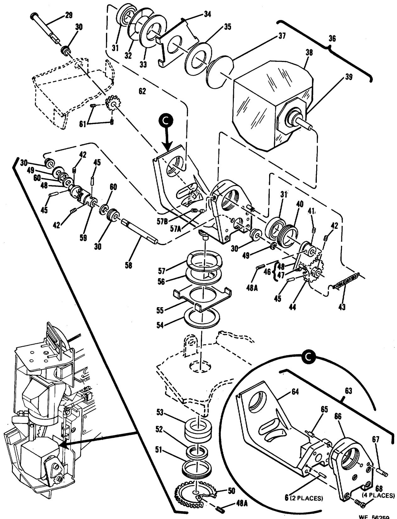
Figure 7. Optical Bench Assembly 11737374-exploded view. (Sheet 3 of 5)
