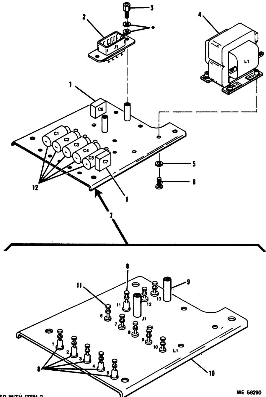
Figure 36. Filter Electronic Component Assembly 11737811 (A77A8)-partial exploded view.
