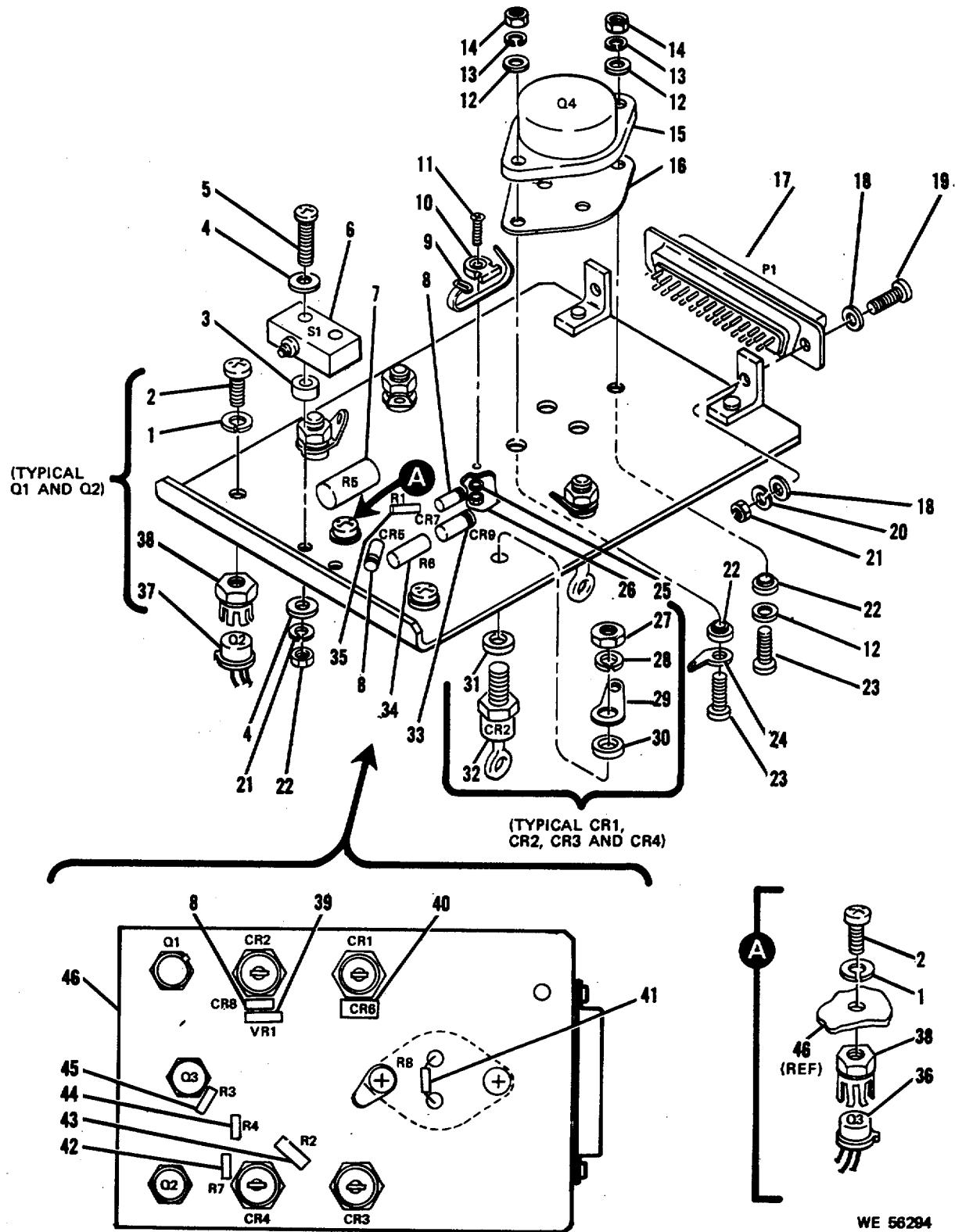
Figure 39. Electronic Component Assembly 11738850 (A78A2)-exploded view. (Sheet 1 of 2)
