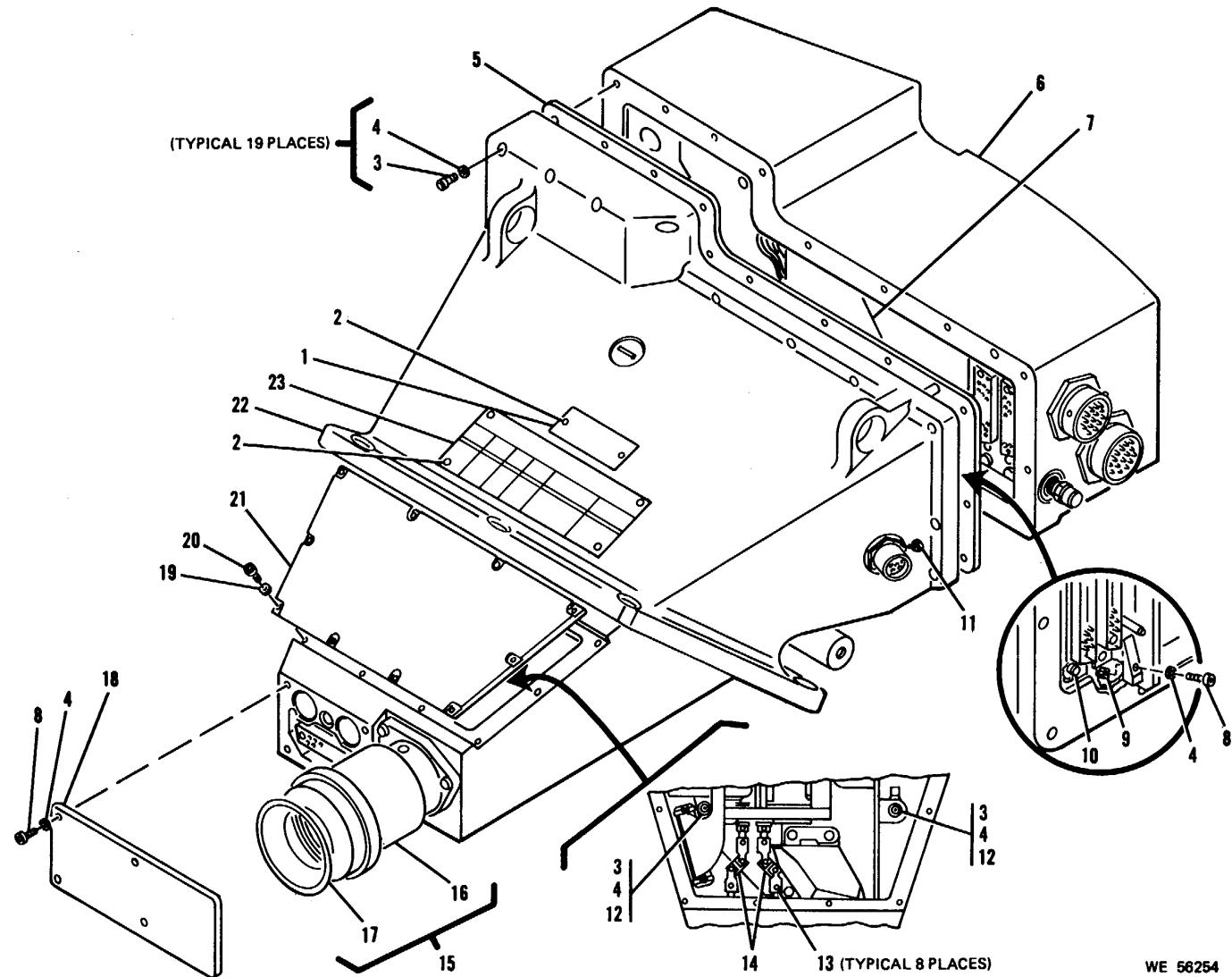
Figure 5. Laser-RT1021 VVG-1 Receiver-Transmitter 11738821 (A76)-exploded view.
