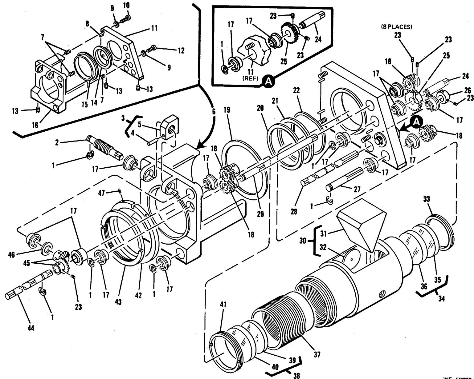
Figure 9. Derotation Prism 11737321 - exploded view.
