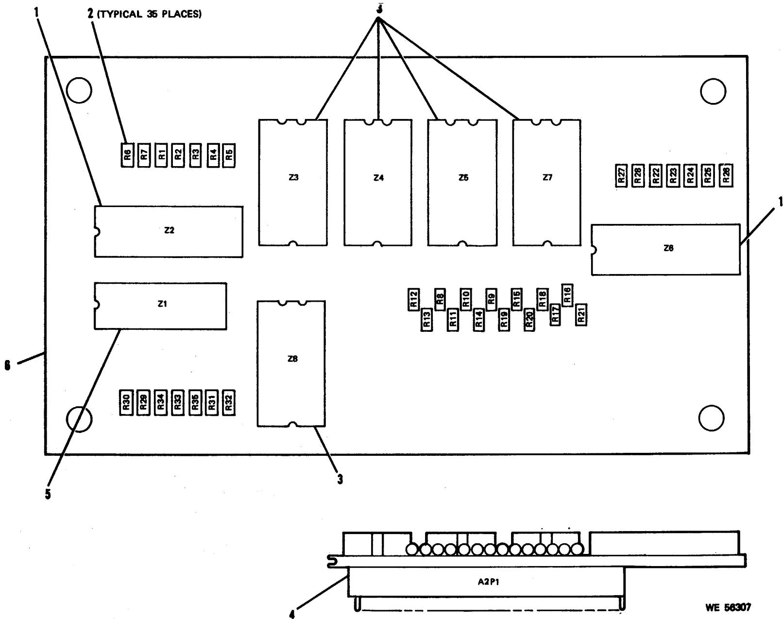
Figure 47. Readout Circuit Card Assembly 11737339 (A79A2A2)
