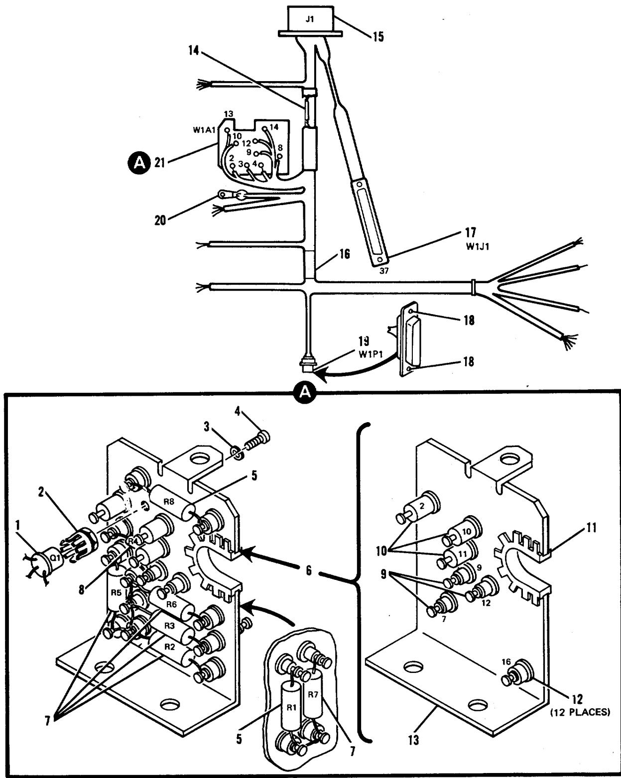
Figure 43. Wiring Harness 11738813 (A79WI)-partial exploded view.
