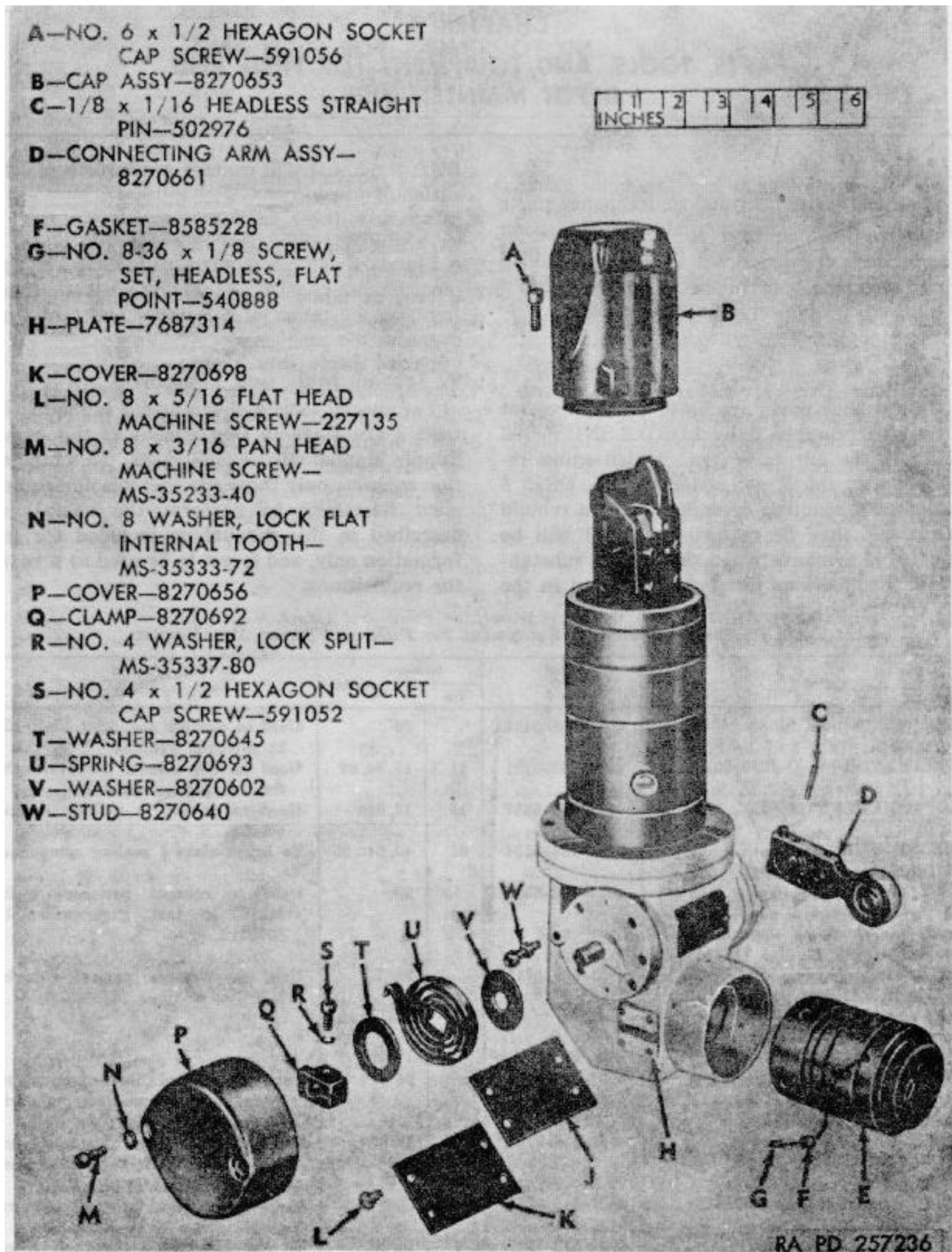
Figure 6. Periscope-exploded view showing cap, arm, and spring assemblies.
