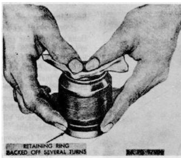
Figure 13. Applying pressure to loosen sealed lens.
