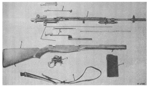
Figure 3-1. Weapon field stripped (M14).
