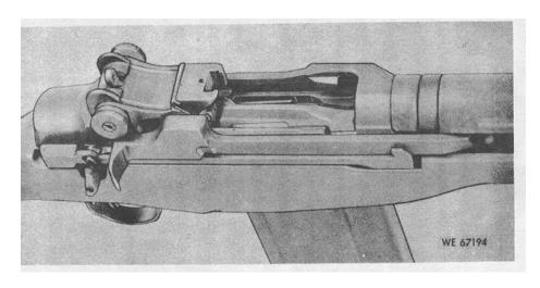
Figure 2-11. Showing bolt in open position.
