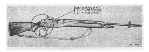
Figure 1-7. 7.62-MM Rifle M14 with winter trigger kit installed.
