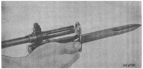
Figure 2-17. Installation/removal of bayonet-knife.
