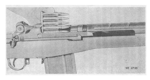
Figure 2-4. Loading magazine with clip.
