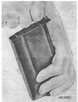
Figure 3-3. Disassembly/assembly of magazine.
