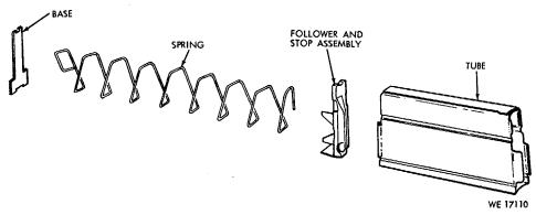
Figure B-1. Magazine-exploded view.
