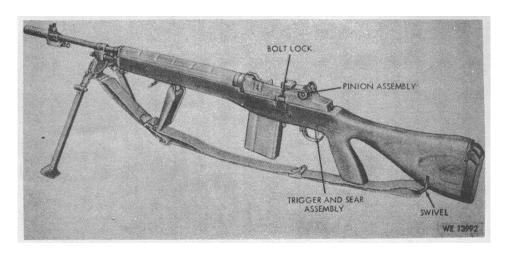
Figure 1-8. 7.62-MM Rifle M14A1-left rear view.
