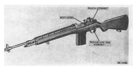
Figure 1-1. 7.62-MM Rifle M14-left front view.
