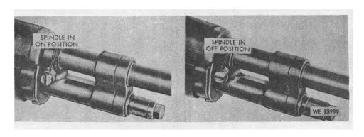
Figure 2-13. ON-OFF position of spindle valve.
