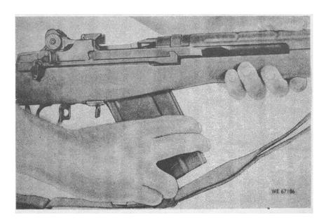
Figure 2-5. Loading magazine into rifle.
