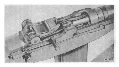
Figure 2-9. Extracting cartridge case from chamber.
