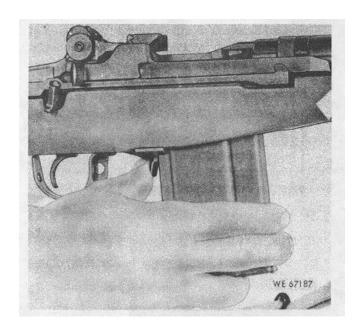
Figure 2-12. Removing magazine from rifle.
