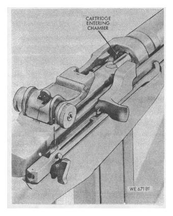
Figure 2-6. Chambering the cartridge.
