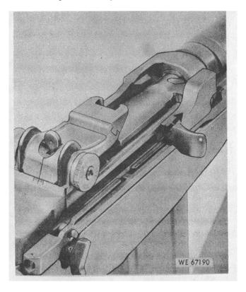
Figure 2-7. Bolt locking and unlocking.
