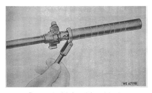
Figure 2-15. Installation/removal of grenade launcher.
