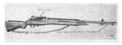
Figure 1-6. 7.62-MM Rifle M14, Blank Ammunition Firing Attachment M12 and Breech Shield M3.
