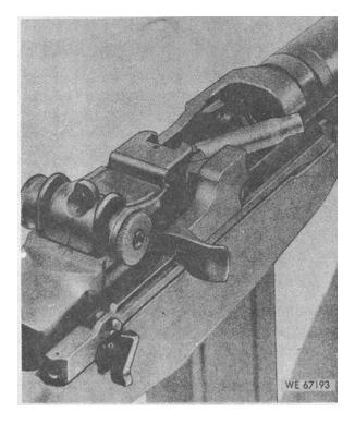
Figure 2-10. Ejecting cartridge case from chamber.
