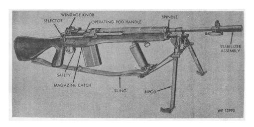
Figure 1-9. 7.62-MM Rifle M14A1-right front view.
