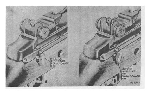
Figure 2-1. Selector set for automatic (A) and semi-automatic (B) fire.
