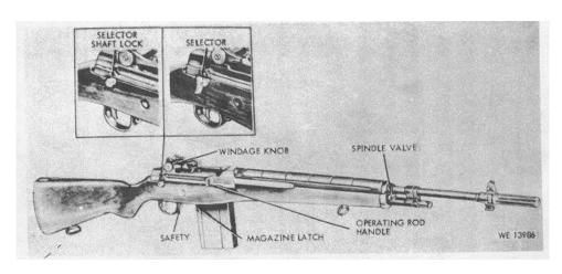
Figure 1-2. 7.62-MM Rifle M14-right front view.
