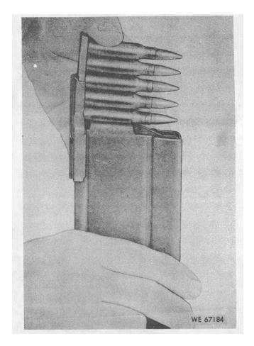
Figure 2-3. Loading magazine with filler and clip.
