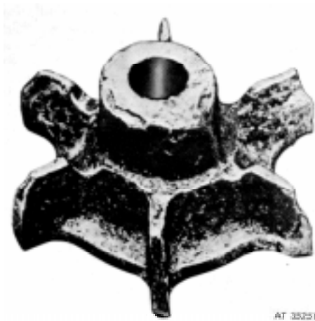
Figure 2-7. Corrosion of water pump impeller.
