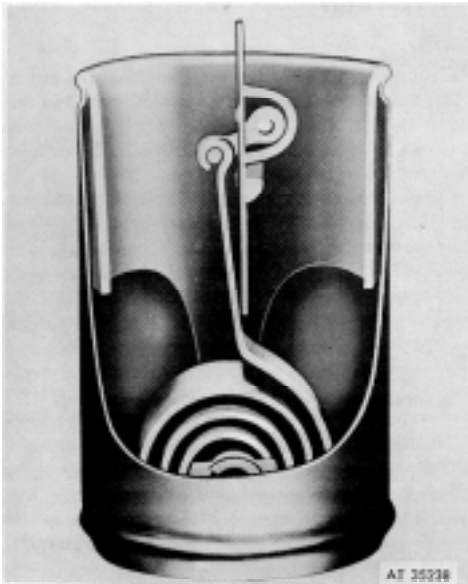
Figure 1-8. Coil spring-type thermostat - cutaway view.
