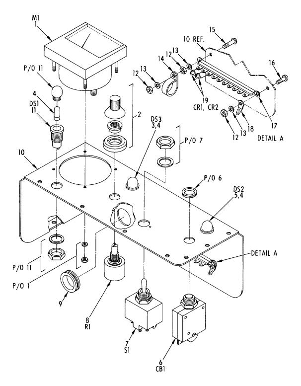
FIGURE C-2. CONTROL PANEL ASSEMBLY.
