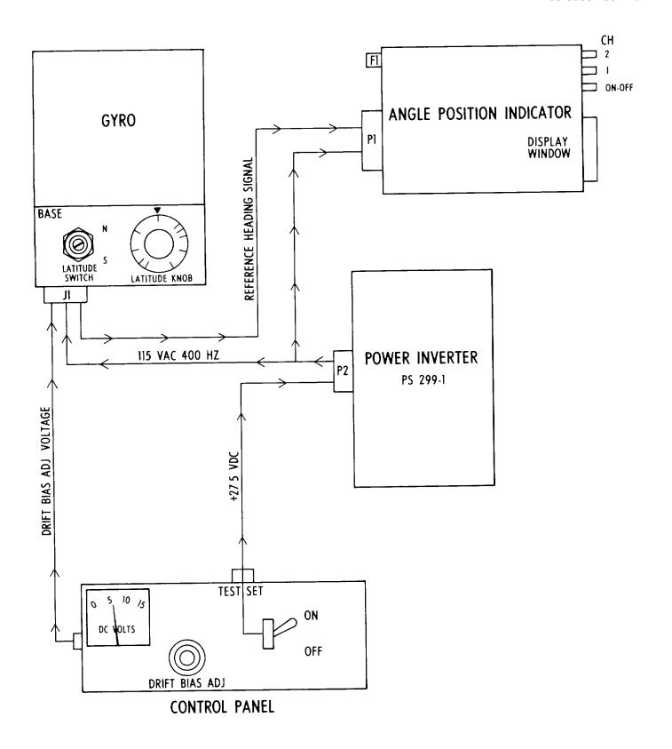
FIGURE 1-6. RMHS REFERENCE GYRO SET BLOCK DIAGRAM.
