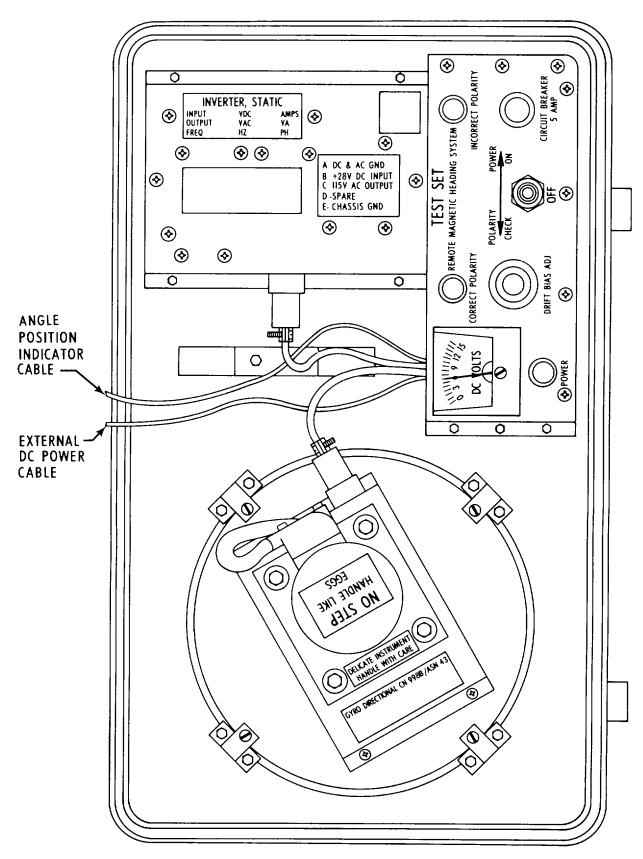
FIGURE 2-1. RMHS REFERENCE GYRO SET CONTROLS AND INDICATORS.
