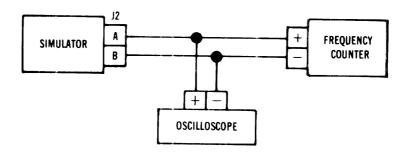
FIGURE 4-3. Frequency Output Check Setup
