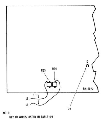
FIGURE 4-15. Signal Generator Board (PCB 2) Wiring, Component Side
