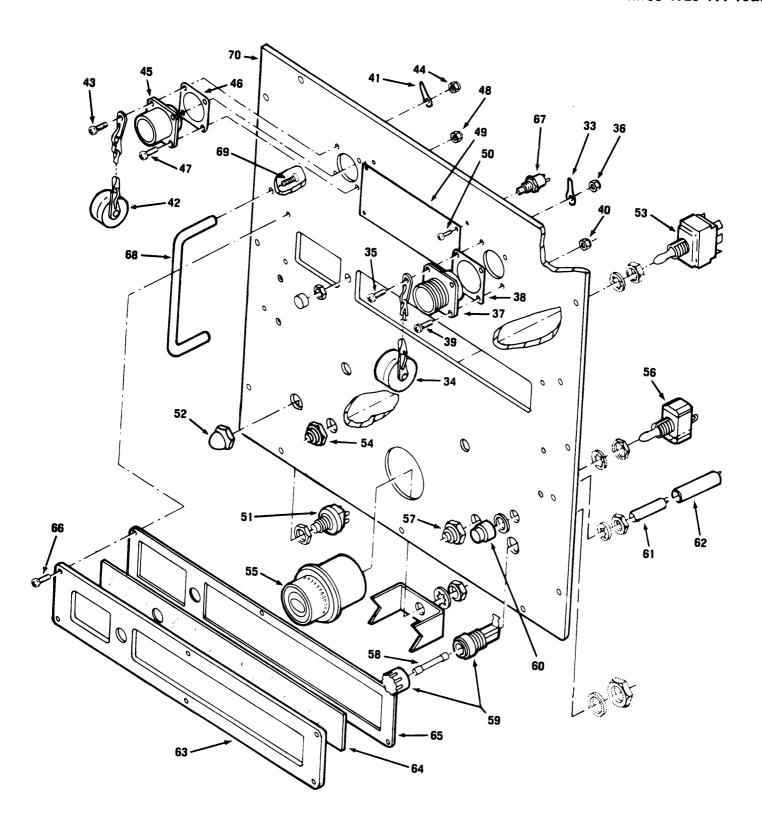
FIGURE C3.Deck Assembly Exploded View (Sheet 2 of 2)
