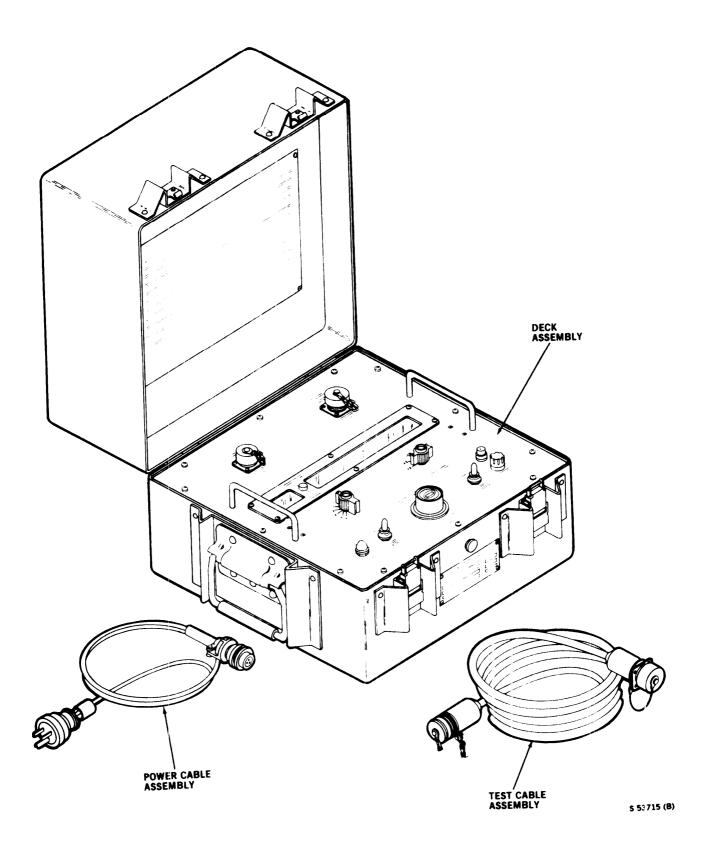
Figure 1-1. Temperature and Speed Simulator
