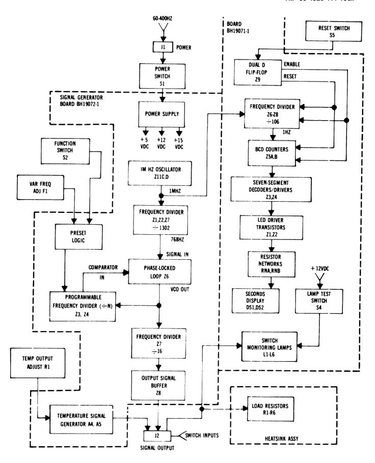
FIGURE 3-2. Block Diagram of Speed-Temperature Signal Unit
