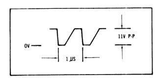
FIGURE 4-13. Oscillator Waveform
