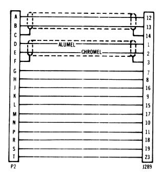
FIGURE 4-10. Test Cable Schematic
