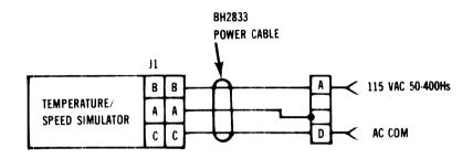
FIGURE 4-11. Simulator Power Connection
