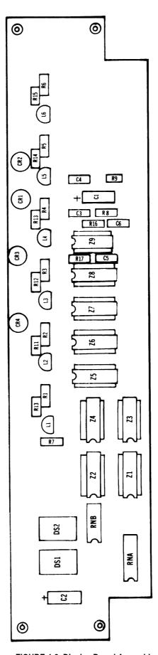
FIGURE 4-2. Display Board Assembly
