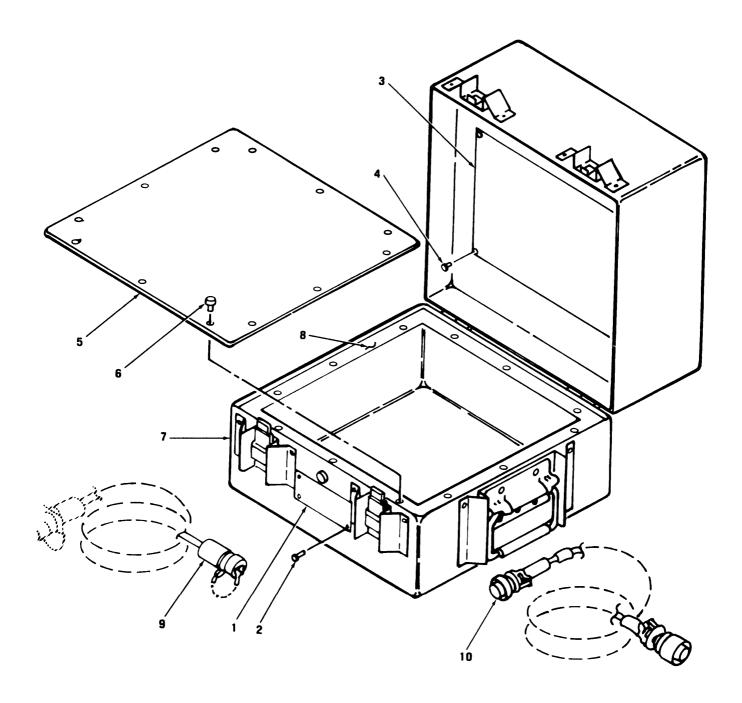
FIGURE C-1. H296A-1 Temperature/Speed Simulator Exploded View
