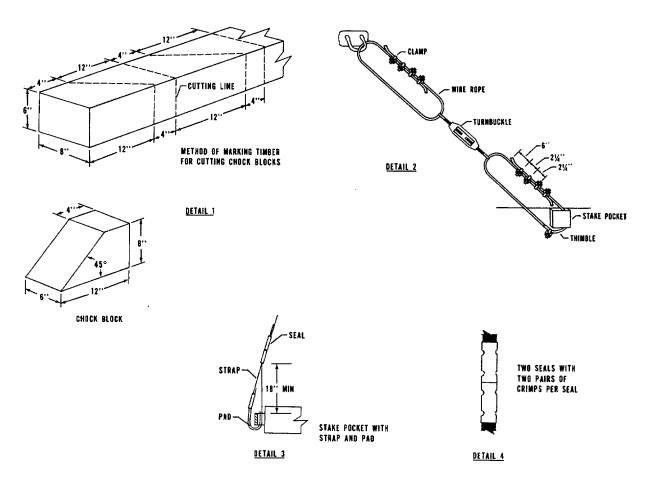
Figure 7-10. Blocking and tiedown details for figures 7-1 through 7-9.
