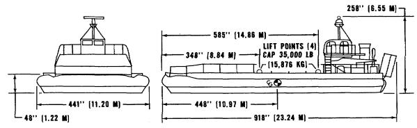
Figure 2-4. LACV-30, side and front elevation.
