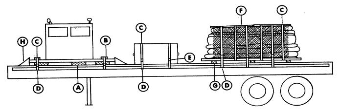
Figure 5-7. Blocking and tiedown of LACV-30 control cabin, bow fenders, and load spreader pallets with peripheral trunk and cargo net on flatbed trailer.
