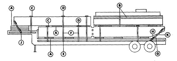
Figure 5-1. Blocking and tiedown of LACV-30 aft center buoyancy box (air management system) with center midcraft buoyancy box, vehicle ramps, and port and starboard aft side decks on low-bed semitrailer.
