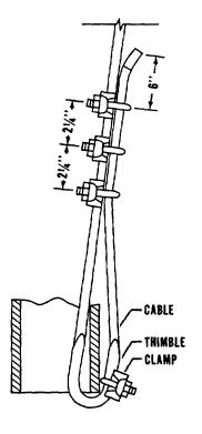
Figure 7-11. Blocking and tiedown details(railcar stake pocket and wire rope loop)
