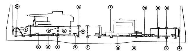
Figure 7-1. Blocking and Tiedown of LACV-30 port power module with port midcraft buoyancy box, control cabin, and port and starboard midcraft side decks on PTTX bulkhead railcar.
