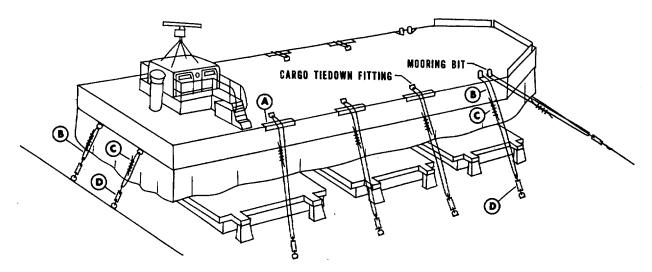
Figure 6-2. Tiedown details, LACV-30 on deck of break-bulk ship.
