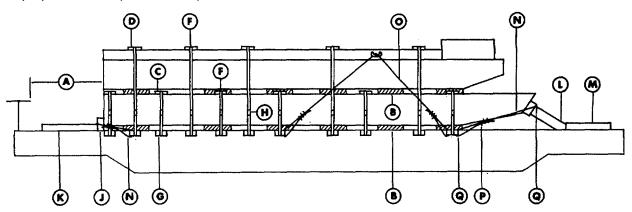
Figure 7-7. Blocking and tiedown of LACV-30starboardforward buoyancy box and port and starboard forward side decks on CONUS general-purpose flatcar (side view).
