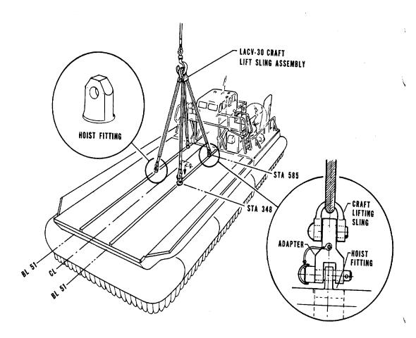
Figure 6-1. Lifting Diagram, LACV-30.
