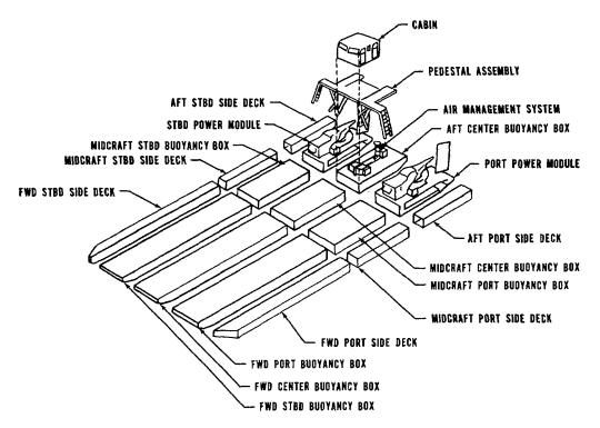
Figure 2-3. L4CV-30, modular construction.
