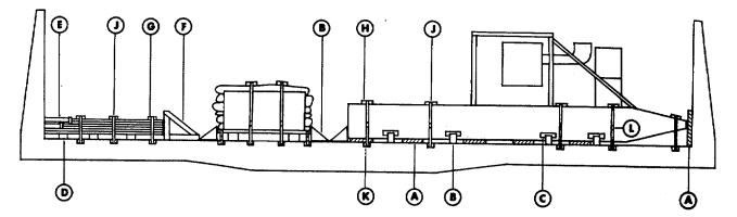
Figure 7-3. Blocking and tiedown of LACV-30 aft center buoyancy box (air. rnanagement system without stack) with center midcraft buoyancy box, four load-spreader pallets, two tracks, and palletized flexible trunk system on PTTX bulkhead railcar
