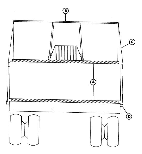
Figure 5-6. Blocking and tiedown of LACY-30 starboard forward buoyancy box, port and starboard forward side decks, and landing pads on flatbed semitrailer (end view).
