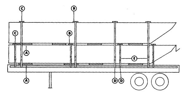
Figure 5-5. Blocking and tiedown of LACV-30 starboard forward buoyancy box, port and starboard forward side decks, and landing pads on flatbed semi-trailer (side view).
