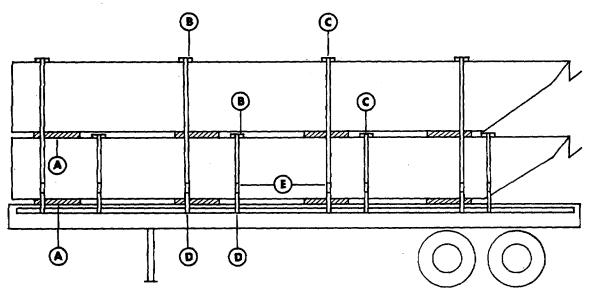
Figure 5-4. Blocking and tiedown of LACV-30 center and port forward buoyancy boxes on flatbed semitrailer.
