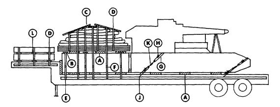
Figure 5-3. Blocking and tiedown of LACV-30 starboard power module with starboard midcraft buoyancy box, four load-spreader pallets with stability trunks, rear trunks and two fenders, and two crated propellers on low-bed semitrailer.
