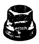
Description: Model 1600 Wager Tank Air Escapes consist of a body (of any material) equipped with a 30 x 30 mesh monel flame screen and a VY x Y4 mesh monel protecting screen, separated by a spacer ring. These parts are held in place on the body by means of a monel cap and #316 stainless steel screws.
