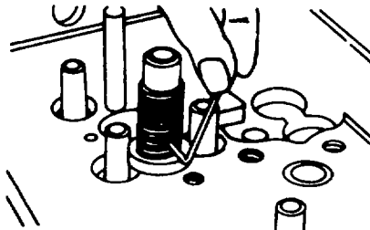
Figure 4-7. Bridge Guide Removal Tool, Installation.
