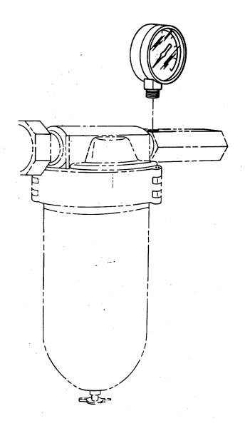
Figure 2-117. Starting Air Pressure Gage.
