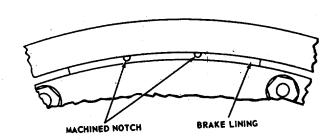
Figure 2-63. Brake Lining.
