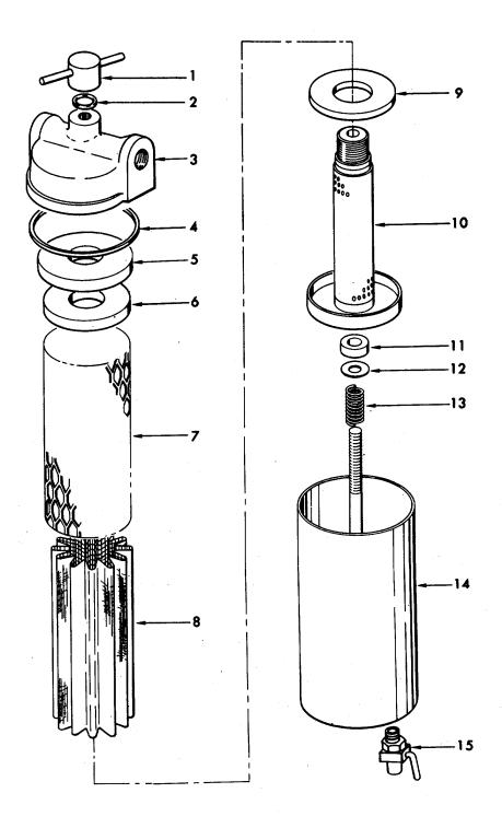
Figure 2-61. Fluid Pressure Filter, Exploded View.
