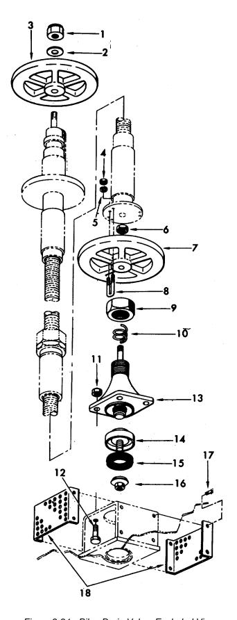
Figure 2-21. Bilge Drain Valve, Exploded View.
