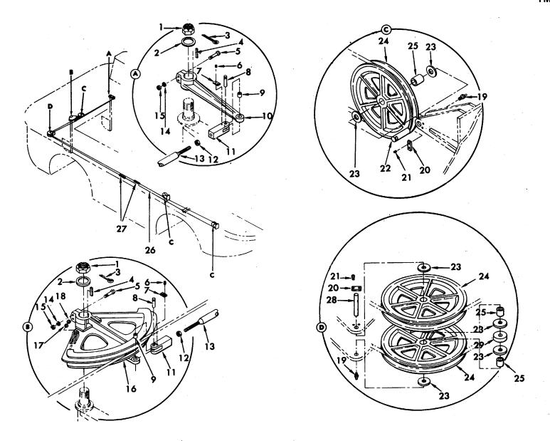
Figure 2-109. Marine Steering, Exploded View.
