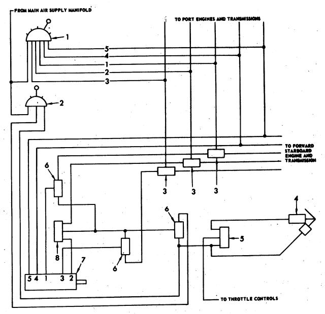
Figure 2-92. Transmission Shifting Control and Engine Cutout Systems Diagram.
