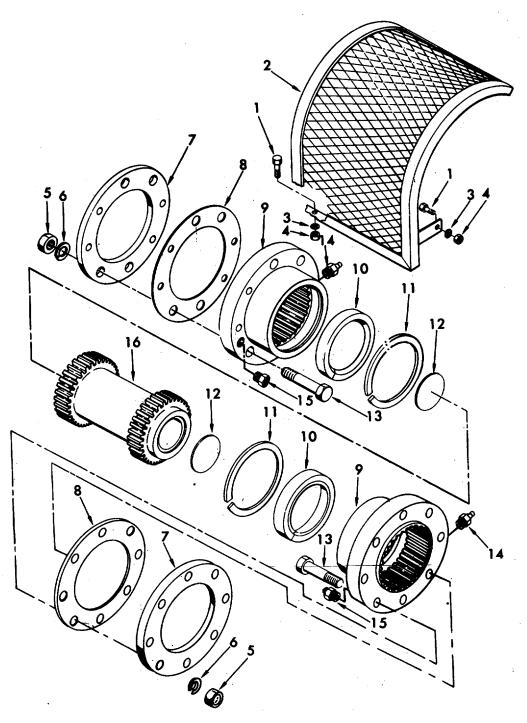
Figure 2-64. Torque Converter - TRANSMISSION FLEXIBLE COUPLING, Exploded View.
