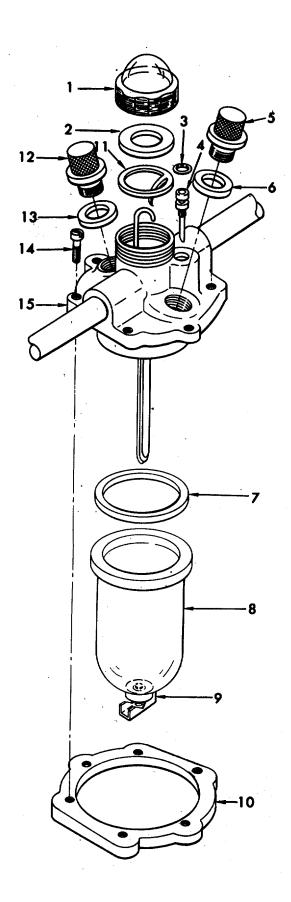
Figure 2-89. Air Starting Lubricator, Disassembly and Reassemby.
