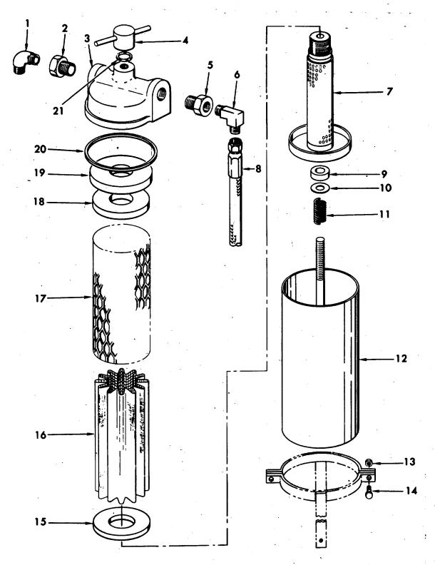
Figure 2-76. Oil Sediment Strainer, Exploded View.
