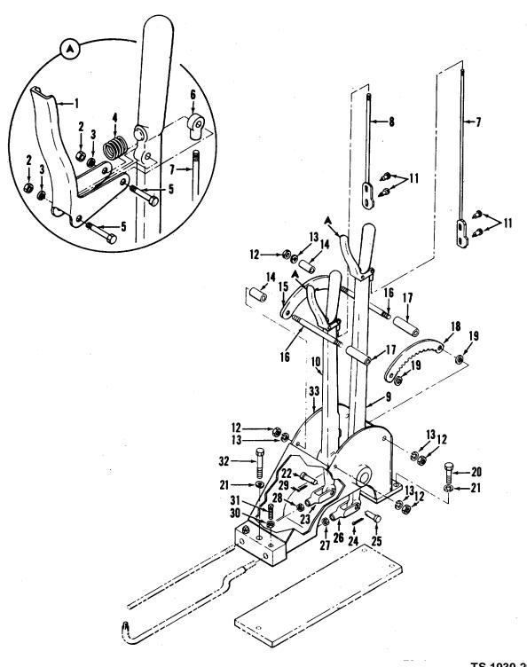
Figure 2-119. Control Stand, Disassembly and Reassembly.
