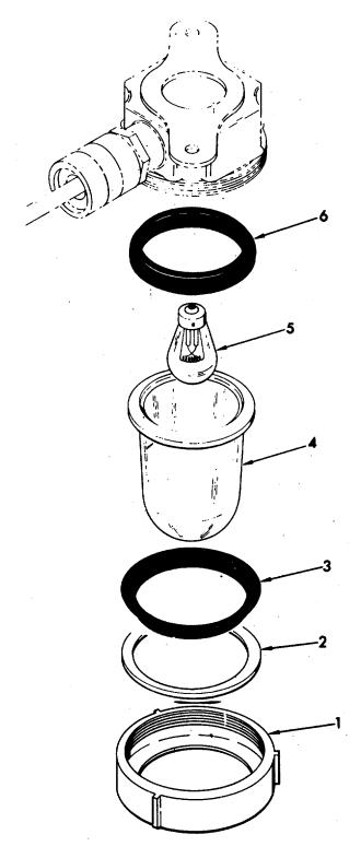
Figure 2-8. Compartment light lamp Replacement.
