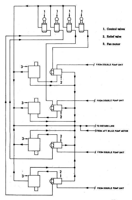
Figure 2-35. Fan Motor Hydraulic System Diagram.
