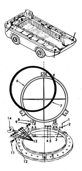
Cotter pin 8. Cotter pin Nut Nut 9. 10. Washer, flat Washer, flat Bolt 11. Bolt Washer, flat Washer, flat Dog bolt and wingnut 5. Washer Scuttle Gasket 13. 6. 7. 14.
