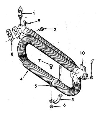
1. Safety valve 6. Nut 2. Bolt 7. Bolt 3. Nut Gasket 8. 4. Intercooler 9. Flange 5. Clamp 10. Flange
