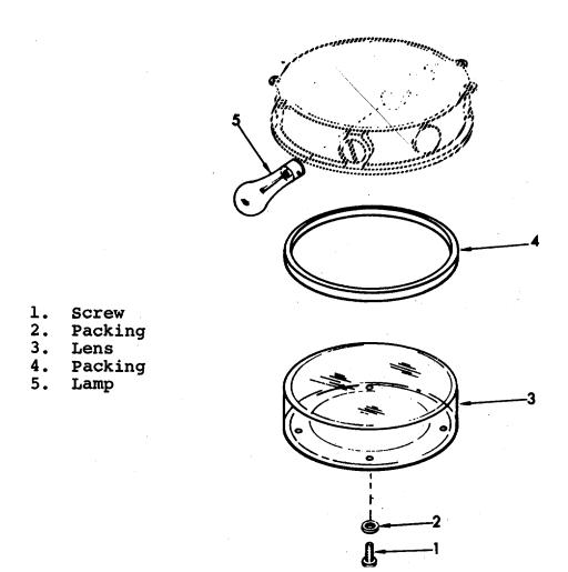
Figure 2-9. Machinery Compartment Light Lamp Replacement.
