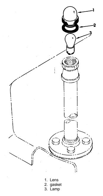
Figure 2-5. Range Anchor Light Lamp Replacement.
