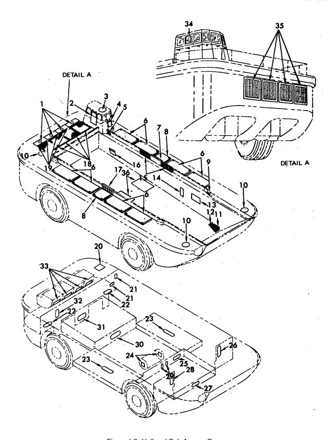
Figure 1-2. Hull and Cab Access Covers.
