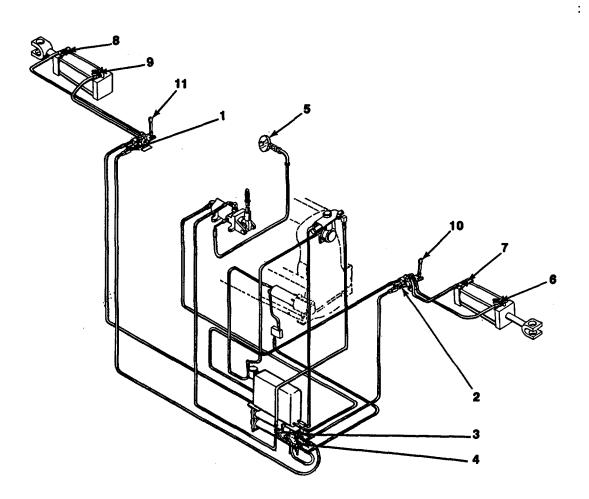
Figure 2-128. Wheel Alignment System.
