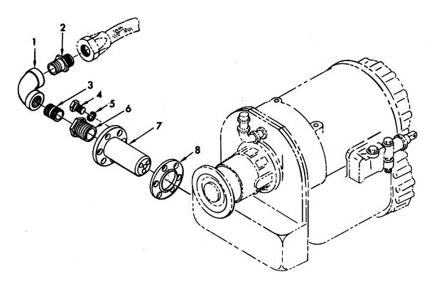
1. Elbow Lockwasher 5. 2. Adapter 6. Bushing, pipe 3. Nipple 7. Oil strainer Capscrew 8. Gasket 4.
