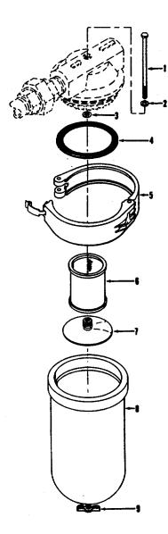
Figure 2-88. Air Starting Filter, Disassembly and Reassembly.
