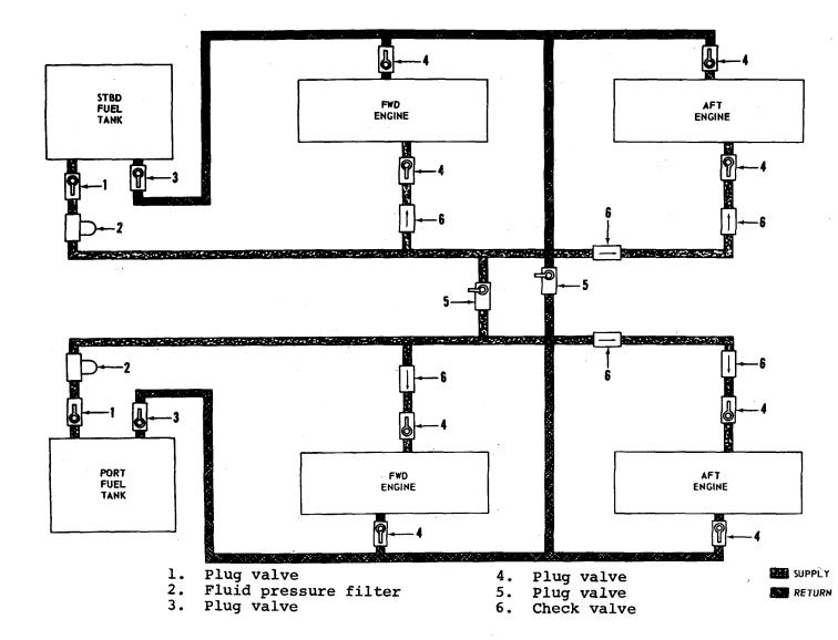
Figure 2-60. Fuel System Schematic. **2-195**
