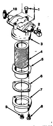
Figure 2-86. Main Air Supply Filter, Disassembly and Rassembly.
