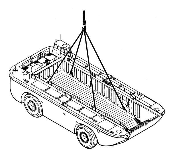
Figure 2-1. Hoisting the LARC.
