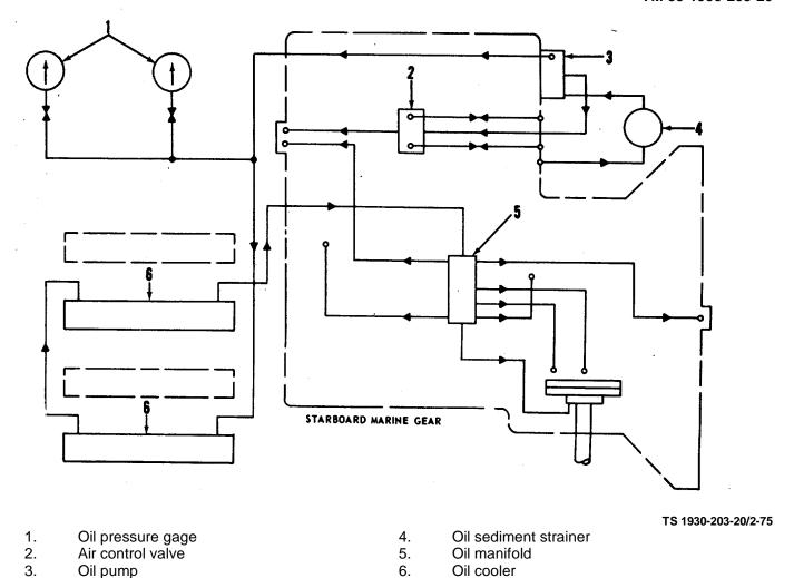
Figure 2-75. Marine Gear Oil Lines Flow Diagram.
