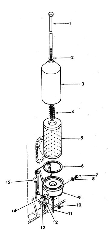
Figure 2-49. Bypass Oil Filter, Removal and Installation.
