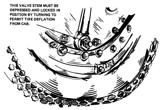
Figure 2-100. Tire Inflation Check Valve.
