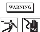
Replace or repair components only after the affected circuit has been secured, locked out, and tagged out. Performing replacement with the circuit energized may resut in injury.
