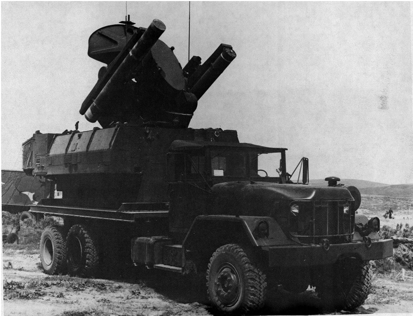
Figure 2-4. ROLAND missile system fire unit in its operational configuration.
