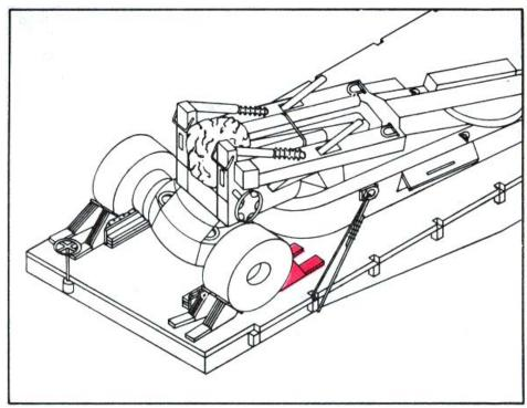
Place the other four chock blocks, two against the front of each tire, and nail to the flatcar deck. Drive two 60d nails through the heel (back) of each chock block, and toenail through the sides of the blocks with two 40d nails on each side.
