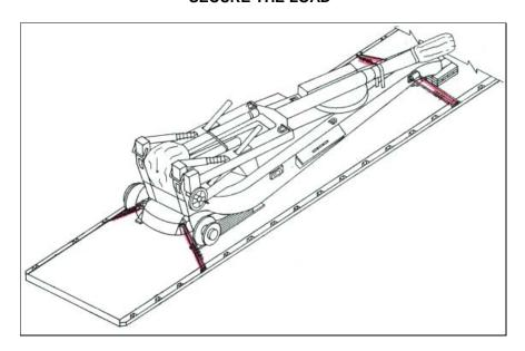
Tie the howitzer to the trailer with 1/2-inch wire rope. A total of four tiedowns are required. Attach one to each of the two rear tiedown points and one to each of the two weapon support brackets.
