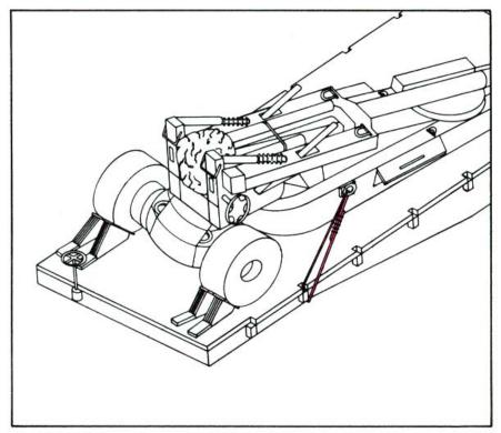
Loop the first two wire rope tiedowns from the tiedown provisions on the sides of the howitzer carriage to a stake pocket near the howitzer tires. Select a stake pocket that will result in a tiedown angle as near to 45 degrees as possible. Tighten these two tiedowns, making sure that the howitzer tires are pulled tight against the rear chock blocks.
