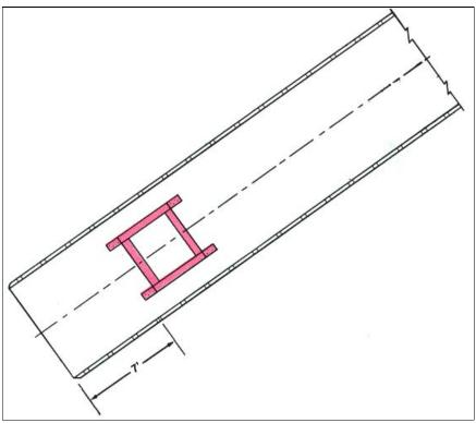
Position the base support assembly seven feet from the rear end of the trailer deck, centered on the center line of the deck, and nail to the deck with four 12d nails through each end of each bottom piece of lumber.
