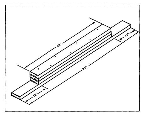
Nail three of the 48-inch-long pieces to each of the two 72-inch-long pieces, using seven 10d nails through each piece.
