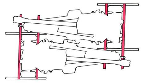
Cut four pieces of 4- by 4- by approximately 110-inch-long lumber, and lay a piece on the top of side blocking and against front and rear of tires. Nail at each place where the top piece crosses the bottom piece with two 50d nails.
