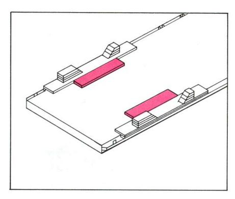
Cut two pieces of 2 by 6 by 48-inch lumber and six pieces of 2 by 4 by 48-inch lumber for the side blocks. Build two side blocks for blocking against the inside of the wheels, using the following steps. Nail one of the 2 by 6 inch pieces to the edge of one of the 2 by 4-inch pieces with five 12d nails.
