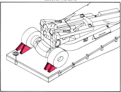
Cut eight pieces of 2- by 6- by 12-inch lumber to use as backup pieces for the chock blocks. When the howitzer is in place on the flatcar, place two chock blocks tightly against the rear of each tire, with the face plates against the tire. Nail the chock block to the deck with two 60d nails through the heel (back) of each block, and toenail through the sides of the blocks with two 40d nails on each side.
