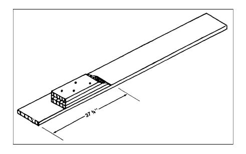
Place the bottom piece on the 2 by 12-inch by 8-foot base so that the 45 degree angle is toward the center of the base and 37-3/8 inches from the end. Nail to the base with four 10d nails. Nail each additional piece to the piece below with four 20d nails.
