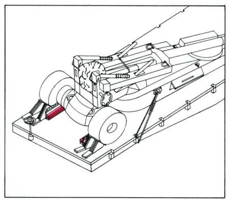
The waterproof paper or burlap protects the tire and should extend from under the side block to about 2 inches above it. Nail two more 2- by 4-inch pieces on top of the bottom piece with five 30d nails through each piece.
