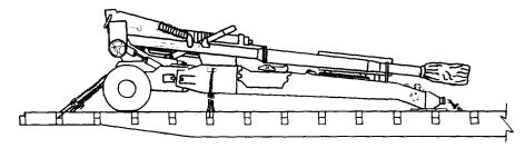
Attach the chain tiedowns from each side and rear howitzer tiedown point to the outside tiedown channels on the railcar. Attach two chain tiedowns from the howitzer lunette to the inside tiedown channels. Tighten the chains with turnbuckles.
