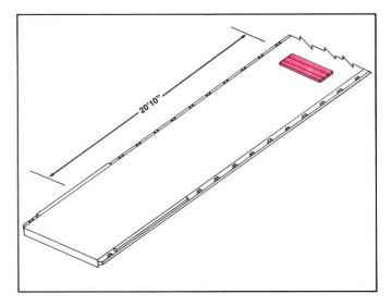
Make a support platform for the trails using three pieces of 2-by 6-by 48-inch lumber. Place the support platform in the center of the trailer deck with the front edge approximately 20 feet 10 inches from the center line on which howitzer wheels will rest. Nail the platform to the trailer deck, using five 12d nails though each piece.
