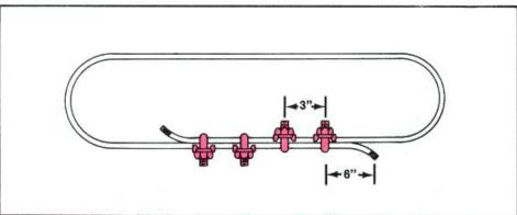
Secure the ends of the wire rope at the overlap area with four 112-inch U-bolt clips, spaced 3 inches apart, none closer than 6 inches from the ends of the wire rope.
