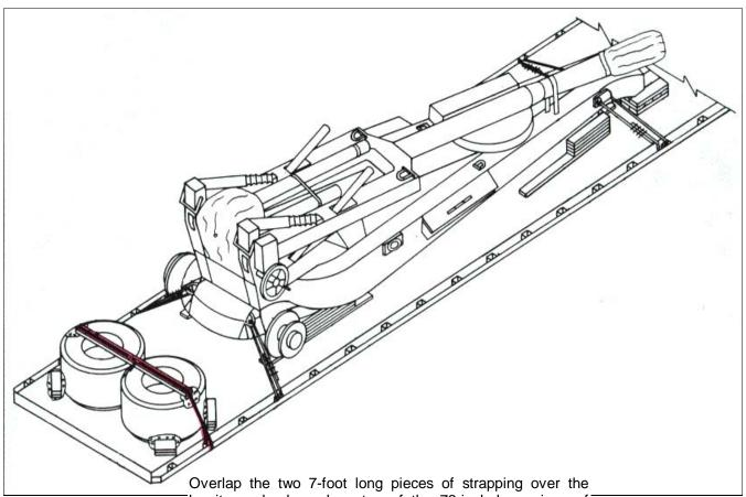
Overlap the two 7-foot long pieces of strapping over the howitzer wheels and on top of the 72-inch long piece of lumber, tighten and join with a seal. This seal requires two pairs of crimps.
