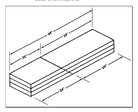
Build two wheel chock-block assemblies, starting with two pieces of 2 by 12-inch by 8 foot lumber as a base. Cut 6 pieces of 2 by 8 by 44-inch lumber. Make two stacks of three pieces each and cut so that four chock blocks with about 45 degree angles can be made.
