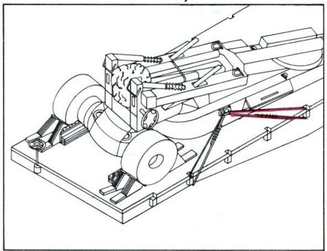
Install the second pair of steel wire rope tiedowns. Form loops from the tie-down provisions on each side of the howitzer carriage to the flatcar stake pockets. Select a stake pocket that will result in a tiedown angle as near to 45 degrees as possible. This will be about the third stake pocket forward of where the first two tiedowns are located. Install thimbles and U-bolt clips, tighten the tiedown and torque the U-bolt clip nuts.
