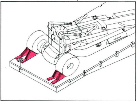
Next, position a 2-by 6-by 12inch backup piece tightly against each chock block and nail each one to the flatcar deck with three 30d nails.
