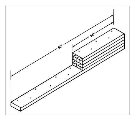
Build two blocking assemblies out of two pieces of 2 by 6 60-inch lumber and eight pieces of 2 by 6 by 24-inch lumber. Nail four 24 inch-long pieces to each of the 60-inch-long pieces with five 10d nails through each 24 inch piece.
