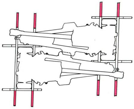
Cut 4- by 4- inch by length-to fit lumber, and use as bracing against the ship's structure and other cargo. Nail in place with 20d nails.
