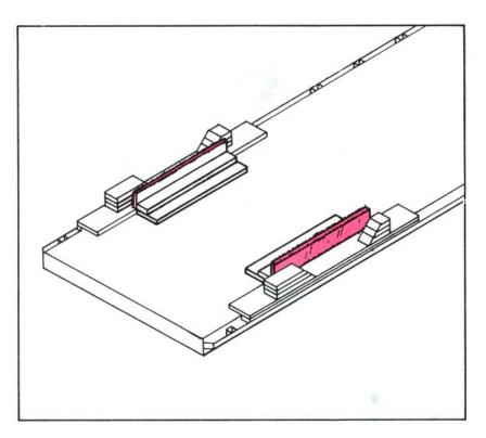
Place a piece of 10 by 48-inch waterproof paper or burlap between the 2 by 6-inch lumber and the howitzer tire and nail the 2 by 4-inch piece to the riser with five 12d nails.
