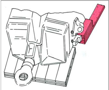
Position a blocking assembly against the plunger assembly slot on each side of the howitzer trails and nail each assembly to the trailer deck through the 60 inch long piece with seven 20d nails.
