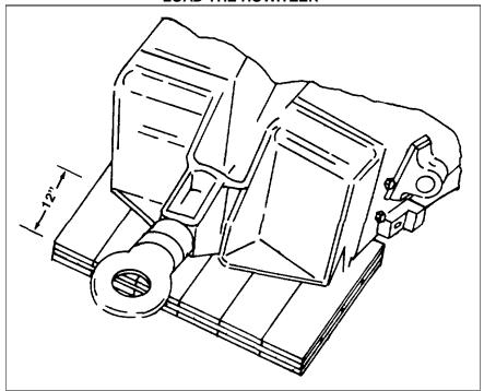
Lift the M198 howitzer onto the trailer using a crane of at least 8-ton capacity. Position the howitzer by centering it across the width of the trailer and in the base support assembly and the riser assembly. Position the howitzer fore and aft by placing the end of the trails 12 inches from edge of the riser assembly.
