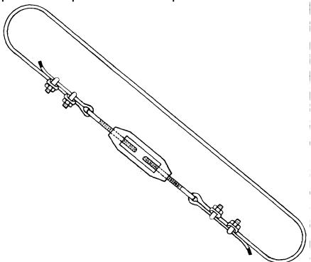
Complete loop. Form complete loop by securing the ends of the 5/8-inch wire rope to the eyes of the 3/4-inch tumbuckle. Allow at least 12 inches overlap on each end of the wire rope for two 518-inch U-bolt clips. Outside U-bolt clip should be placed at least 6 inches from overlapped ends of wire rope.
