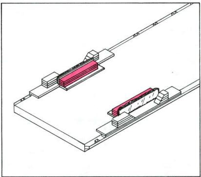
Nail two more 2 by 4 by 48 inch pieces of lumber to the bottom piece with five 12d nails through each piece. Fabricate and install another side block inside the other wheel.
