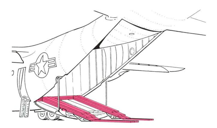
Place two rows of lumber from the ground to the top of the aircraft ramp, spaced to match the howitzer wheels. Each row should be approximately 24 inches wide, 5.25 to 5.5 inches thick, and 17 feet long. The required thickness can be obtained with three pieces of 2-inch-thick undressed lumber, one on top of the other. Shoring at the foot (ground level) of the ramp should be stair-stepped for easy transition to the 5.25 inch level.
