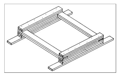
To complete the base support assembly, nail two more 2 by 6 by 48-inch pieces of lumber on top of each side with seven 10d nails.
