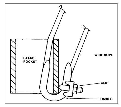
Place standard 1/2-inch opentype thimbles at each place where the wire rope contacts the trailer-stake pocket and where the wire rope contacts the rear tiedown points on the howitzer. Secure the thimbles to the wire rope with a 1/2-inch U-bolt clip.
