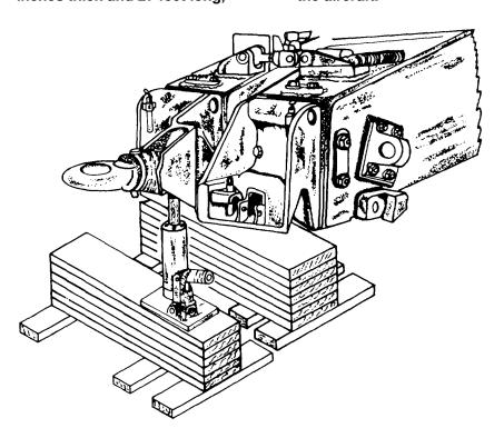
The trails of the howitzer also must be supported on shoring, and this will require 40 pieces of 2x 12-inch by4foot lumber.
