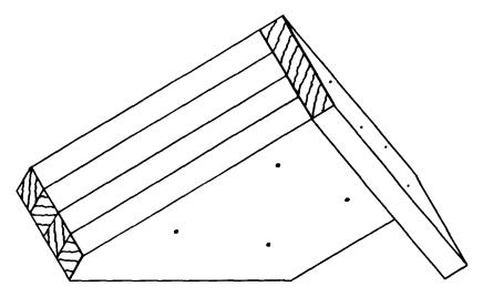
Nail the four pieces together with four 10d nails through each piece. Next, nail a 2-by 6-by 18-inch face piece to the four pieces with four 10d nails like this:
