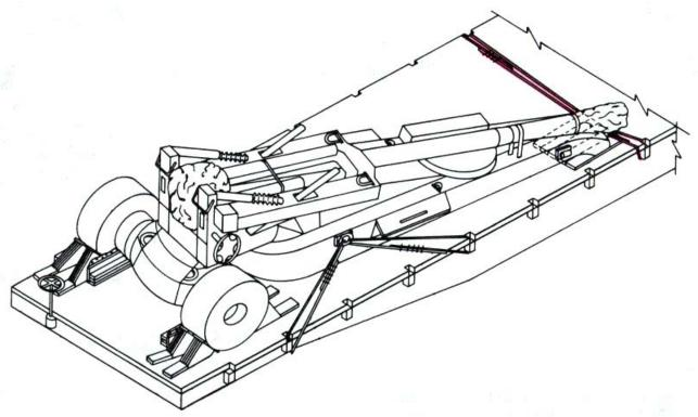
Loop the third pair of steel wire rope tiedowns from the howitzer lunette to the next stake pockets forward of the lunette. Install thimbles only at the point where the tiedowns contact the stake pockets. Tighten the tiedowns, install the U-bolt clips and torque the U-bolt clip nuts.
