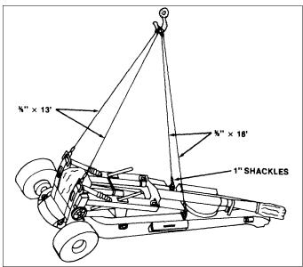
If the trailer is equipped with chains and load binders, no further preparation is required. Lift the howitzer onto the trailer with a crane of at least 8-ton capacity, centering the wheels over the filler strips, with the trails resting on the support platform. Lifting points on the howitzer in the stowed position are the four lifting eyes of 40,000 pound-capacity each. They are located on top of each trail and on each side of the top carriage.
