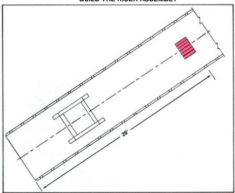
Nail the four pieces of 33-inch long lumber crossways to the lower pieces with six 20d nails through each piece. To complete the riser assembly, nail the other six 22-inch-long pieces on top with five 20d nails through each piece.
