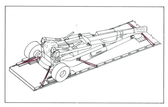
Tie the howitzer to the trailer with 112-inch wire rope. A total of six tiedowns are required. Attach one to each of the two rear tiedown points, one to each of the two side tiedown points, and two to the towing lunette.
