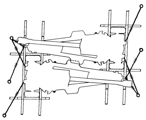
Tie down the howitzers with 5/8-inch steel wire rope and 3/4-inch tumbuckles. A total of four tiedowns to each howitzer Is required. Attach one to each of the two rear tiedown points and two to the towing lunette. The angle between the ship's deck and the tiedowns should be as close to 45 degrees as possible. Two types of tiedowns may be used.
