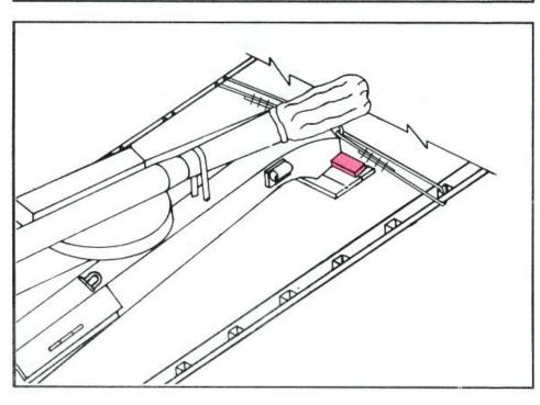
Tighten the U-bolt clip nuts enough to prevent slippage of the wire rope. After the U-bolt nuts have been tightened initially, the "U side of each clip must be struck several times with a hammer to insure proper seating. The nuts must then be re-tightened.
