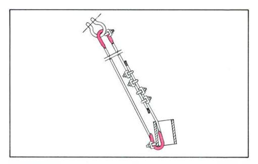
Place standard 112-inch opentype thimbles at each place where the wire rope contacts the trailer stake pocket and the howitzer tiedown points, except that no thimbles are required at the howitzer lunette. Secure the thimble to the wire rope with a 112-inch U-bolt clip.
