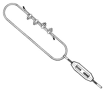
Wire loop with suspended tumbuckle. One end of the tumbuckle is attached to the ship's padeye or other deck fitting with a shackle. Run the wire rope through the other eye of the tumbuckle. Overlap and secure the ends of the wire rope at the overlap with four U-bolt clips, placed 3-3/4 inches apart, and a minimum of 6 inches from the ends of the wire rope. The wire rope ends should overlap at least 24 inches.
