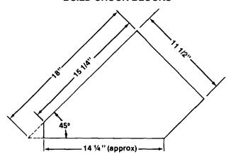
Build eight chock blocks for the howitzer wheels. Each block is made from four pieces of 2-by 12-inch lumber cut like this:
