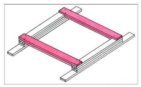
Nail two pieces of 2 by 6 by 37-inchlong lumber between the ends of the tie pieces with five 10d nails through each.
