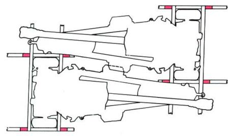
Cut 8 backup blocks of 4- by 4- by 18-inch lumber. Place one block against the top piece where it crosses the bottom piece near each tire. Nail the backup block to the bottom piece with two 50d nails.
