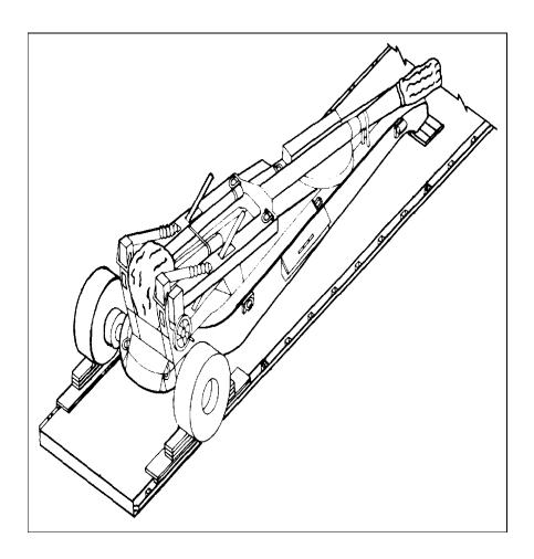
Center the howitzer on the trailer with the wheels in the wheel-block assemblies and the trails resting on the support platform. Set and wire tie the howitzer handbrakes.
