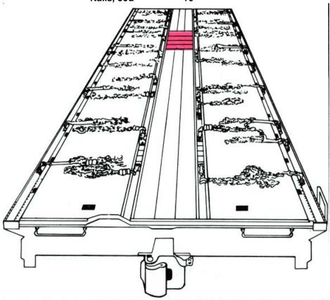
Before loading the howitzer, make a support platform for the trails using four pieces of 2- by 8- by 36-inch lumber. Decide where the trails will rest and center the platform on the railcar at that point. Nail the platform to the railcar deck crossways to the center line with four 30d nails through each piece.
