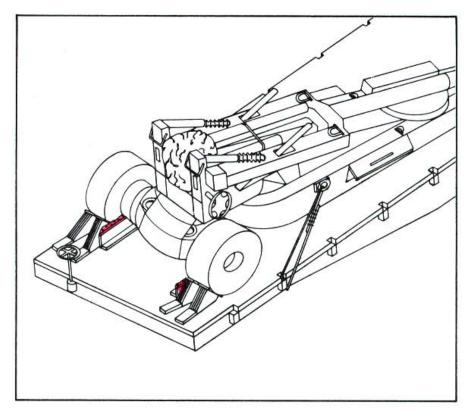
Place a piece of waterproof paper or burlap between the 2- by 6- inch side block and the tire, and place against the inside of the wheel. Nail to the flatcar deck through the 2- by 4-inch piece with five 30d nails.
