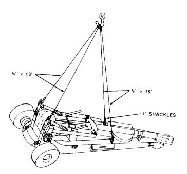
The howitzer can be placed in the tiedown position on the flatcar by a crane of at least 8-ton capacity. It can also be towed or pushed onto the flatcar if a suitable ramp is available.
