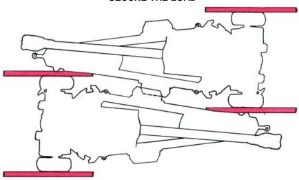
Cut four pieces of 4-by 4-by approximately 66-inch-long lumber for side blocking. Locate one piece against the outside of each howitzer wheel.
