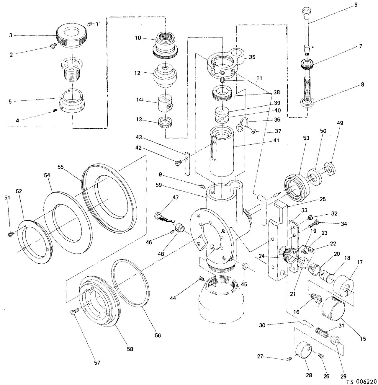
Figure 8. Telescope assembly.
