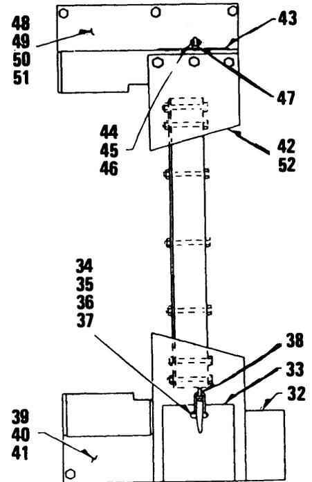
ENGINE TO MAIN GENERATOR COUPLING
