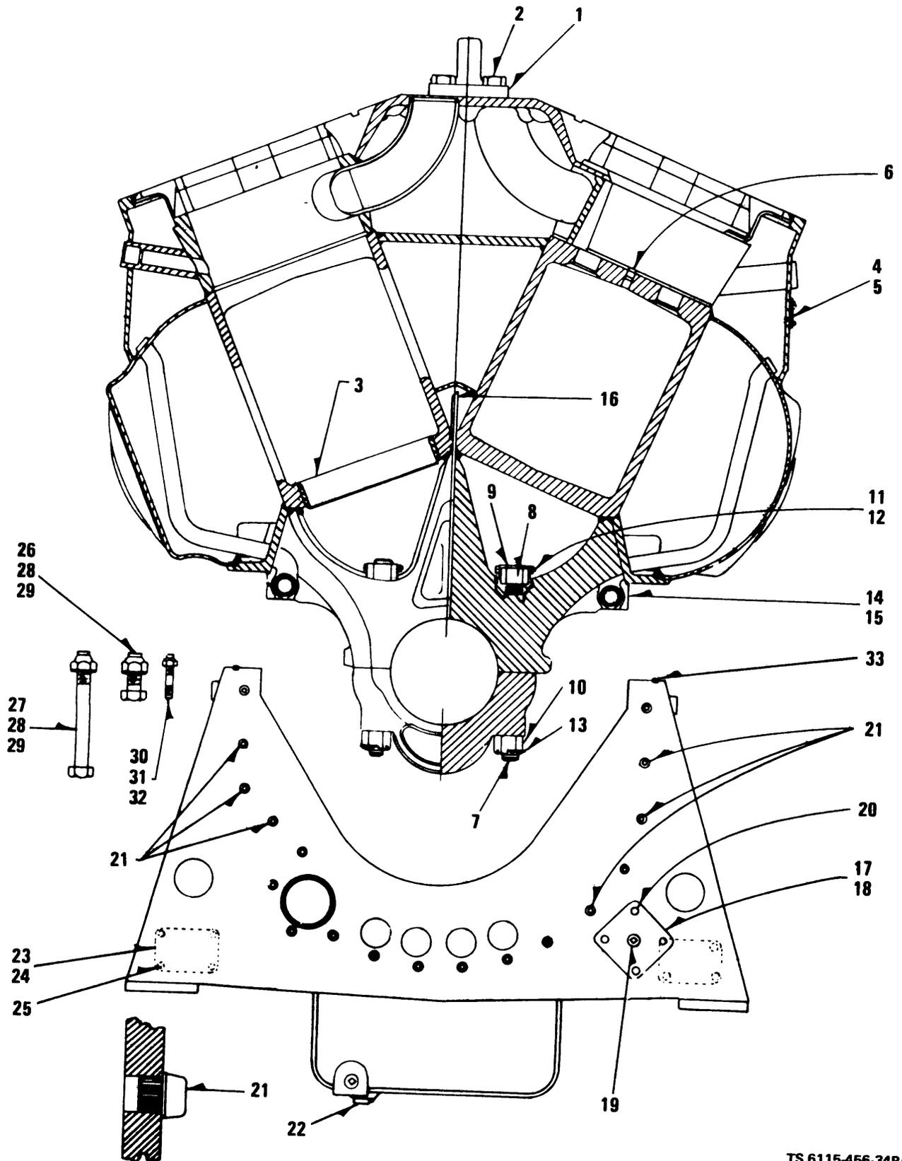
Figure 1. Crankcase and Oil Pan
