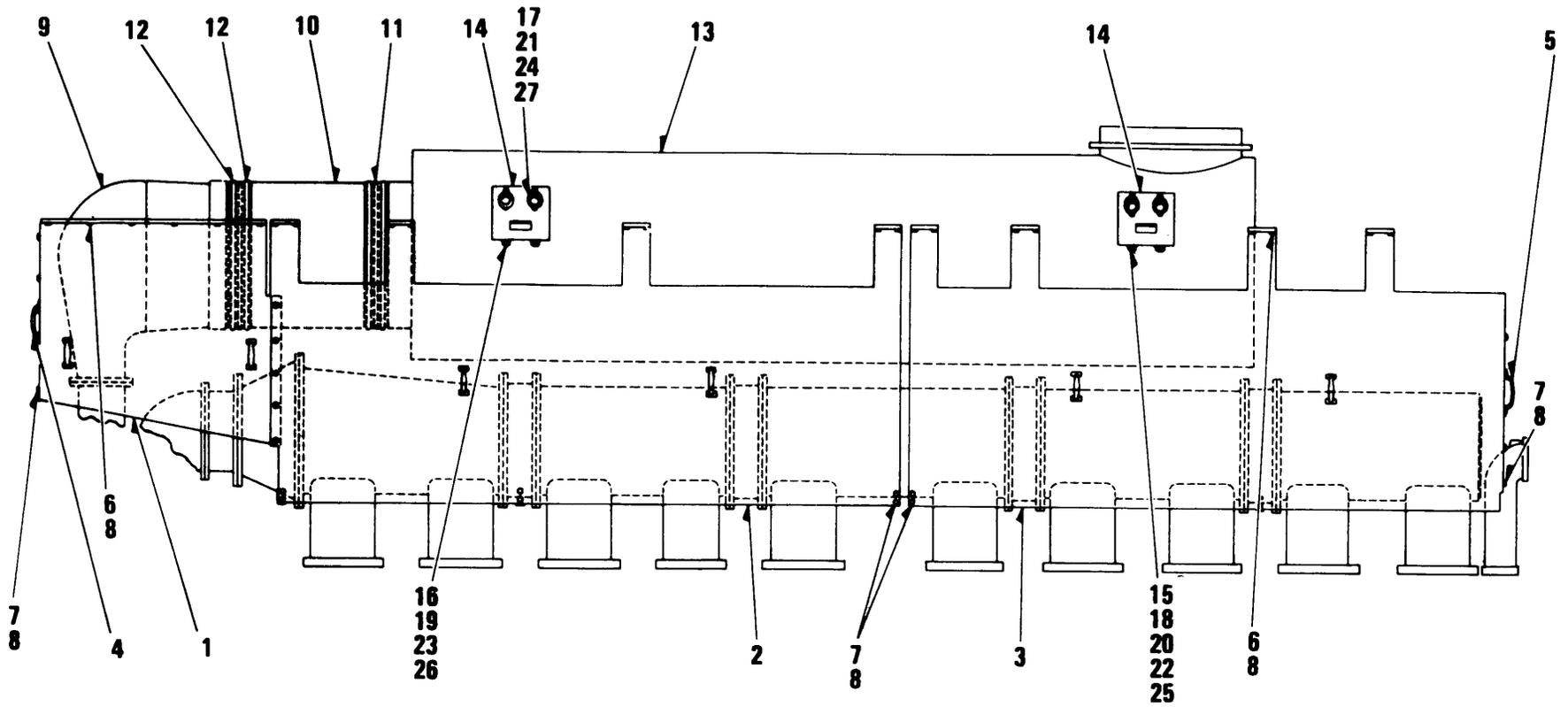
Figure 37. Exhaust Chamber Heat Shields and related Components
