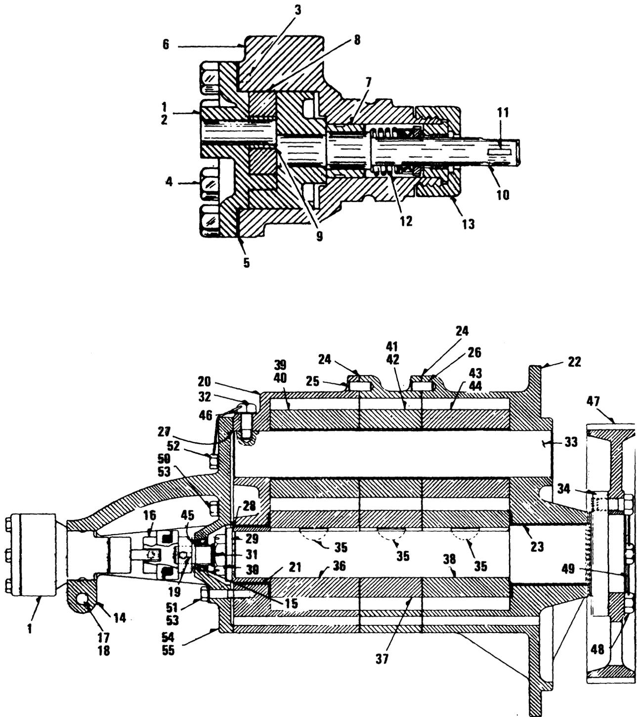
Figure 29. Lubrication Oil Scavenging Pump
