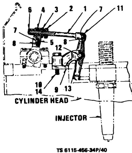
Figure 40. Injector Control Adjusting Link and Control Lever
