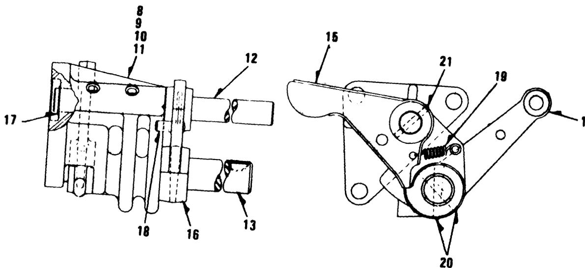
Figure 19. Camshaft Overspeed Trip Linkage
