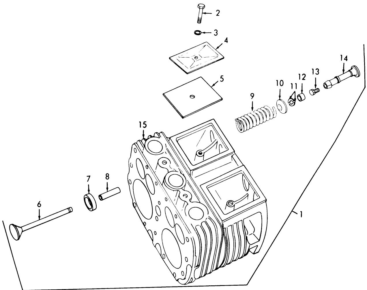
Figure 21. Cylinder Block
