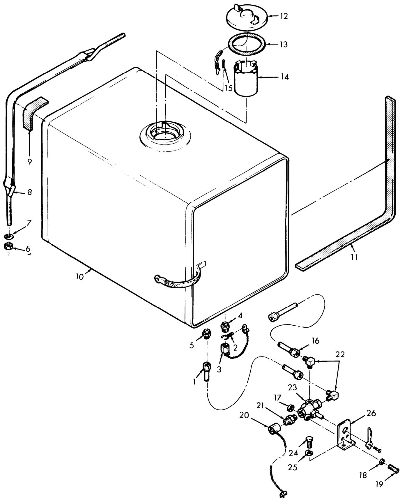
Figure 5. Fuel Tanks, Selector Valve
