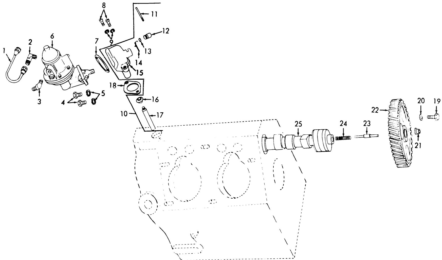
Figure 19. Camshaft and Fuel Pump
