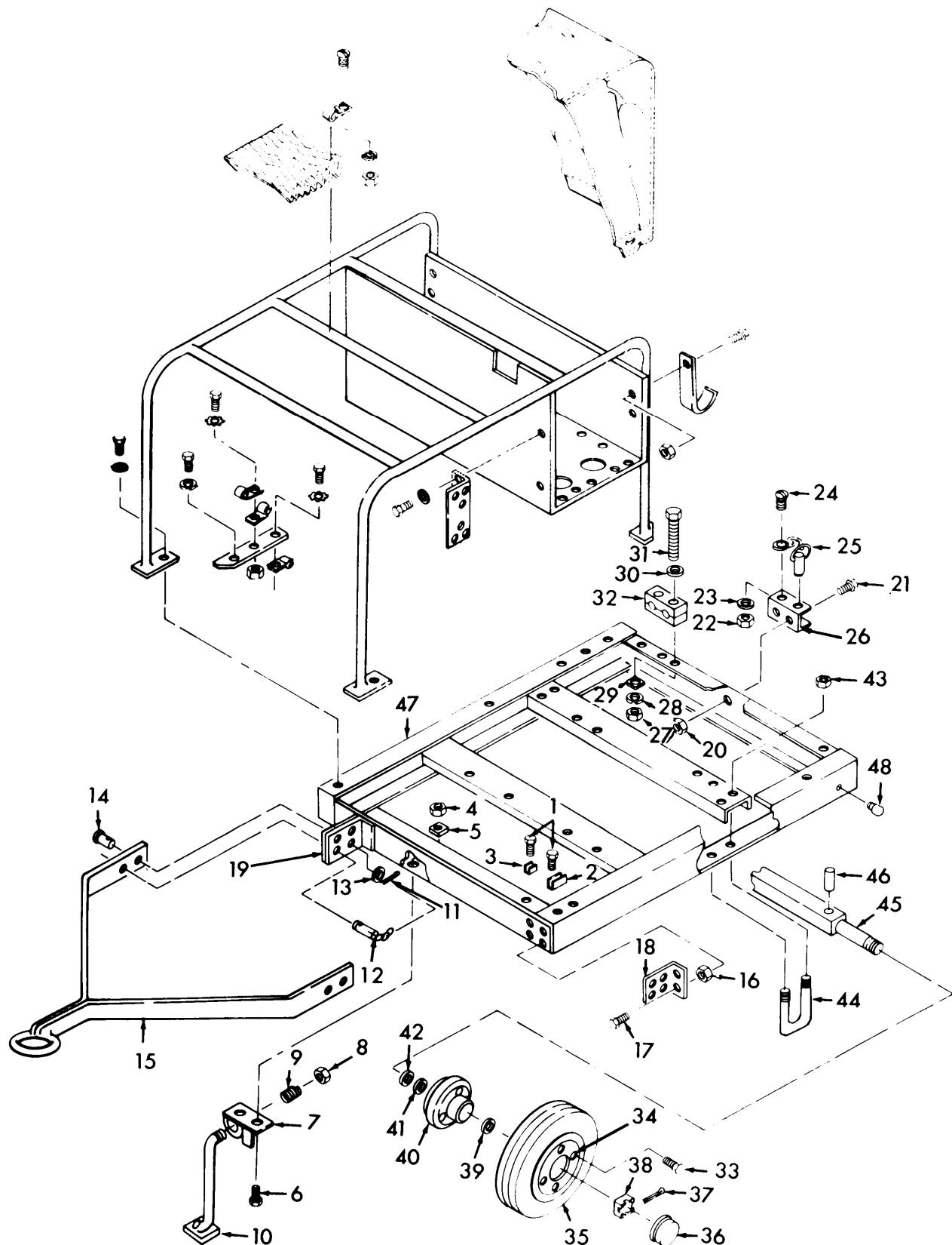
Figure 23. Base, Tow Bar, Wheel and Axle
